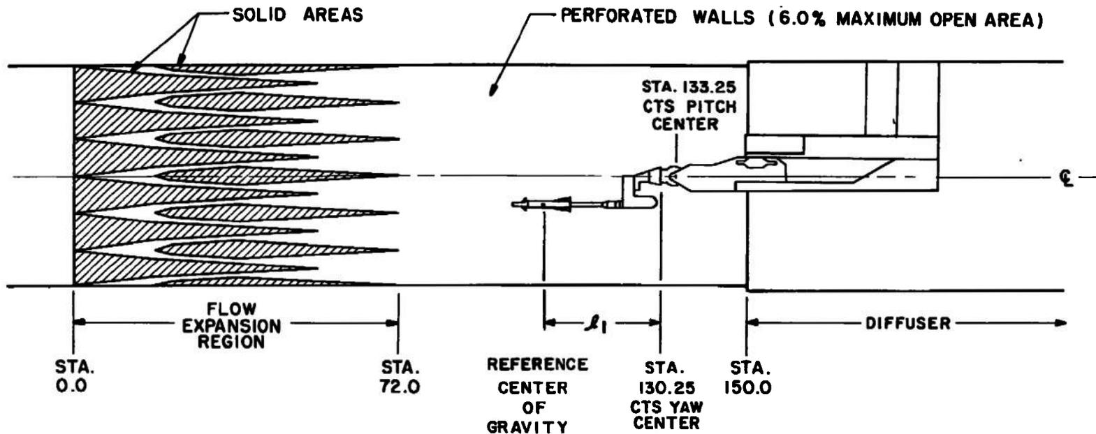
**Fig. 2 Schematic of the Tunnel 4T Test Section**
