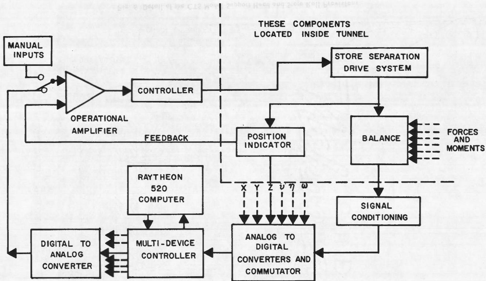
Fig. 7 Schematic of CTS Control System
