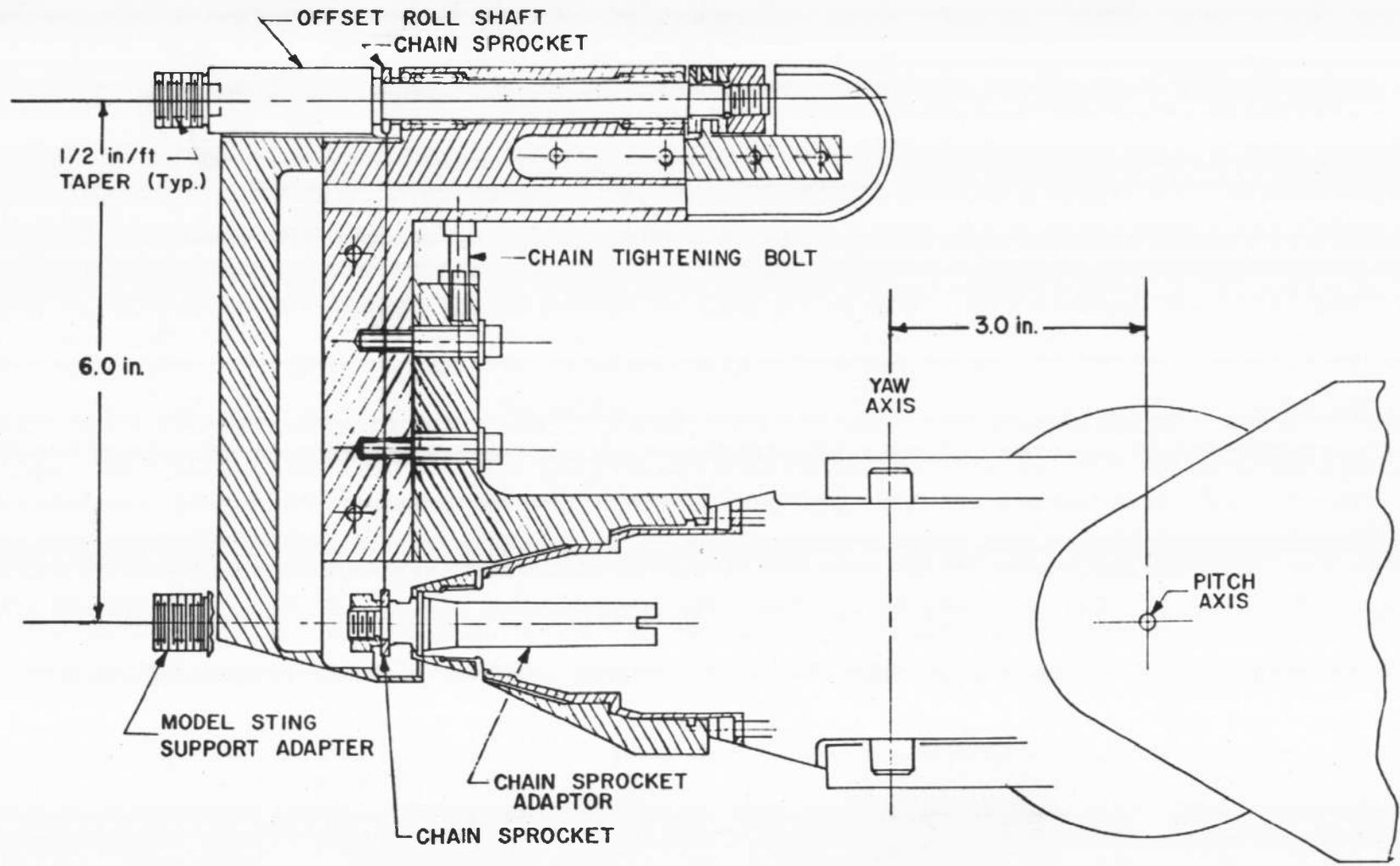
Fig. 6 Detail of the CTS Model Support Head and Store Roll Provisions
