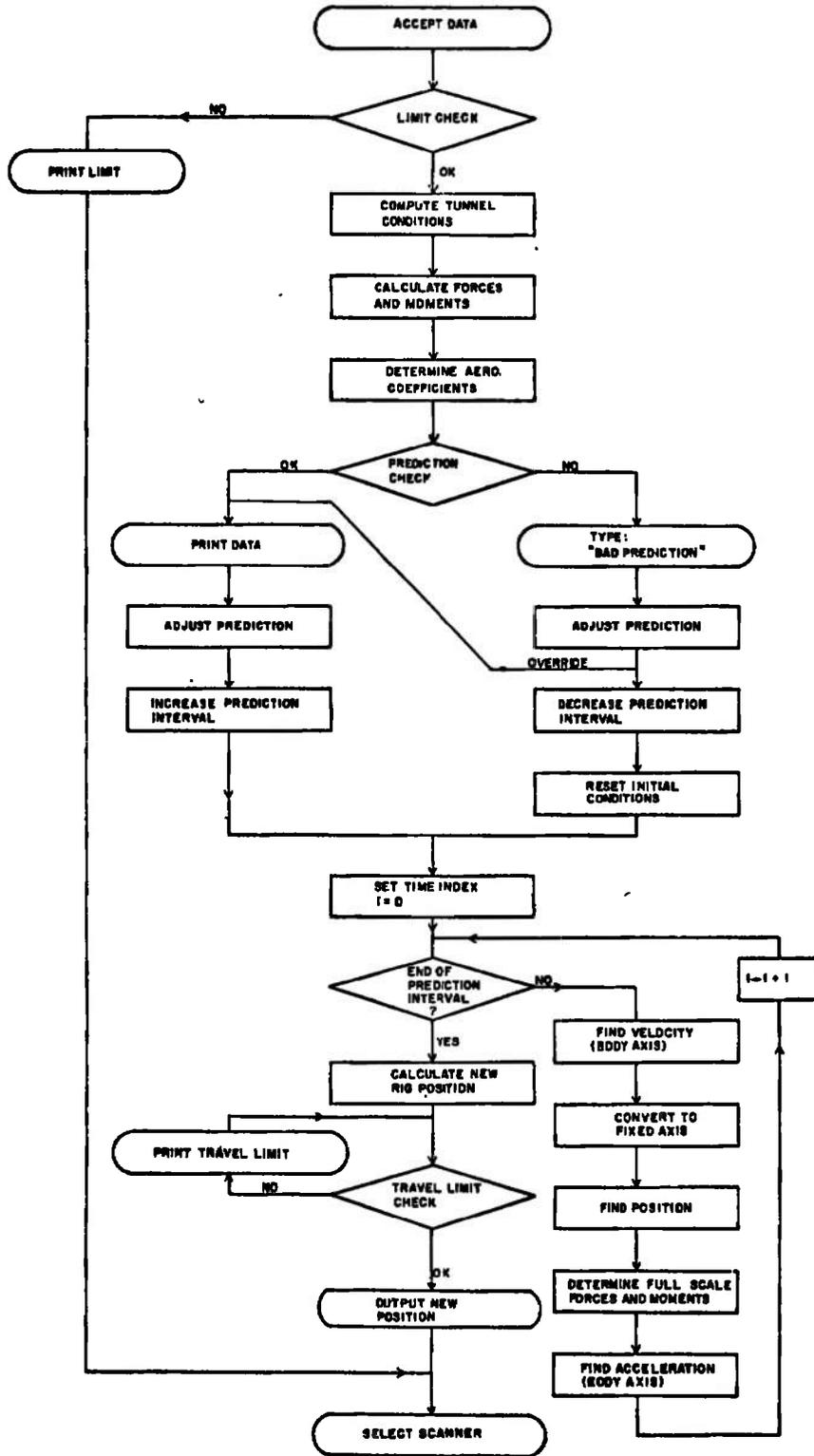
Fig. 10 Trajectory Generation Flow Diagram
