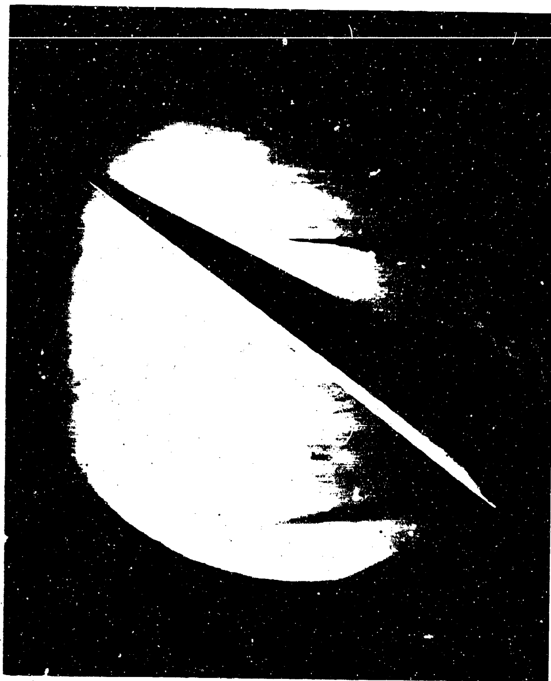
FIG. 40 SCHLIEREN PHOTOGRAPH OF AN INCLINED SLENDER CONE ( \alpha = 30^\circ )
