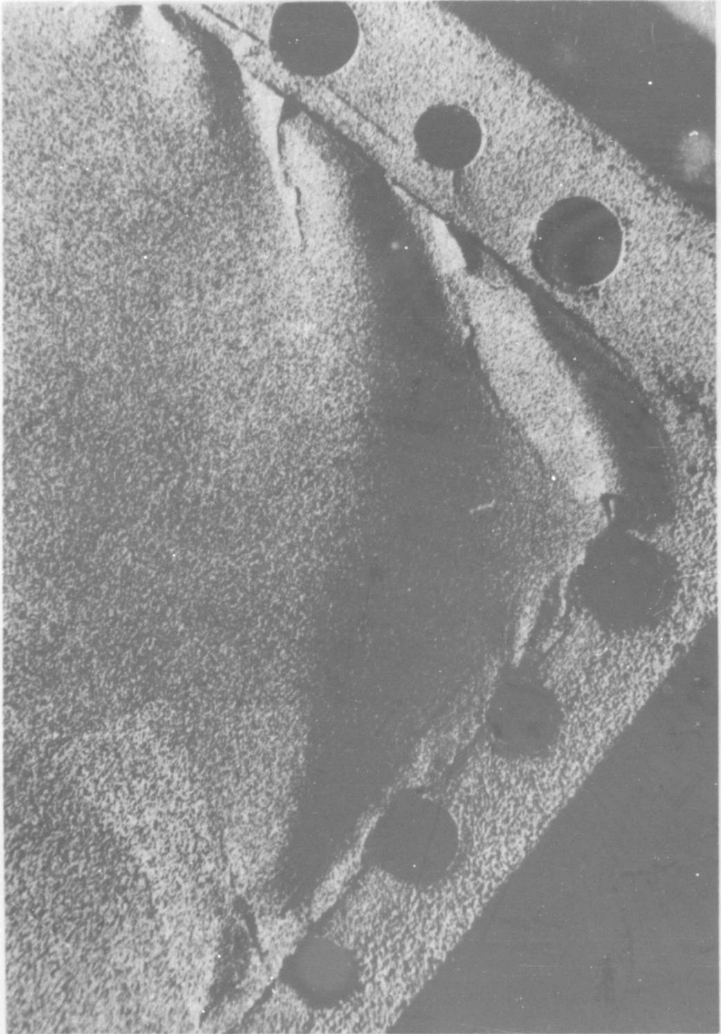
FIGURE 125 CLOSE UP OF FAILURE AT CORNER OF PANEL 8. CRACKING WAS ASSOCIATED WITH COATING ONLY AS PANEL EXHIBITED A DUCTILE TYPE FAILURE
