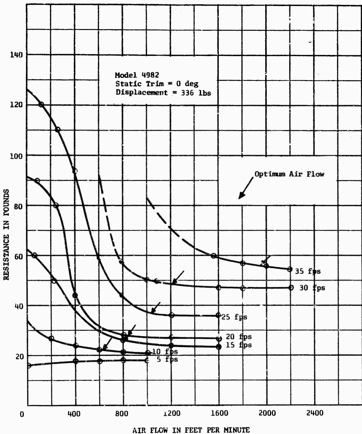
Figure 5 - Effect of Air Flow on Resistance
