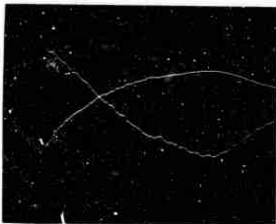
a. Inverted Trace: IR Detector Output, 40 mv/(div.). Normal Trace: Heat-flux Gage Temperature, 50°C/(div.). Sweep Rate: 5 maec/(div.) (Left to Right).
