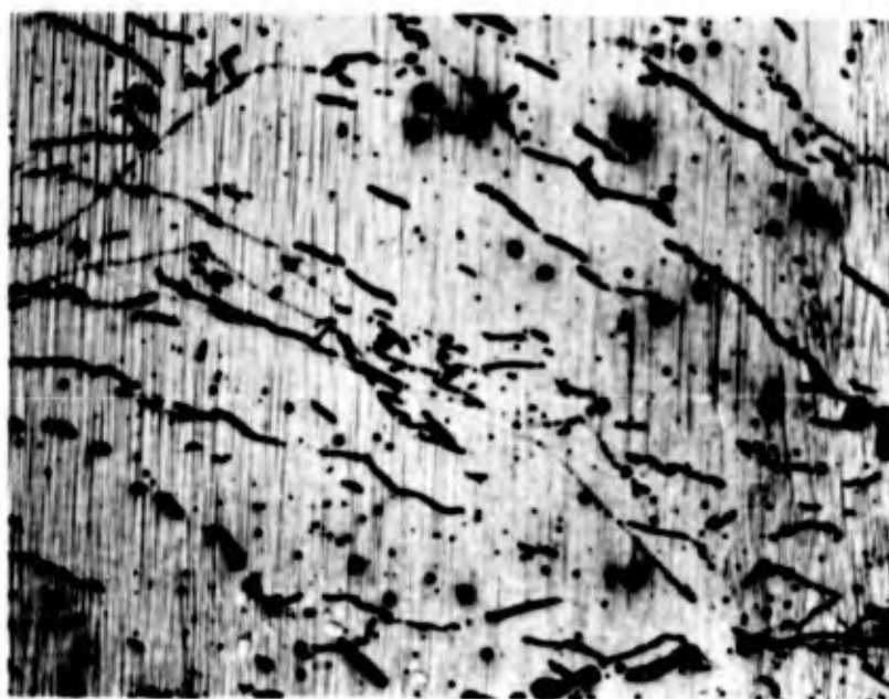
Figure 17. Diffusion Couple L (V,C) + C, V_2C -Zone X500 Diffusion Couple Reacted at 1800^\circ\text{C} , Then Reannealed for 15 Minutes at 800^\circ\text{C} .
