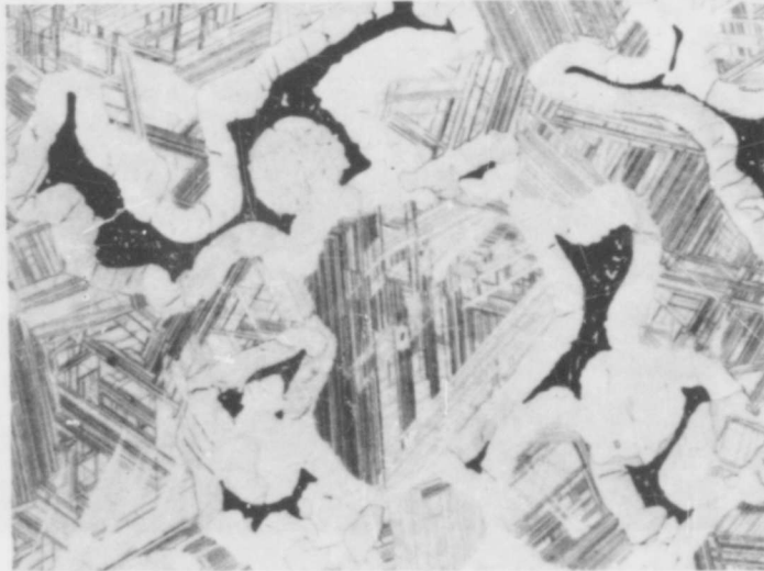
Figure 28. Nb-C (33.2 At.% C), Cooled at \sim 60^\circ\text{C} per Second from 3100 ^\circ\text{C} . X300
