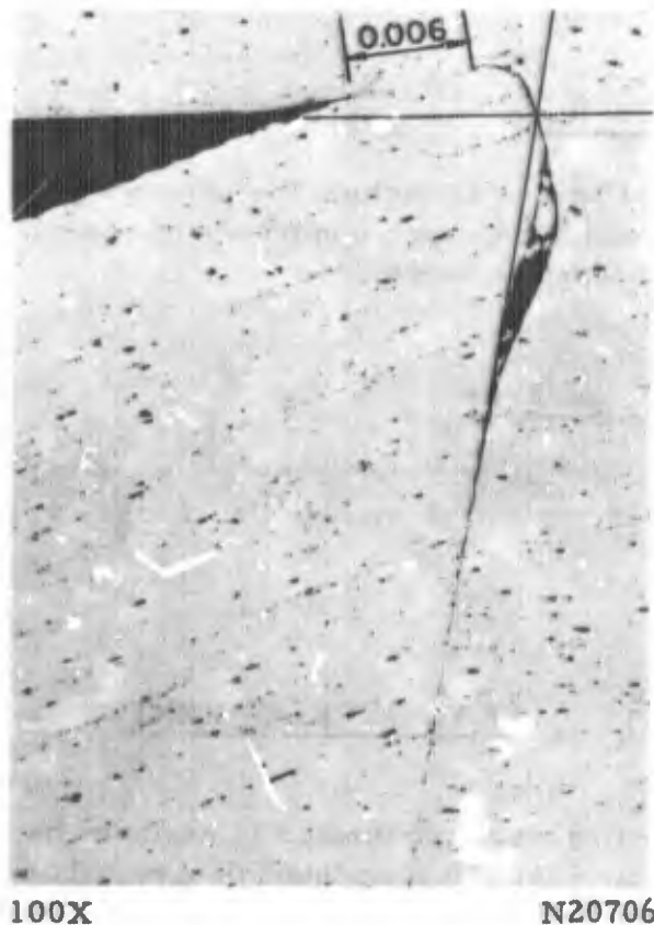
FIGURE 1. SEAL INTERFACE DAMAGE OF 6061-T6 SEAL IN 6061-T6 FLANGE AFTER FIFTEENTH REASSEMBLY
