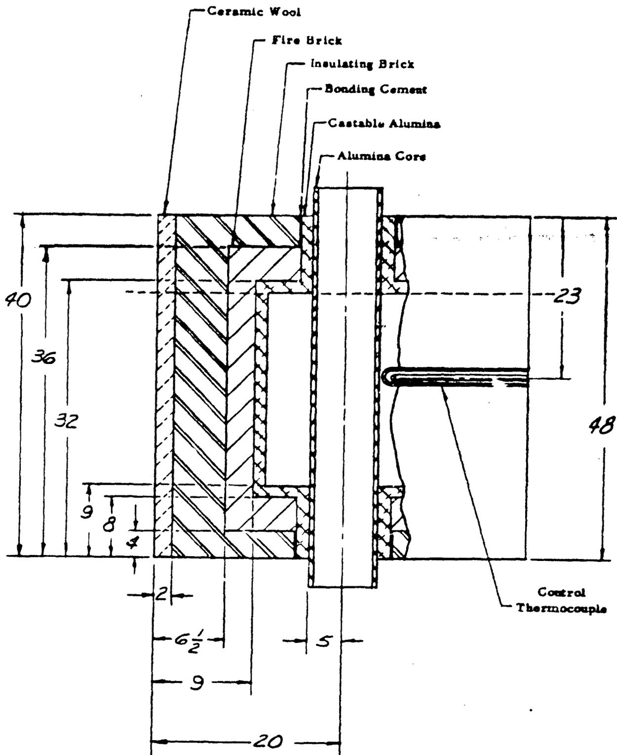
Figure 4 - Inside Cross-Section 10 Inch I.D. Furnace
