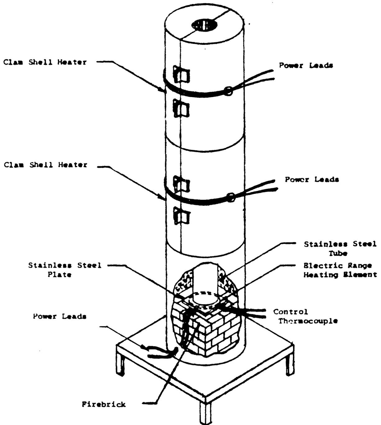
Figure 19 - Furnaces Used to Heat Autoclaves
