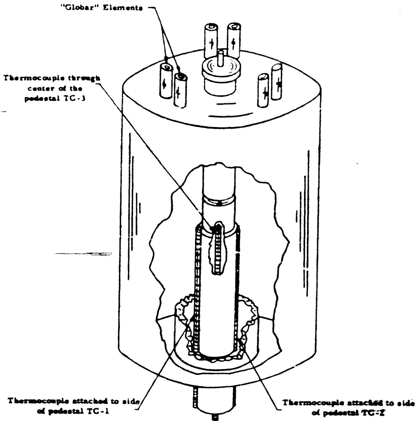
Figure 33 - Three Inch Furnace Showing Thermocouple Positions for Measuring Lateral Gradient
