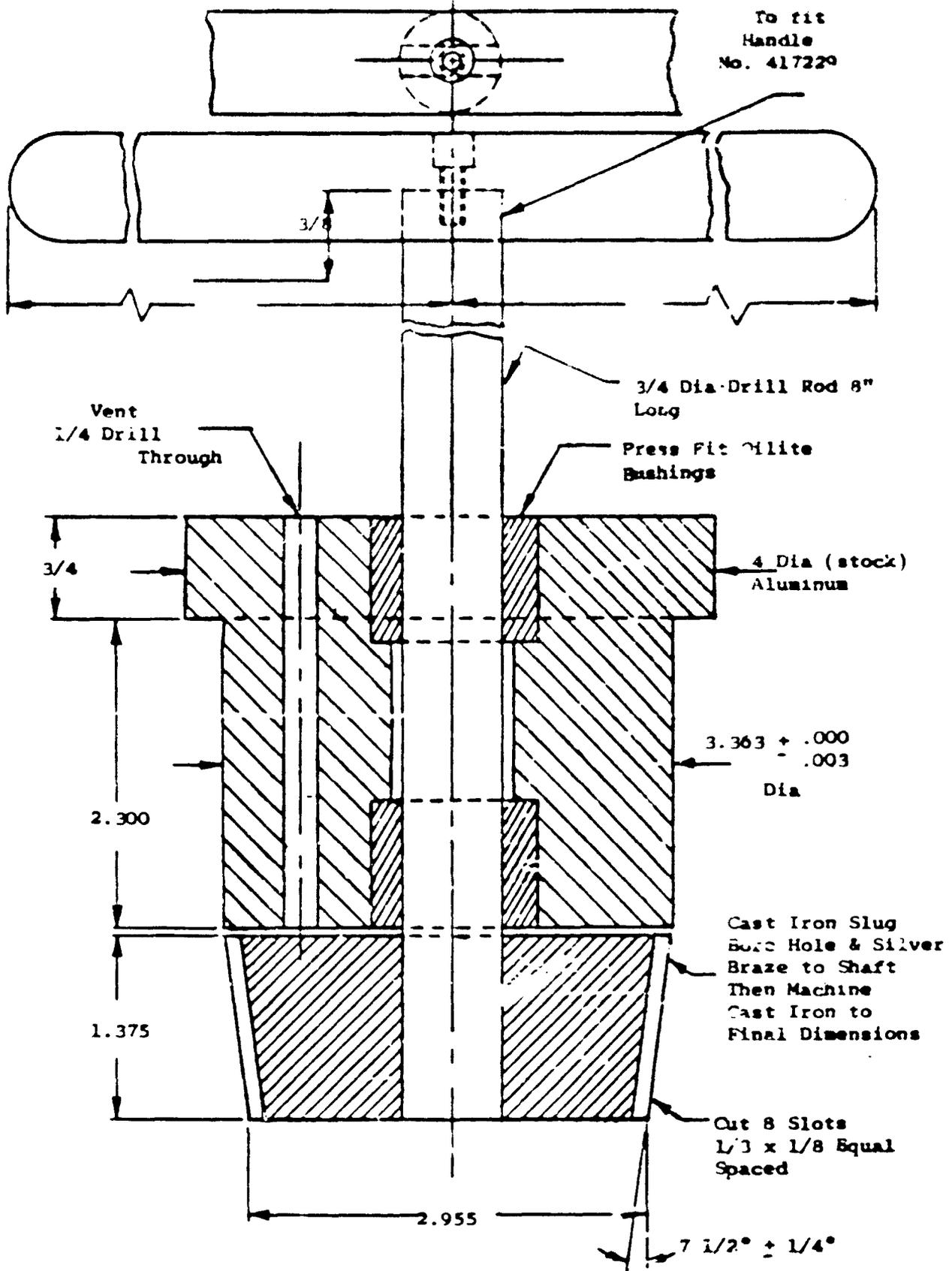
Figure 24 - Seal / ca Lapping Tool
