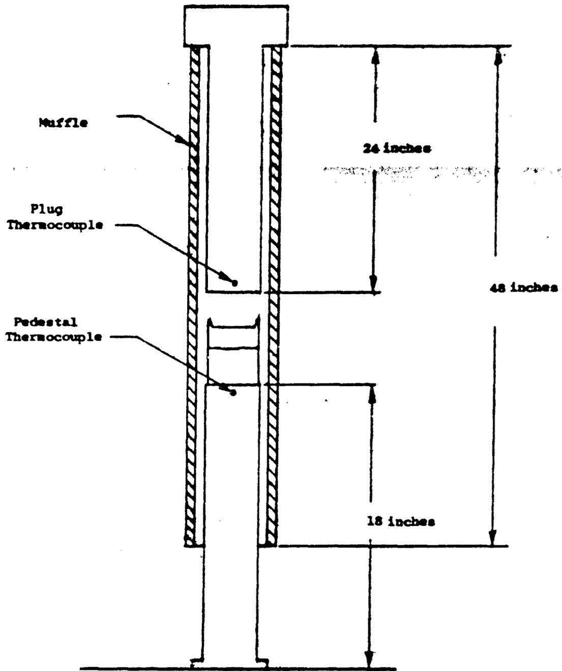
Figure 11 - 3 Inch Furnace Position Dimensions
