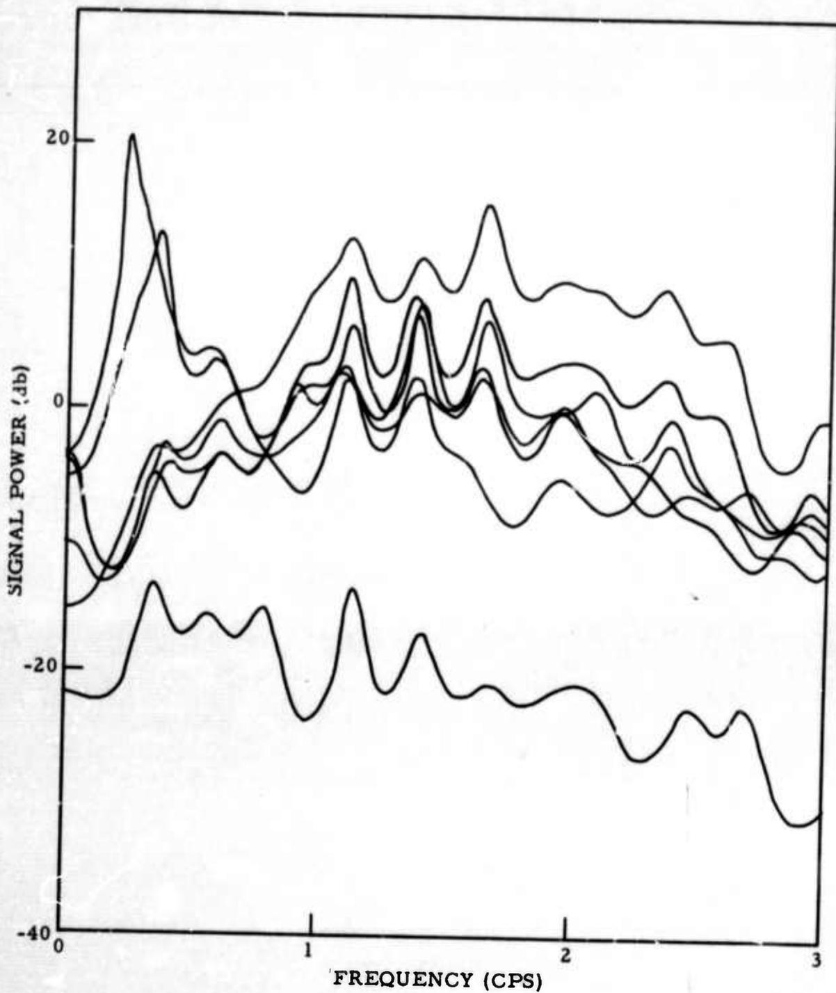
Figure 10. Signal Power Spectra of Seven Deep-Focus Events Between 30° and 31.3°
