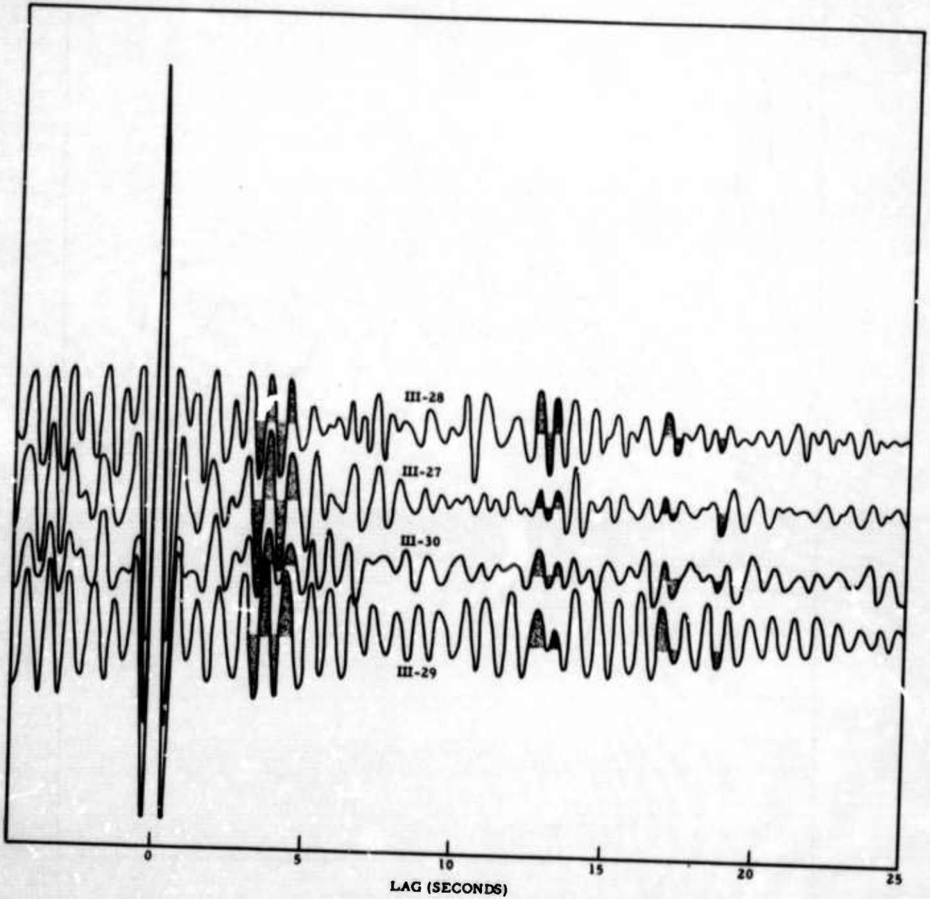
Figure 11. Autocorrelations of Four Teleseismic Signals from Earthquakes Near the Colombia-Venezuela Border
