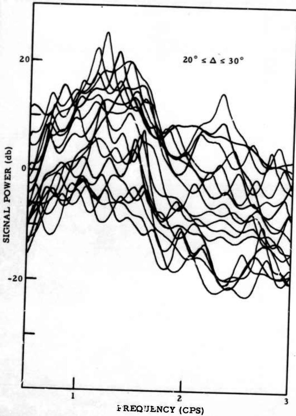
Figure 8. Signal Power Spectra of 16 Ensemble II Events Between 20° and 30°
