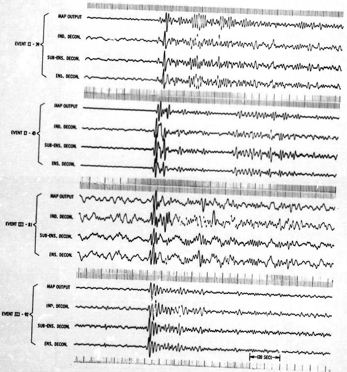
Figure 4. Original and Deconvolved Recordings of Four Events (1.5-cps High-Cut Playback Filter Applied)
