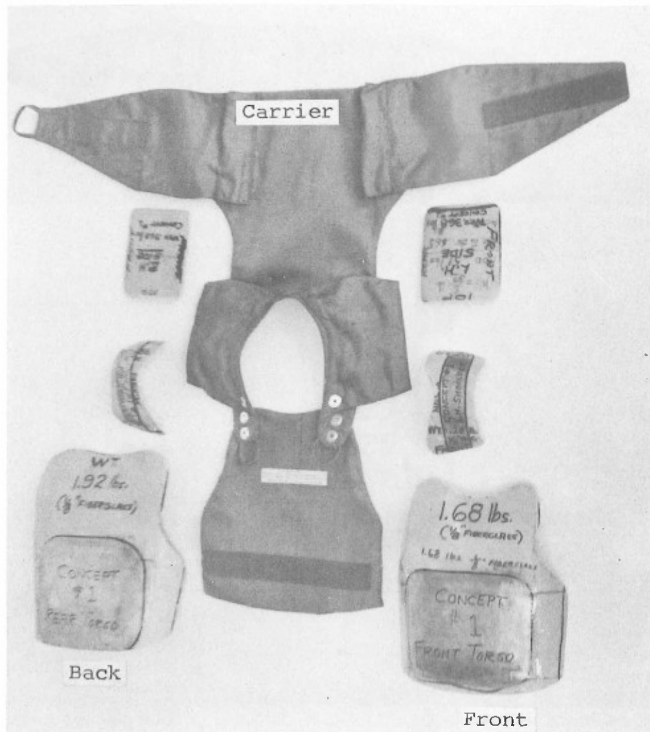
Figure 5. Model D Layout, Basic Carrier with Rigid Elements, Anatomically Contoured
