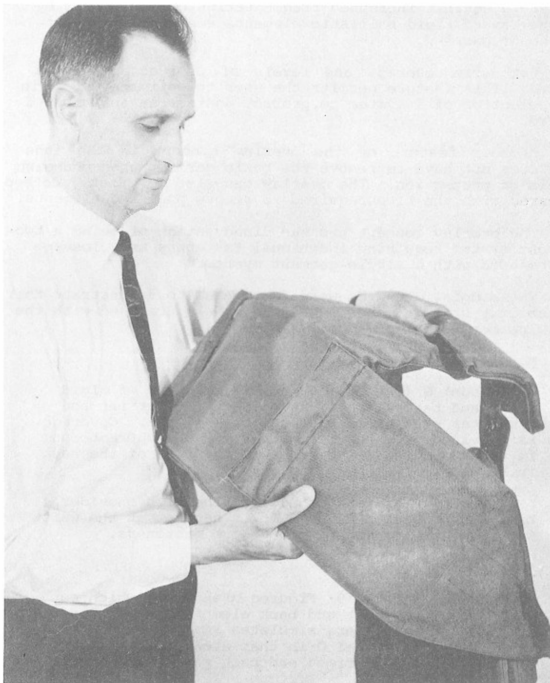
Figure 27. Model E, IITRI Rigid-Element Jacket, Rigid Articulated Rear Elements
