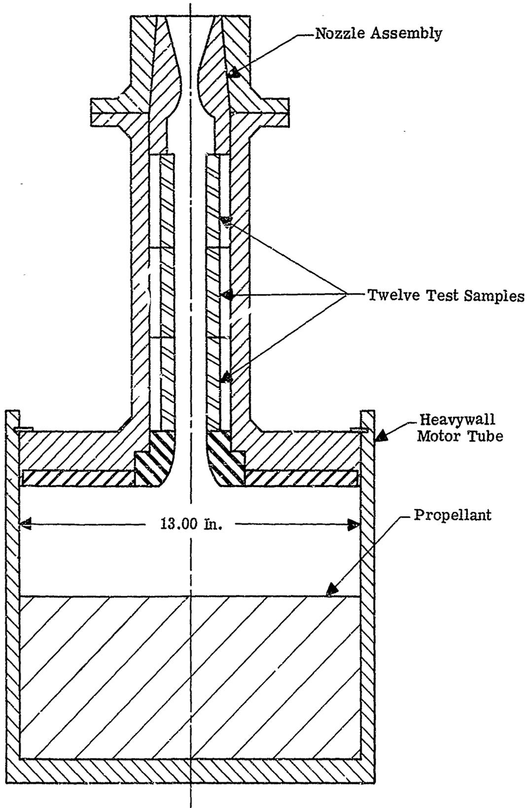
Figure 1. High Velocity Materials Evaluation Motor Assembly.
