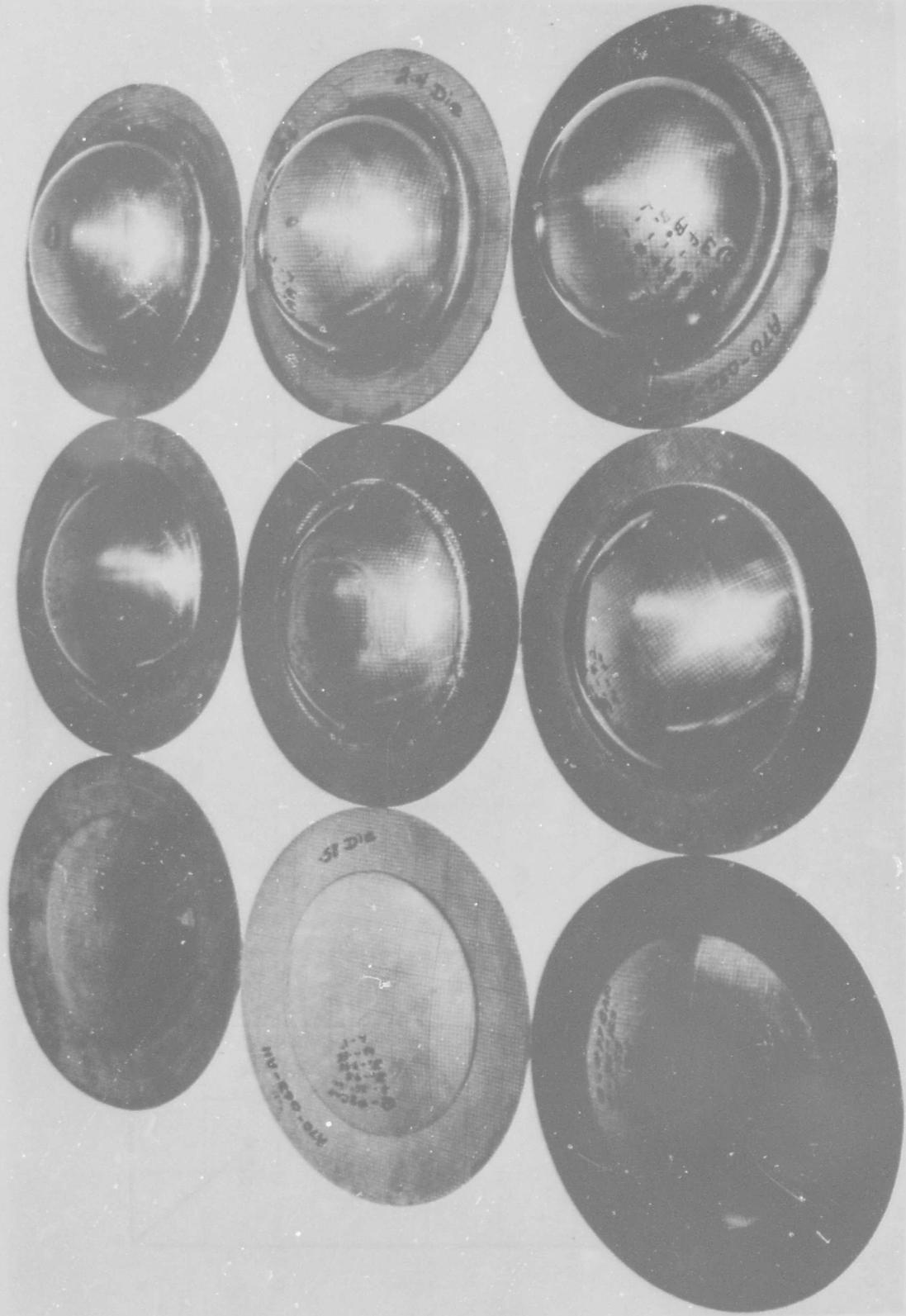
Figure 36 Deformed Specimens of T039-0 Aluminum Sheet Used to Establish the Relation Between Explosive Charge and Metal Draw Depth
