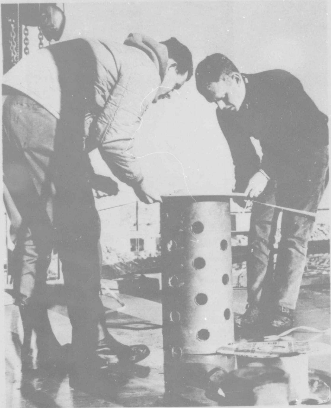
Figure 40 Explosive Standoff Installation for Full Scale Forming.
