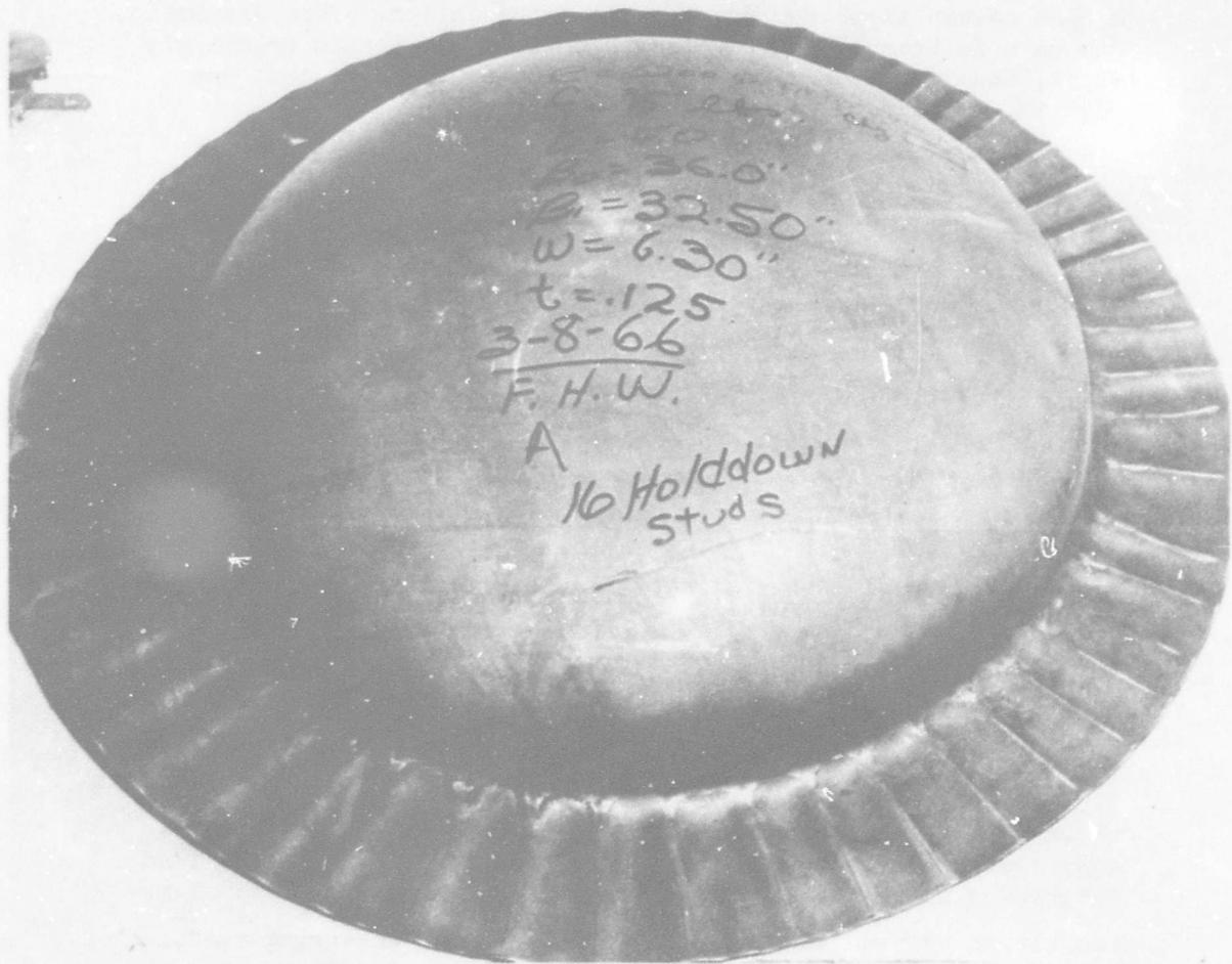
Figure 60 Flange Wrinkling of Explosively Formed D6AC Steel Sheet
