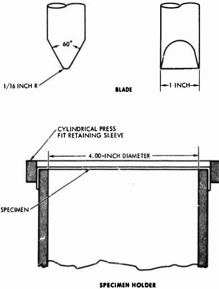
Figure 46. Puncture Test Blade and Specimen Holder, Type II, Classes A, B, and C Test.
