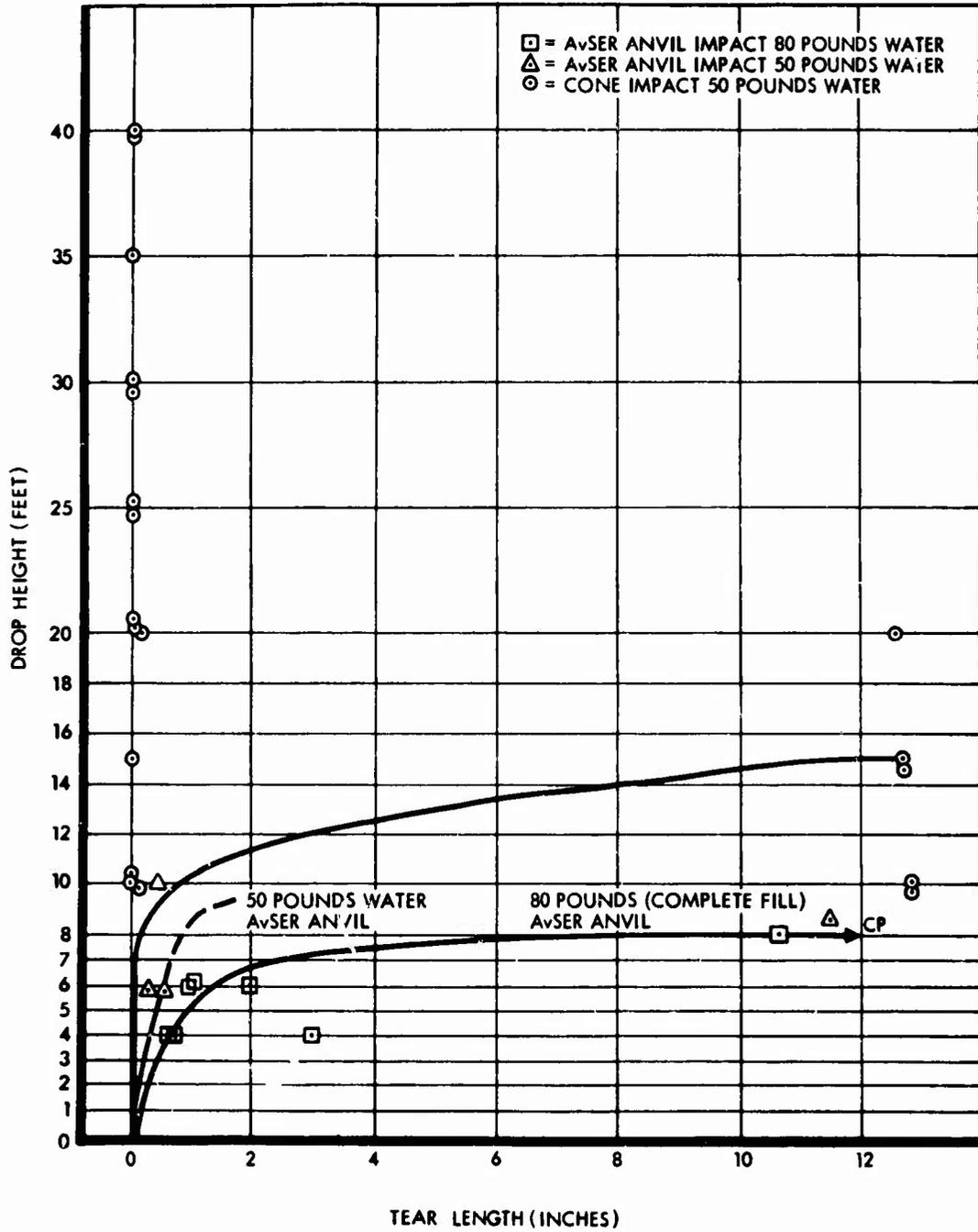
Figure 26. Cylindrical Tank Anvil Drop Test.
