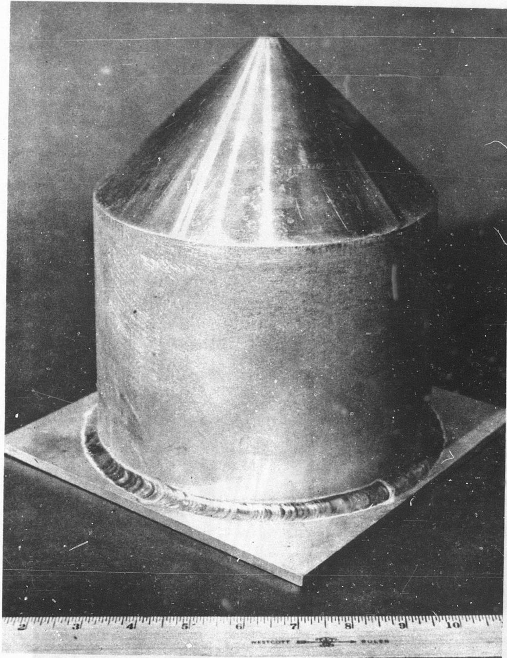
Figure 28. Drop Test Anvil (90 Degrees, 10 Inches High).
