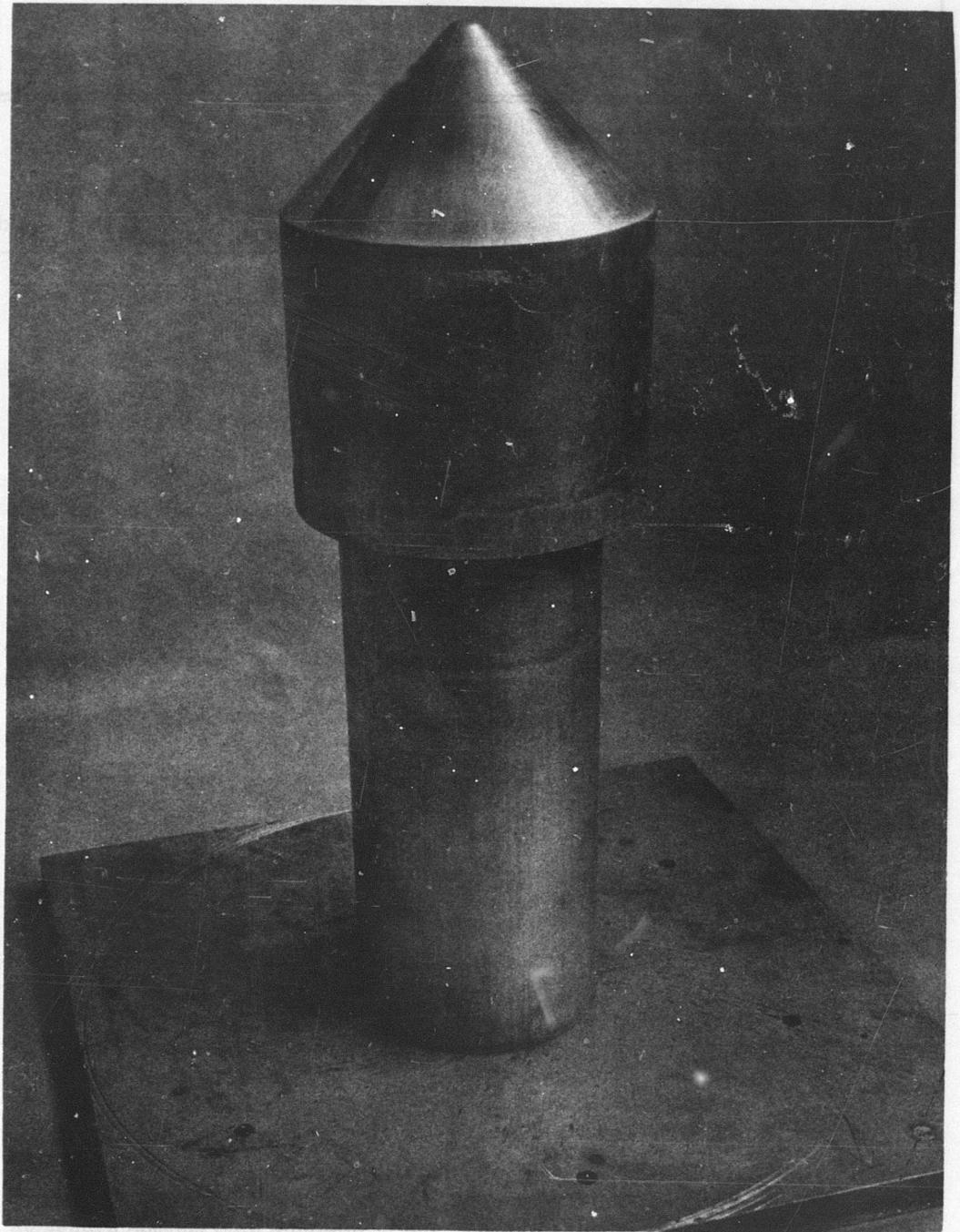
Figure 31. Drop Test Anvil (90 Degrees, 24 Inches High).
