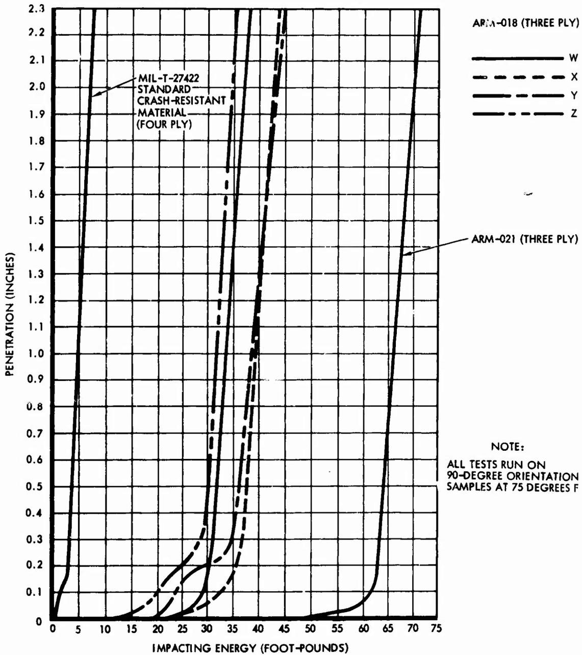
Figure 12. Puncture Resistance (Impacting Energy Versus Puncture Depth).
