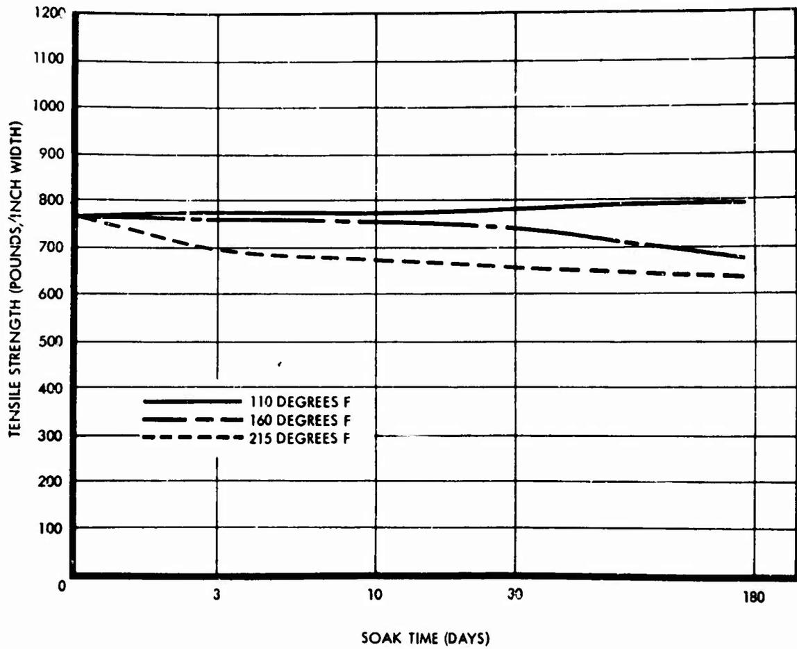
Figure 32. High Temperature Tensile Aging (W Resin, 20 Inches/Minute).
