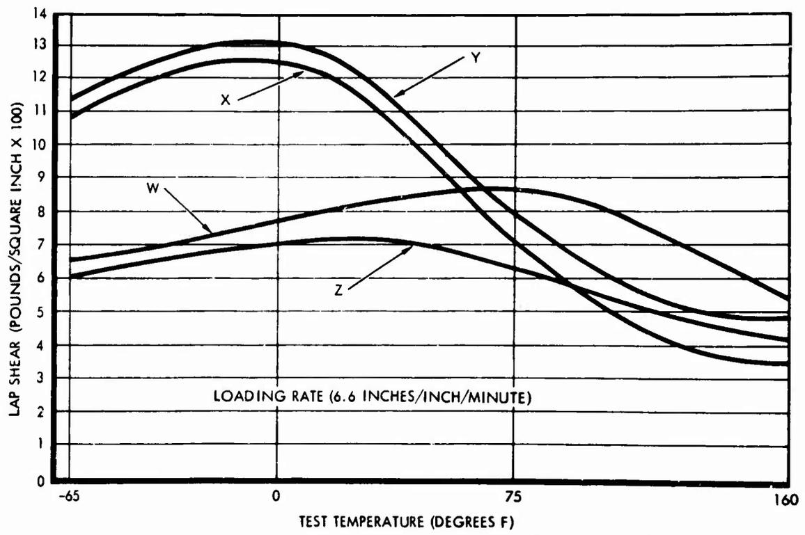
**Figure 8. Effect of Temperature on Lap Shear Strength.**
