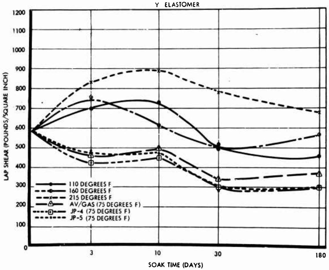
Figure 36. Heat and Fuel Soak (Y Lap Shear).
