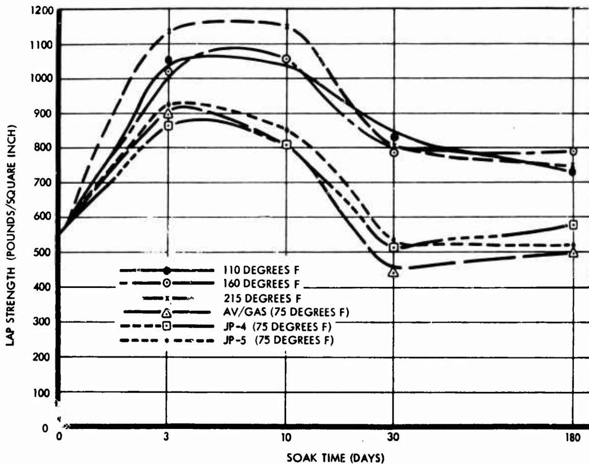
Figure 34. Heat and Fuel Soak (W Lap Shear)
