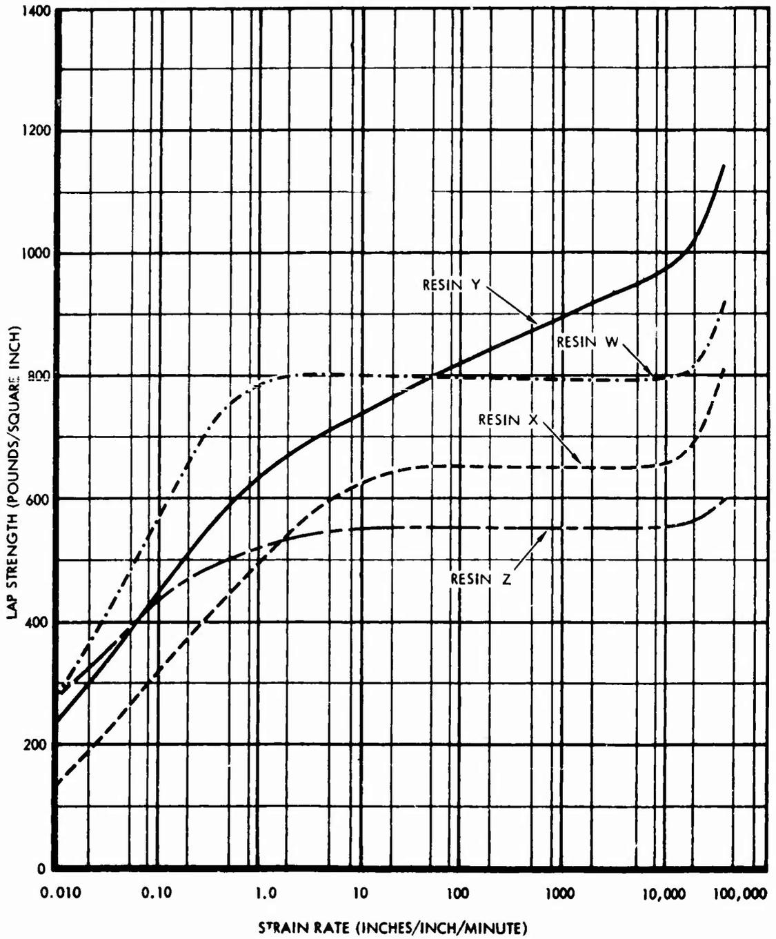
Figure 7. Lap Shear Test (Test Temperature 75 Degrees F).
