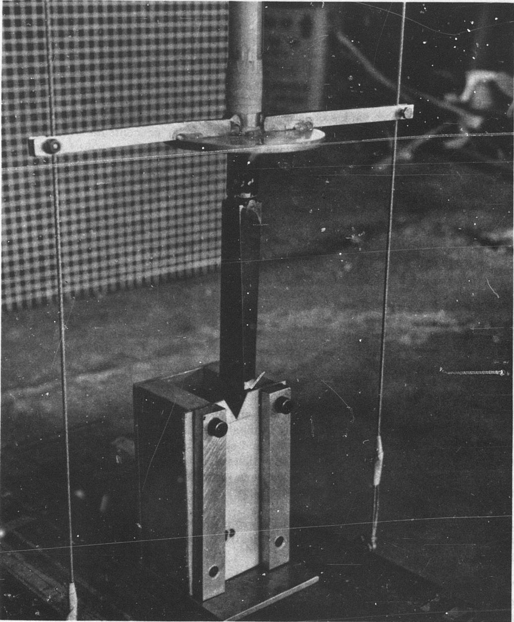
Figure 16. Edgewise Tear Test Apparatus and Mounted Specimen.
