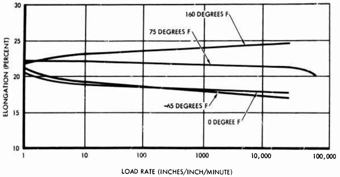
Figure 4. Elongation Versus Rate of Loading, ARM-018 W Laminate.
