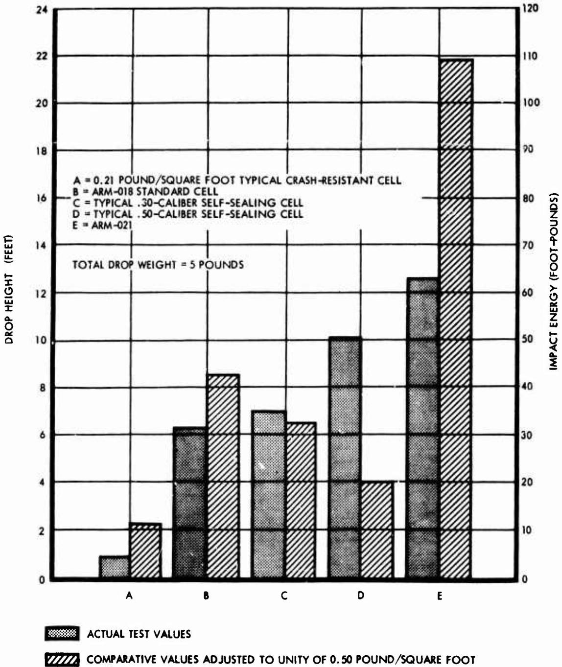
Figure 15. Puncture Resistance.
