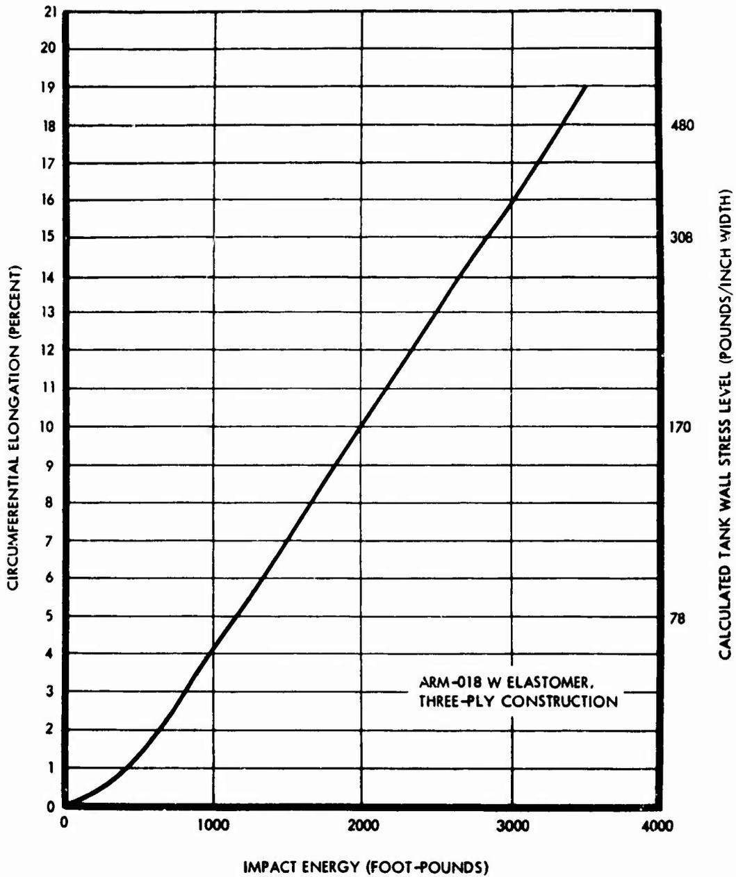
Figure 25. Cylindrical Tank Flatwise Impact Drop Test.
