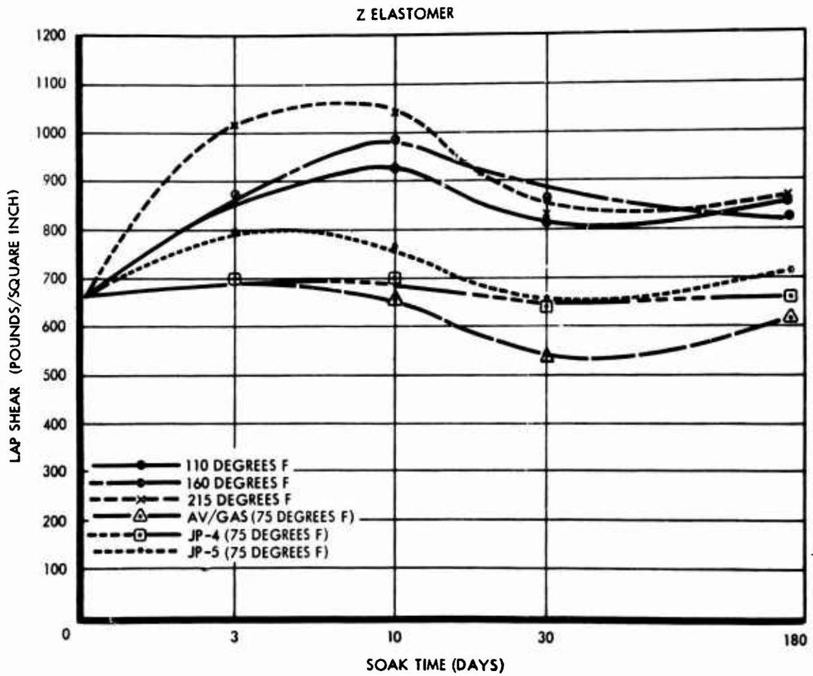
Figure 37. Heat and Fuel Soak (Z Lap Shear).
