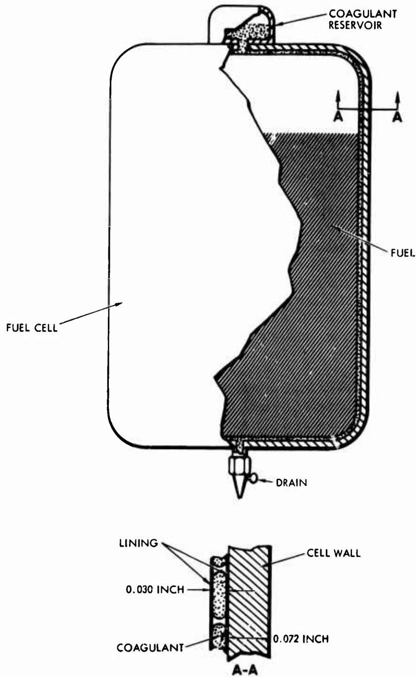
Figure 1. Basic Coagulant-Lined Fuel Cell.
