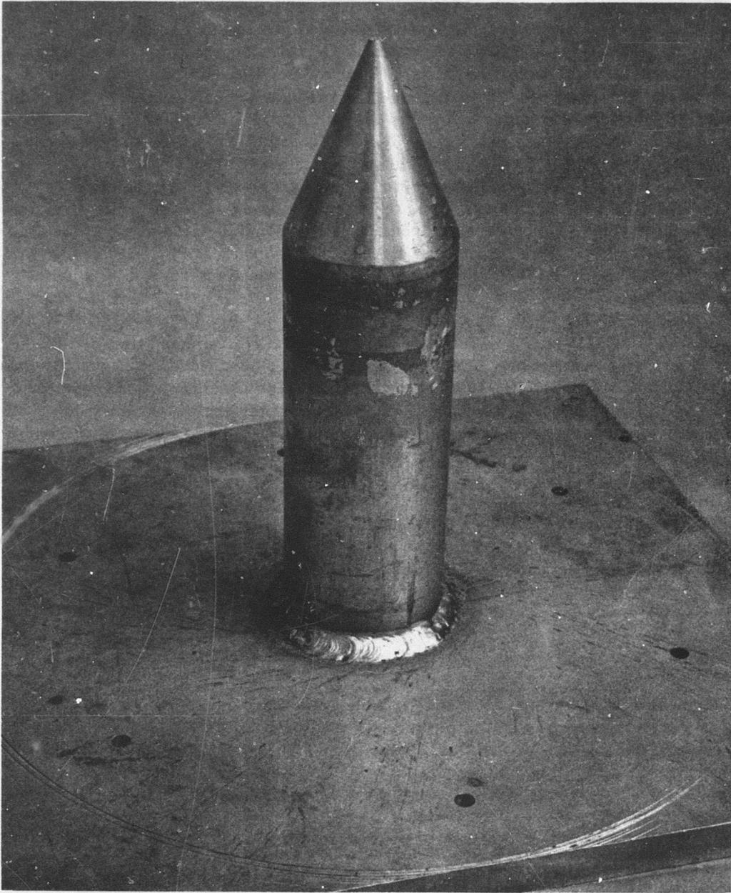
Figure 30. Drop Test Anvil (45 Degrees, 4-Inch Diameter, 15 Inches High).
