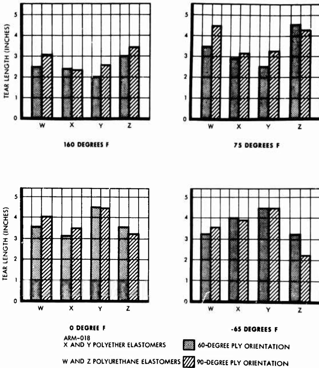
COMPARATIVE RESULTS SHOWN ARE RESULTANT TEARS CAUSED BY 20-FOOT DROPS OF A 5-POUND DART.
