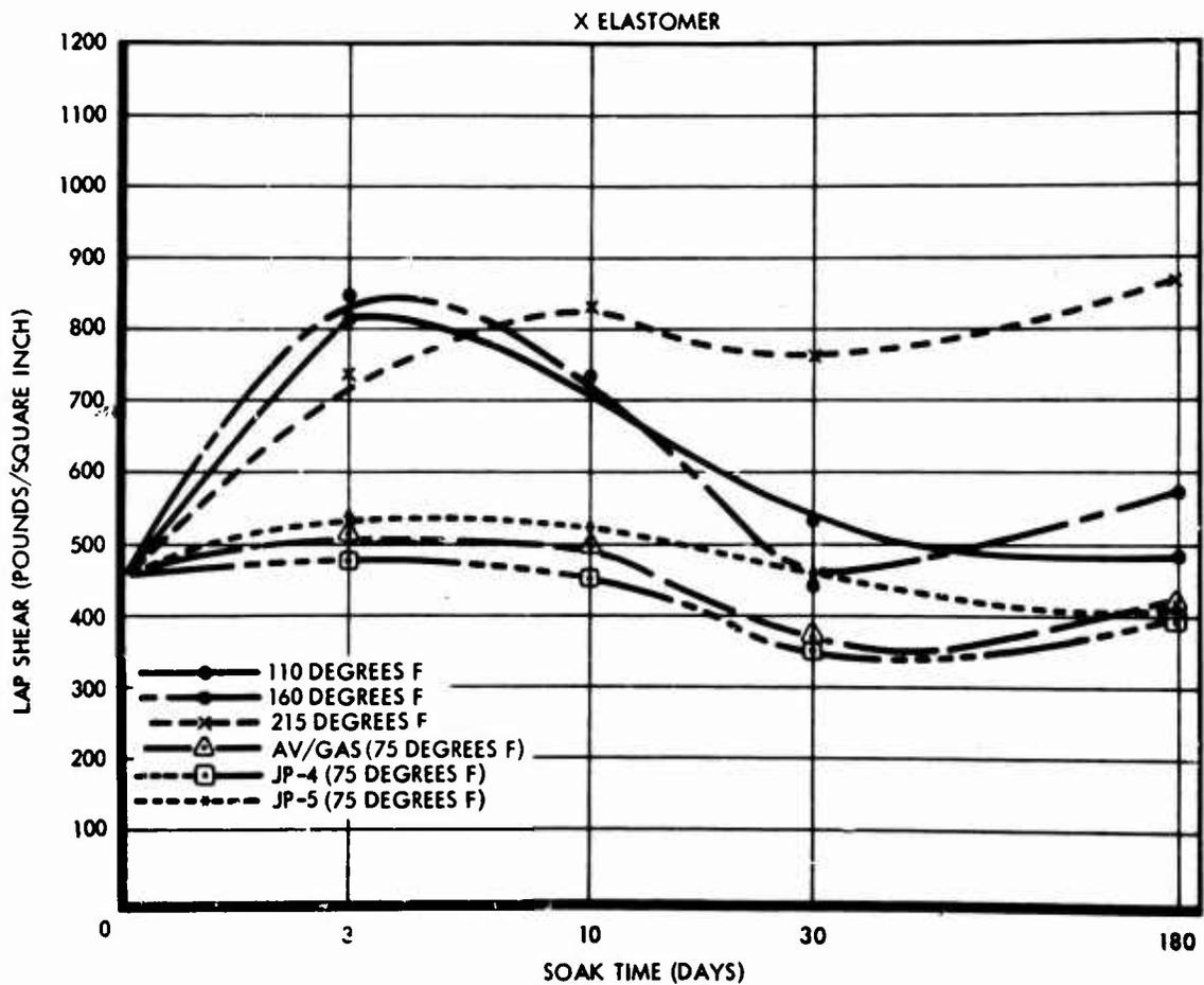
Figure 35. Heat and Fuel Soak (X Lap Shear).
