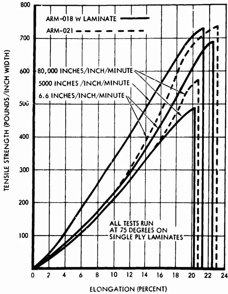
Figure 3. Typical Load-Elongation Curves at Various Loading Rates.
