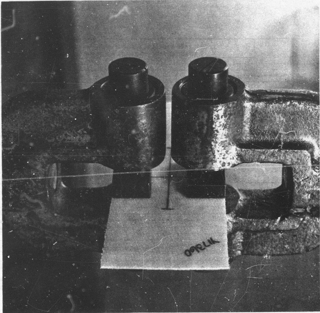
Figure 21. Constant Rate Tear Test.
