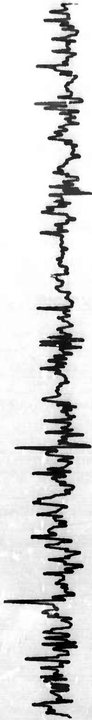
Figure 10. Noise recorded on 13 July 1965 on ocean bottom at 72°03'W, 36°11'N. Depth of water 3600m. Magnification 125K at 1 Hz
