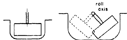
Figure 10-3. Increase in Radome Size for Roll-Stabilized Antenna
