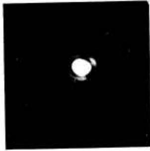
Figure D6a. Photograph of Fraunhofer Diffraction Pattern for 1.5" Diameter Aperture, 0.6328 Micron Wavelength, and Measuring Optics Only.
