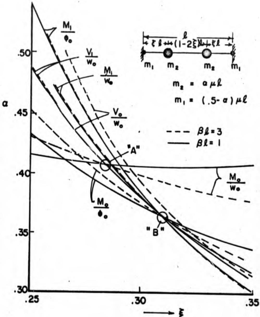
FIG. 2 OPTIMIZING CONDITION, CLAMPED-CLAMPED BEAM
