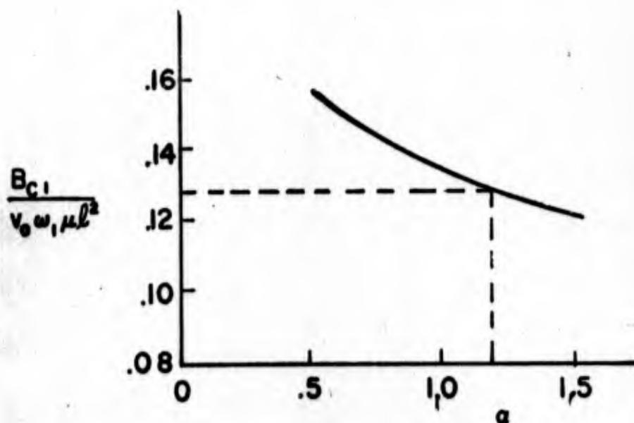
FIG. C-4(b) FIRST MODE BENDING MOMENT VS.  $\alpha$
