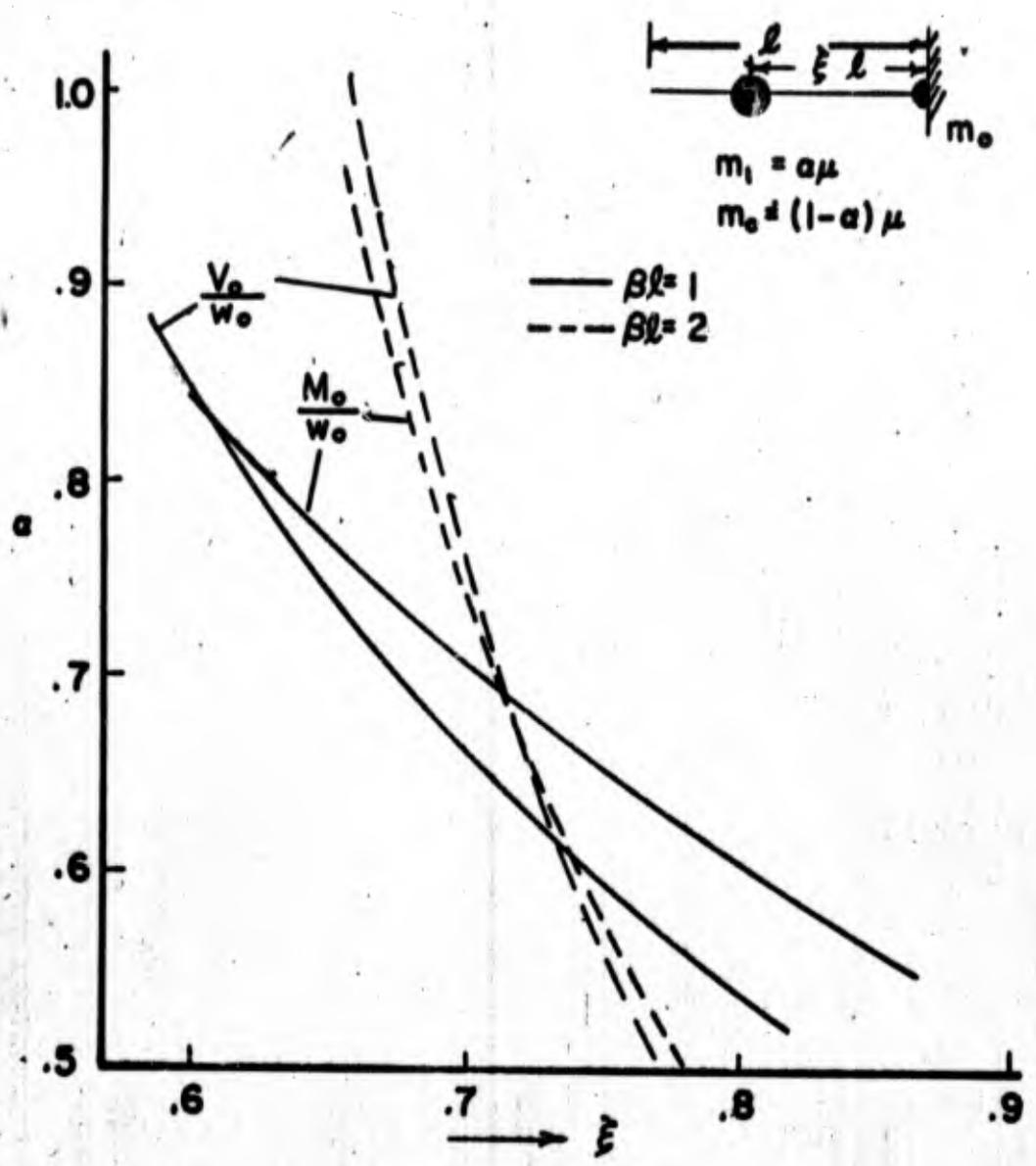
FIG. A-7 OPTIMIZING CONDITION FOR CLAMPED-FREE BEAM
