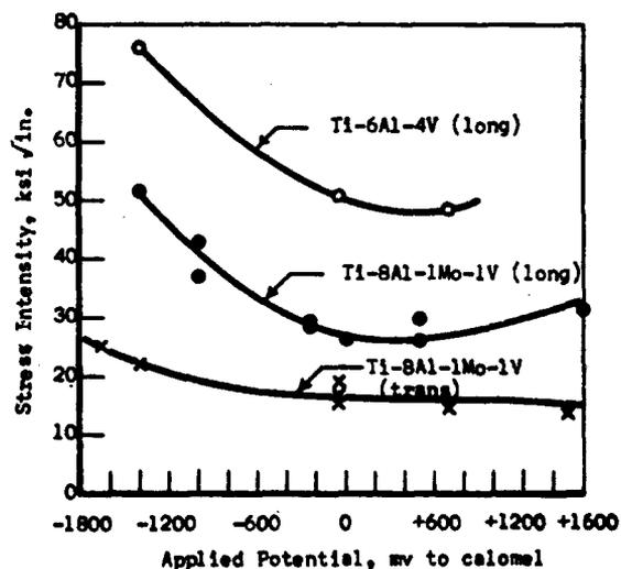
FIGURE 19. THE EFFECT OF APPLIED POTENTIAL ON THE STRESS INTENSITY FACTOR TO CAUSE FAILURE IN 3-1/2 PERCENT SALT WATER<sup>(41)</sup>
