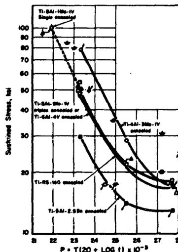
FIGURE 4. APPLICATION OF LARSEN-MILLER PARAMETER FOR PREDICTING STRESS-CORROSION CRACKING BY HOT SALT OF ANNEALED TITANIUM ALLOYS<sup>(10,12)</sup>
