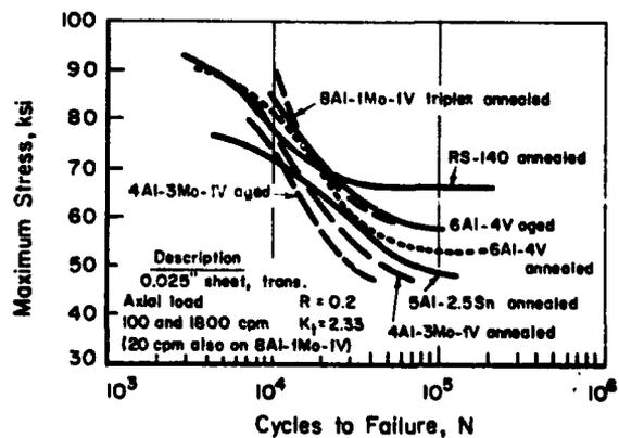
FIGURE 11. CORROSION FATIGUE OR AIR FATIGUE (SAME) S-N CURVES FOR TITANIUM ALLOYS<sup>(16)</sup>
