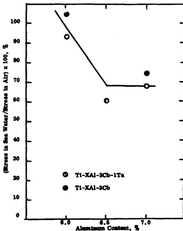
FIGURE 15. EFFECT OF ALUMINUM CONTENT ON THE SEAWATER TO AIR FAILURE STRESS RATIO OF BETA-ANNEALED PLATE<sup>(39)</sup>
