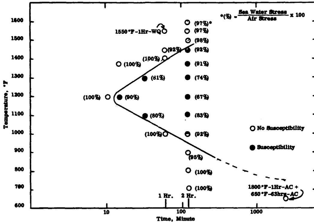
FIGURE 17. EFFECT OF EXPOSURE TEMPERATURE AND TIME ON THE STRESS-CORROSION CRACKING OF Ti-8Al-1Mo-1V PLATE IN ROOM TEMPERATURE SYNTHETIC SEAWATER<sup>(39)</sup>
