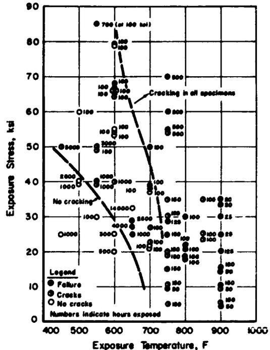
FIGURE 1. EFFECT OF EXPOSURE VARIABLES ON THE OCCURRENCE OF VISIBLE SALT STRESS-CORROSION IN Ti-8Al-1Mo-1V(7)
