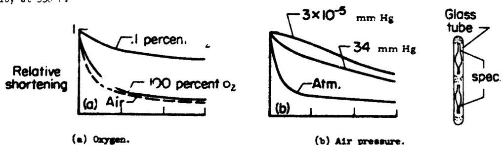
FIGURE 8. EFFECT OF OXYGEN AND AIR PRESSURE ON SALT STRESS CORROSION OF DUPLEX ANNEALED Ti-8Al-1Mo-1V ALLOY SHEET AT 550 F.<sup>(9)</sup> (See also Figure 5)
