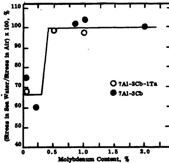
FIGURE 16. EFFECT OF MOLYBDENUM CONTENT ON THE SEAWATER TO AIR FAILURE STRESS RATIO OF BETA-ANNEALED PLATE<sup>(39)</sup>
