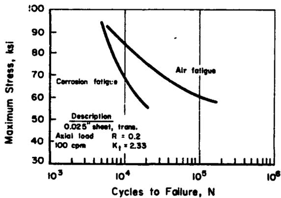
FIGURE 10. CORROSION FATIGUE AND AIR-FATIGUE S-N CURVES FOR Ti-8Al-1Mo-1V TRIPLEX ANNEALED<sup>(10)</sup>
