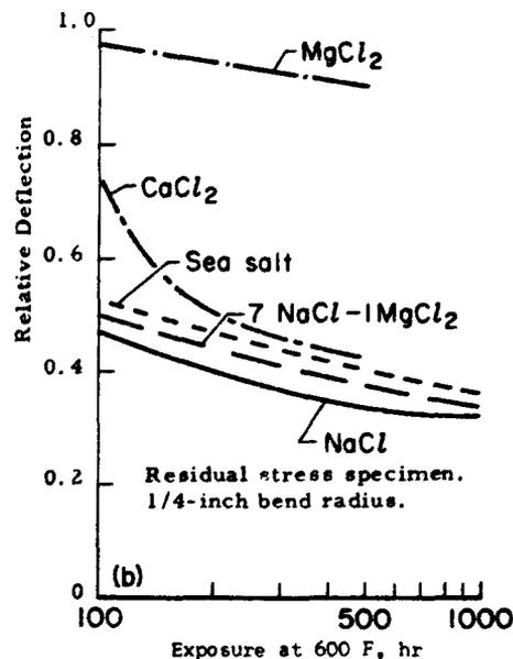
FIGURE 6. EFFECT OF TYPE OF SALT ON STRESS CORROSION OF DUPLEX ANNEALED Ti-8Al-1Mo-1V ALLOY SHEET AT 600 F<sup>(9)</sup>
