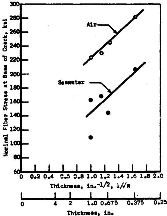
FIGURE 18. EFFECT OF PLATE THICKNESS AND TESTING MEDIA ON THE NOMINAL FIBER STRESS AT FAILURE IN PRE-CRACKED BETA-ANNEALED Ti-7Al-2Cr-1Ta ALLOY, THREE-POINT BEND SPECIMENS(35)
