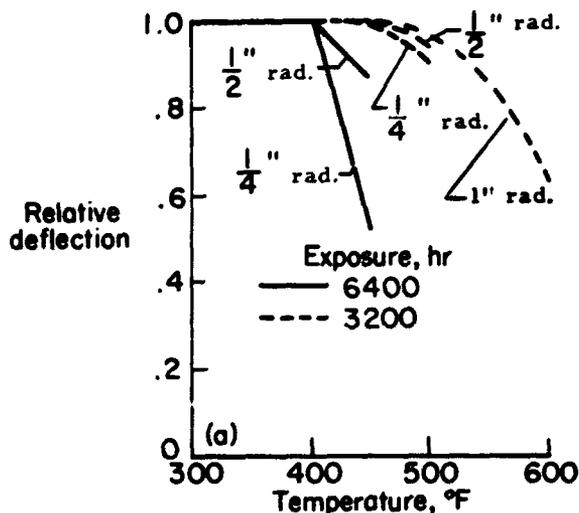
FIGURE 3. STRESS-TEMPERATURE THRESHOLDS FOR DUPLEX ANNEALED Ti-8Al-1Mo-1V RESIDUAL STRESS SPECIMENS<sup>(9)</sup>
