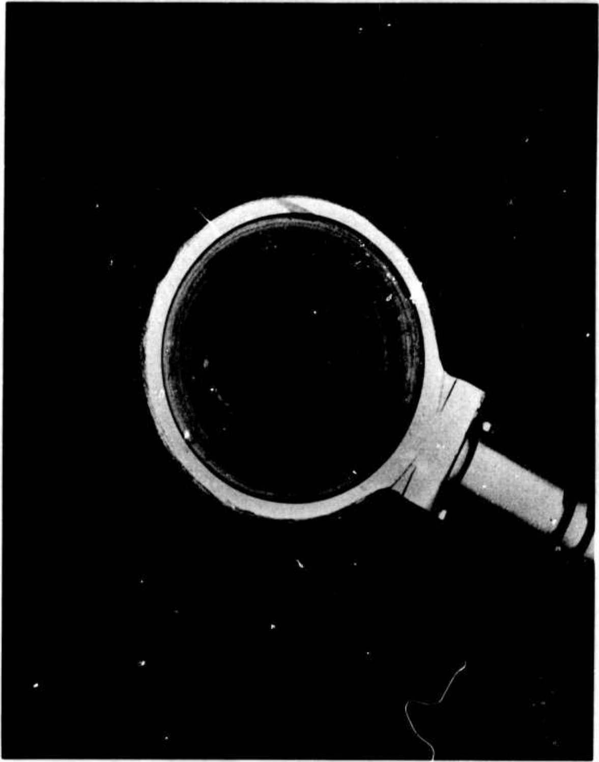
Figure 71 Anode After 100-Hour Test (cleaned)
