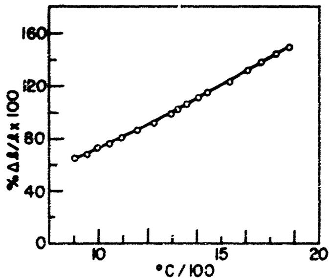
Figure 31. Thermal Expansion of HfB<sub>2</sub>-LaB<sub>6</sub> Composite
