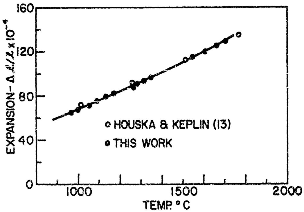
Figure 20. Thermal Expansion of 78 Percent Dense ZrB<sub>2</sub>
