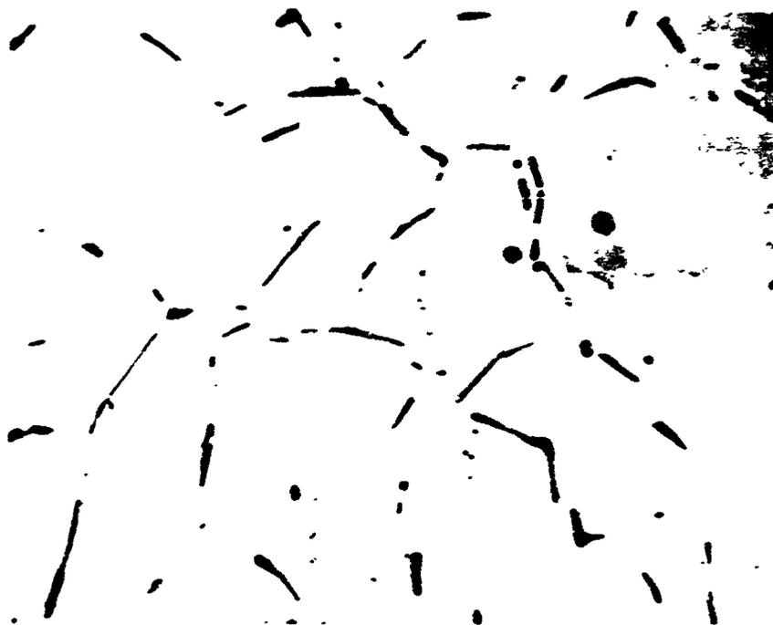
Figure 42. Photomicrograph of Polycrystalline ZrC Showing a Small Amount of Graphite in the Form of Flakes
