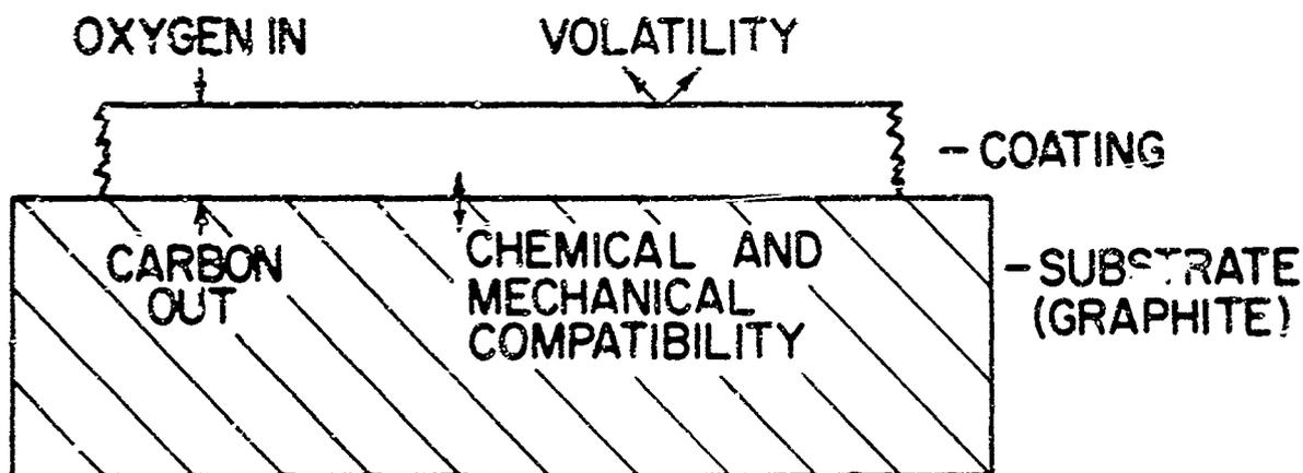
Figure 1. Factors Controlling the Oxidation Protection of Graphite
