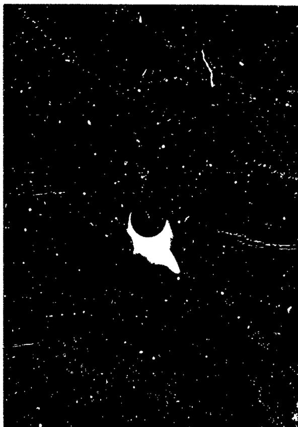
Figure 57. Laue Back-Reflection Photograph of Single Crystal  $ZrB_2$ . The Axis of the Crystal Is Nearly Parallel to the (00.1) Pole. The Area Corresponds to That Shown in Figure 54
