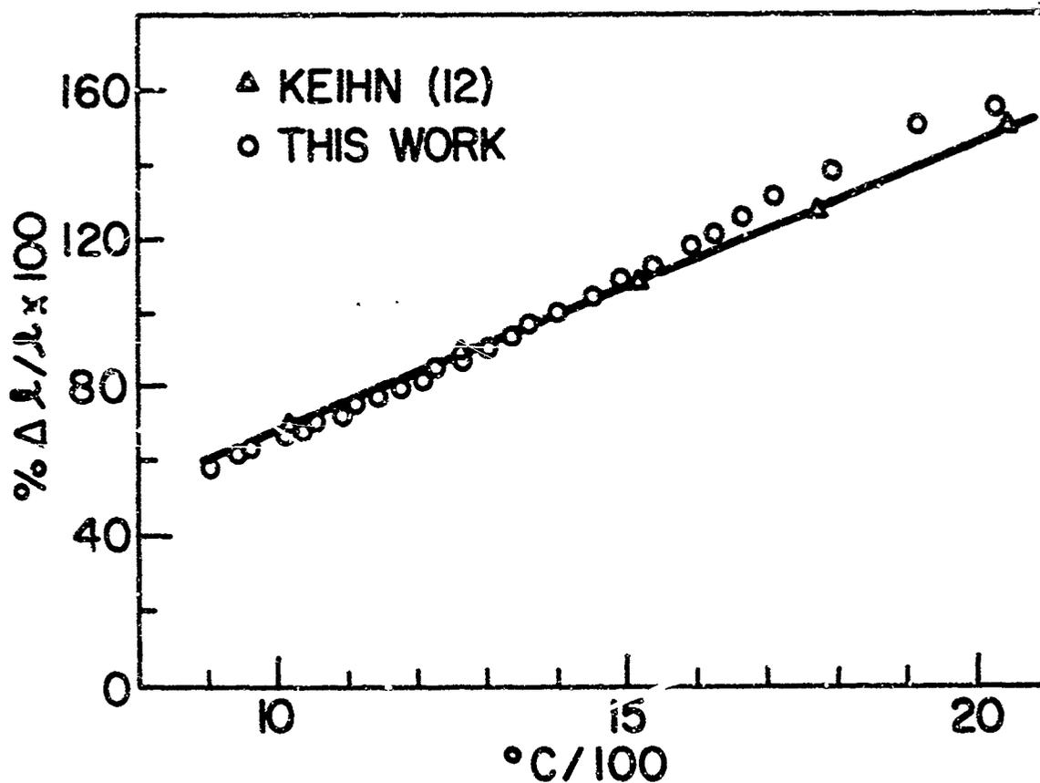
Figure 29. Thermal Expansion of 74.6 Percent Dense  $\text{HfB}_2$
