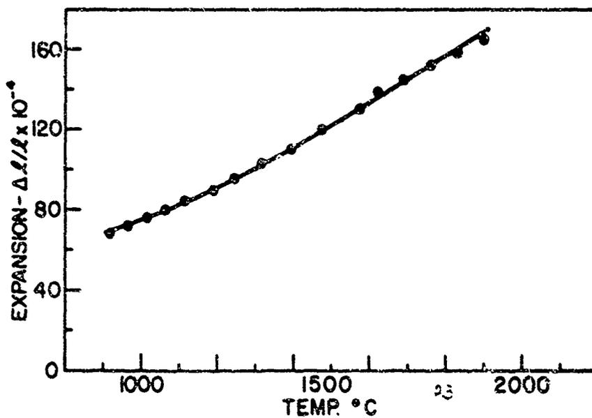
Figure 23. Thermal Expansion of ZrB<sub>2</sub>-LaB<sub>6</sub> Composite
