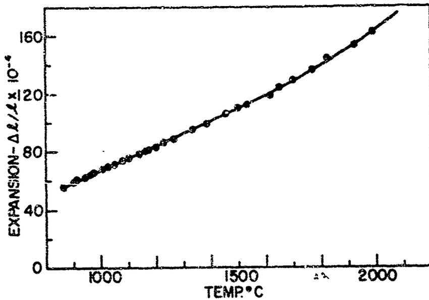
Figure 22. Thermal Expansion of ZrB<sub>2</sub>-CeB<sub>6</sub> Composite
