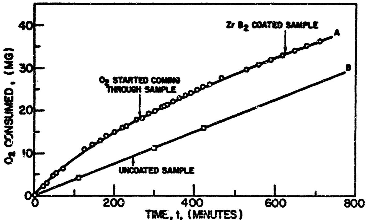
Figure 61. Oxygen Consumption Versus Time for Thoria Coated With ZrB<sub>2</sub> (A) and for Uncoated Thoria (B), Runs at 1660°C
