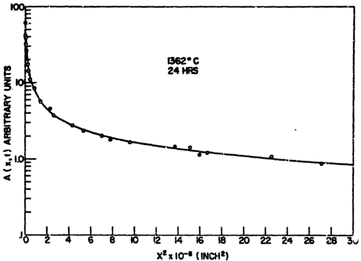
Figure 47. Portion of the Concentration Profiles for Two Polycrystalline ZrC Specimens. The Closed Circles (●) Refer to Mechanical Sectioning and the Open Circles (○) to Chemical Sectioning
