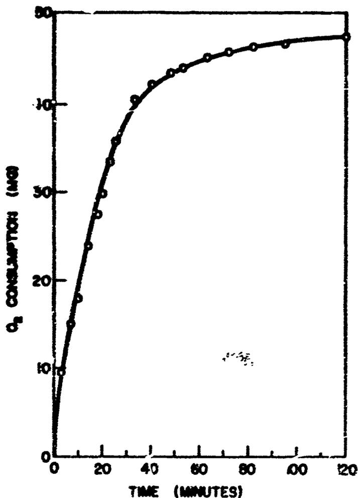
Figure 60. Oxygen Consumption Versus Time for  $Y_2O_3$  Stabilized  $ZrO_2$  Coated With  $ZrB_2$
