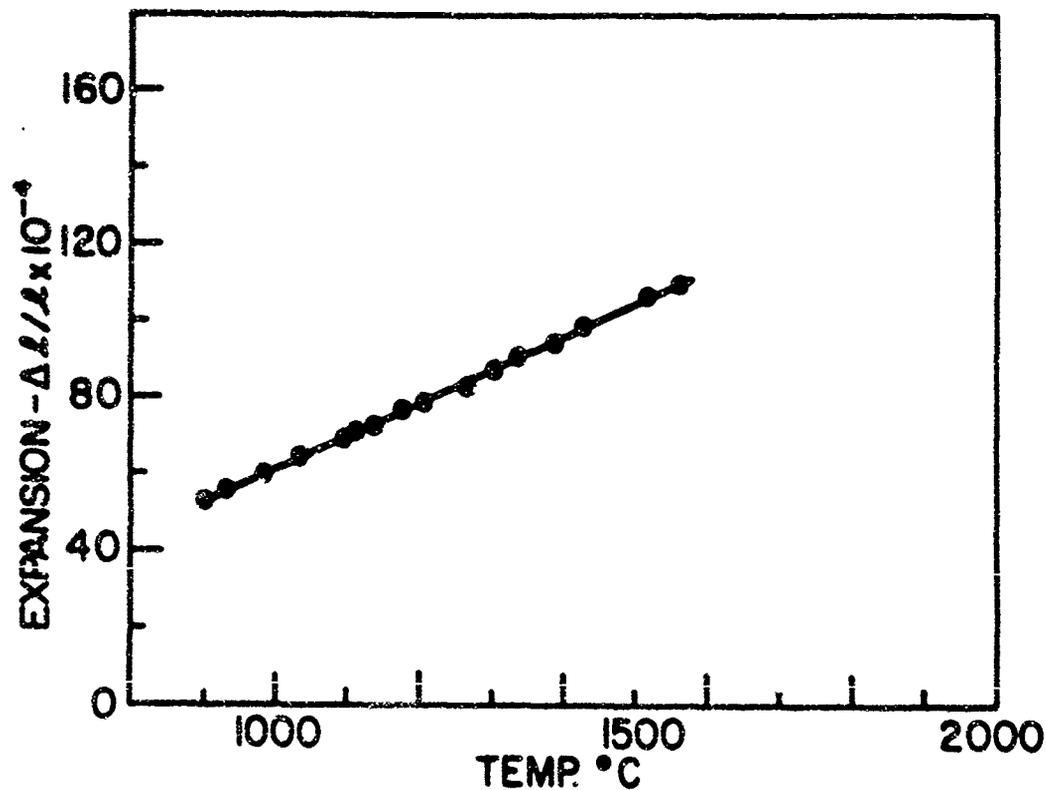
Figure 24. Thermal Expansion of  $ZrB_2$ - $YB_6$  Composite
