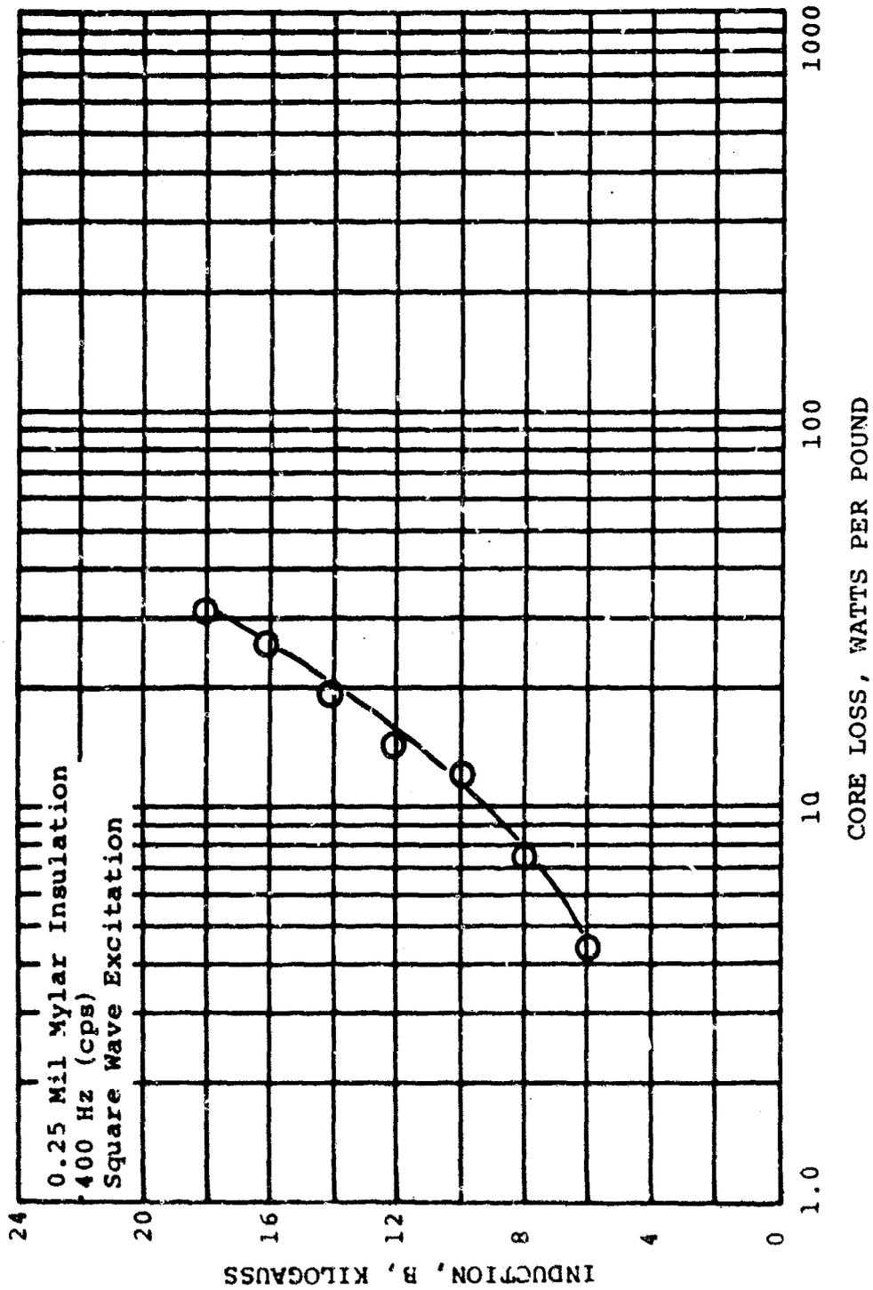
FIGURE 6. Core Loss, Pc sq., Annealed 0.008-Inch Thick Hiperco 27 Alloy
