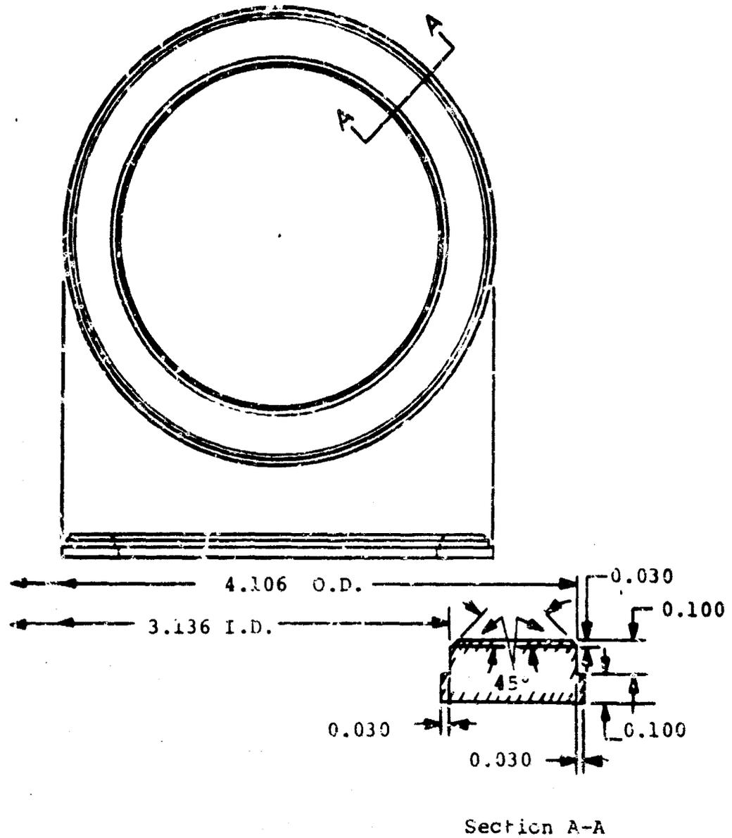
FIGURE 25. Rowland Ring Core Box Ceramic Washer - Alite A-610
