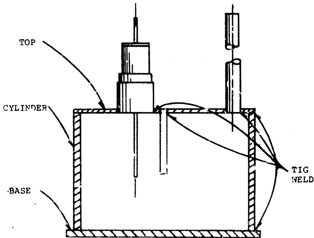
FIGURE 24. Electrical Conductor Continuous Measurement Contained
