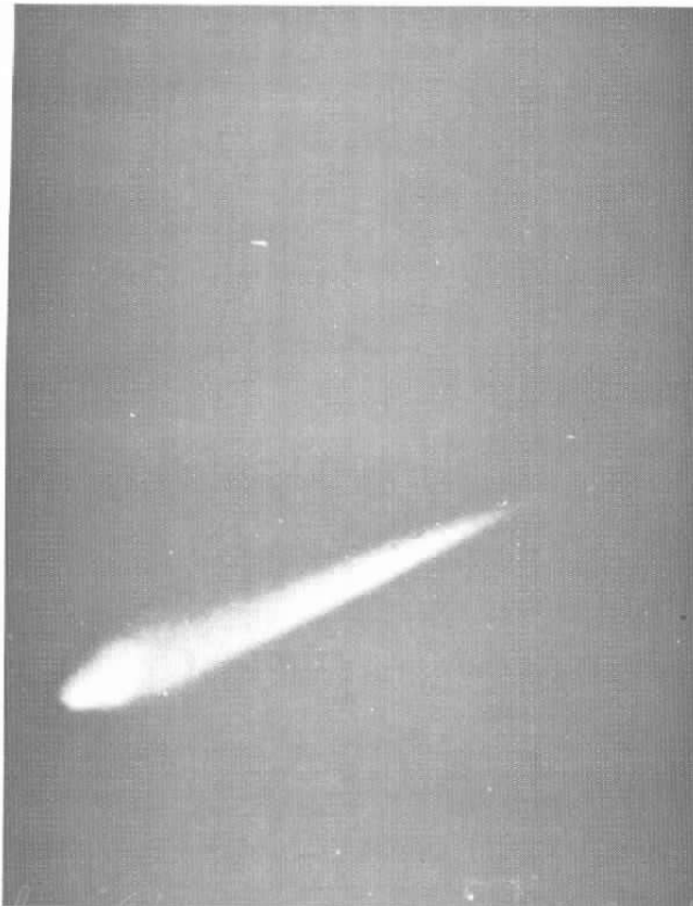
Shot K-1388 0.25-in.-diam Aluminum Sphere Model Velocity = 26,000 ft/sec Range Pressure = 9.8 mm Hg
