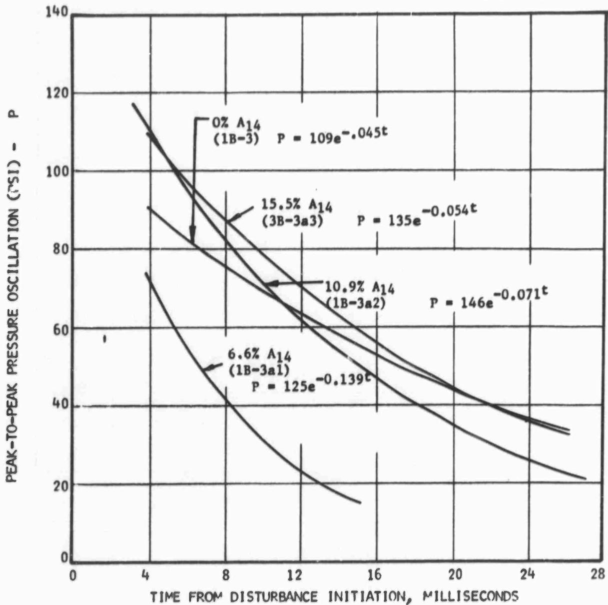
Figure 18. Damping Rate Comparison for Various Concentrations of A<sub>14</sub> Additive; 10 Grain Pulse Charge - Mixture Ratio = 3.0
