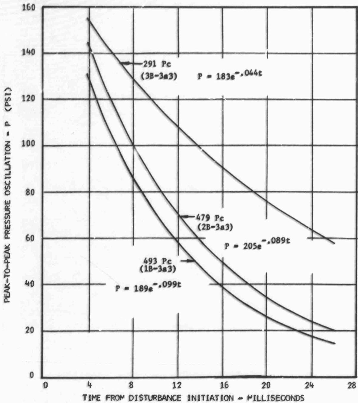
Figure 24. Effect of Chamber Pressure on Instability Damping Rate with 15.5% A<sub>14</sub> Concentration
