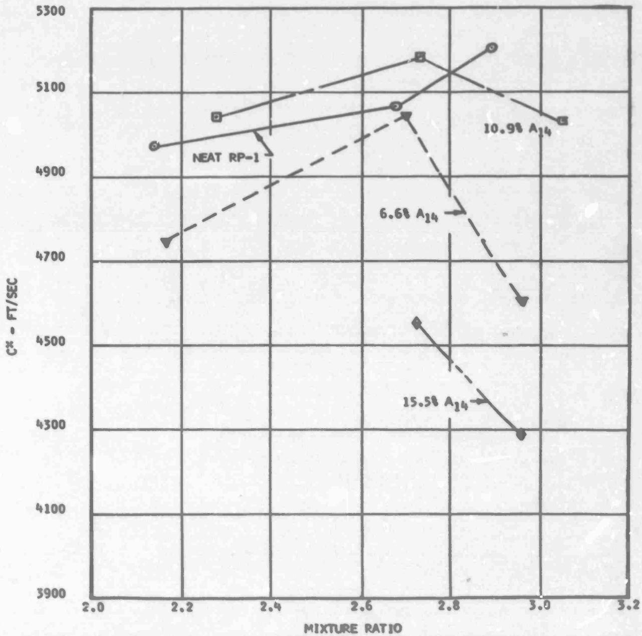
Figure 13. Experimental C\* vs Mixture Ratio for Various Concentrations of A<sub>14</sub> Additive
