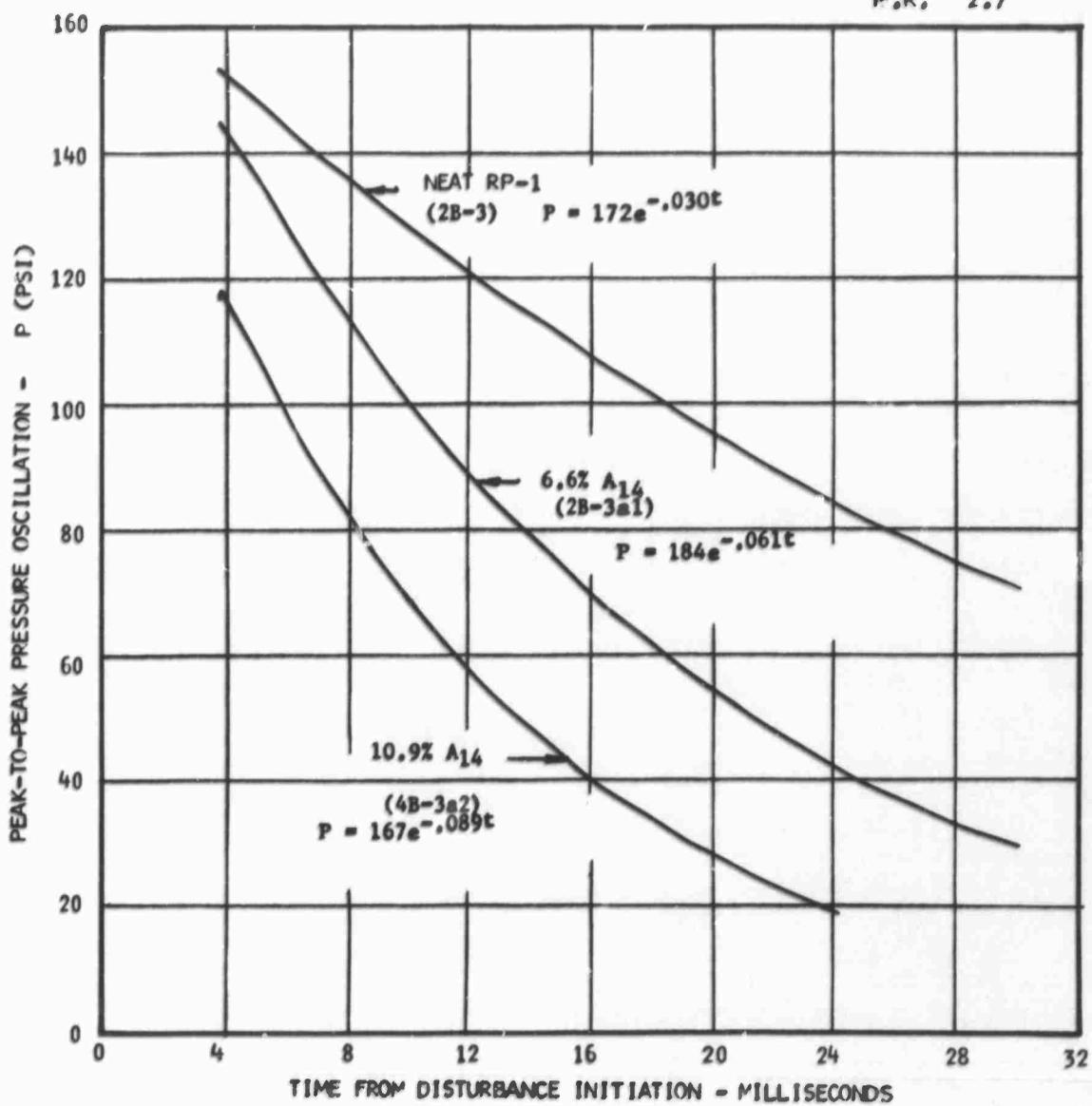
Figure 21. Damping Rate Comparison for Various Concentrations of A<sub>14</sub> Additive; 20 Grain Pulse Charge - Mixture Ratio = 2.7
