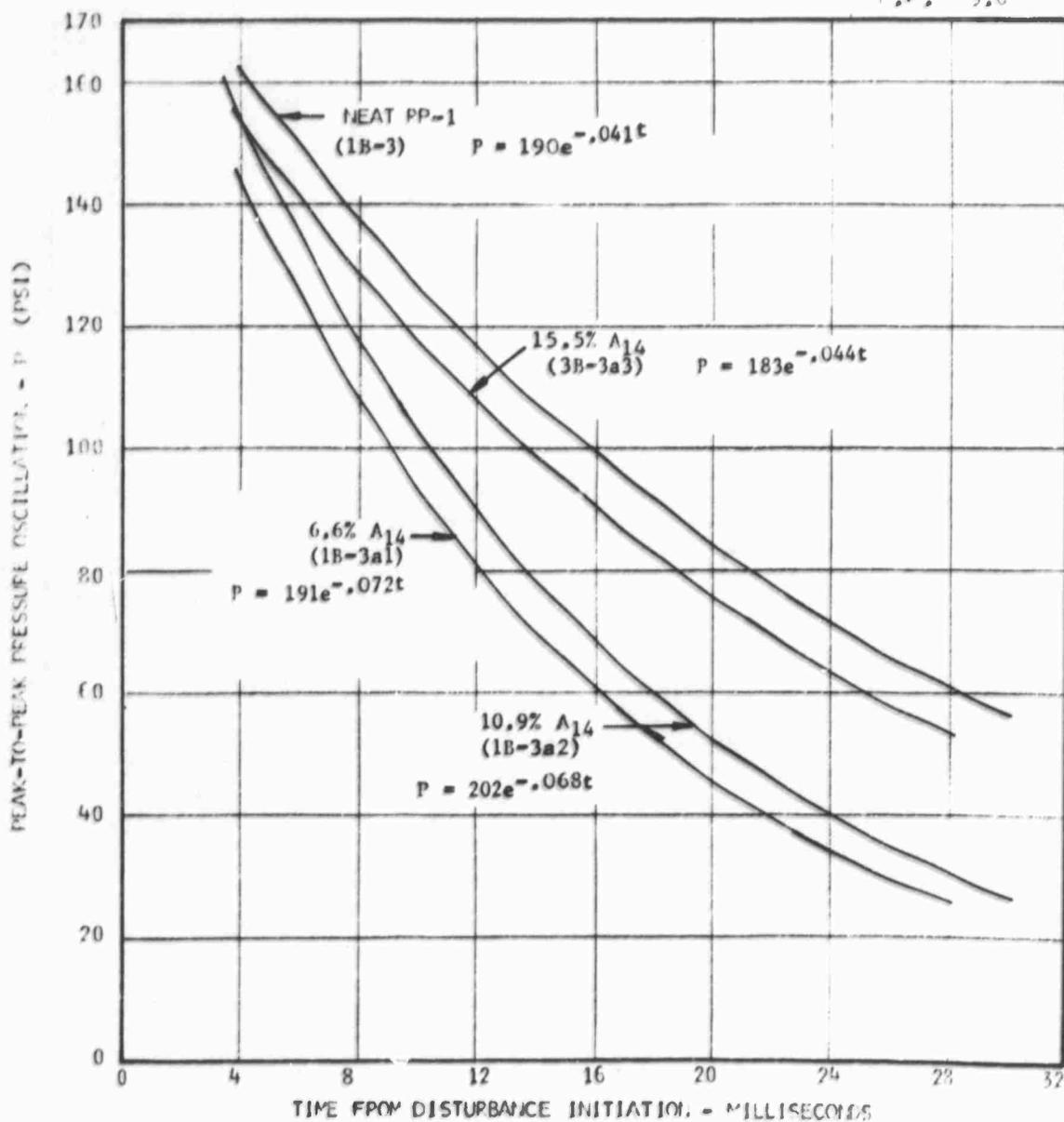
Figure 22. Damping Rate Comparison for Various Concentrations of A<sub>14</sub> Additive; 20 Grain Pulse Charge - Mixture Ratio = 3.0
