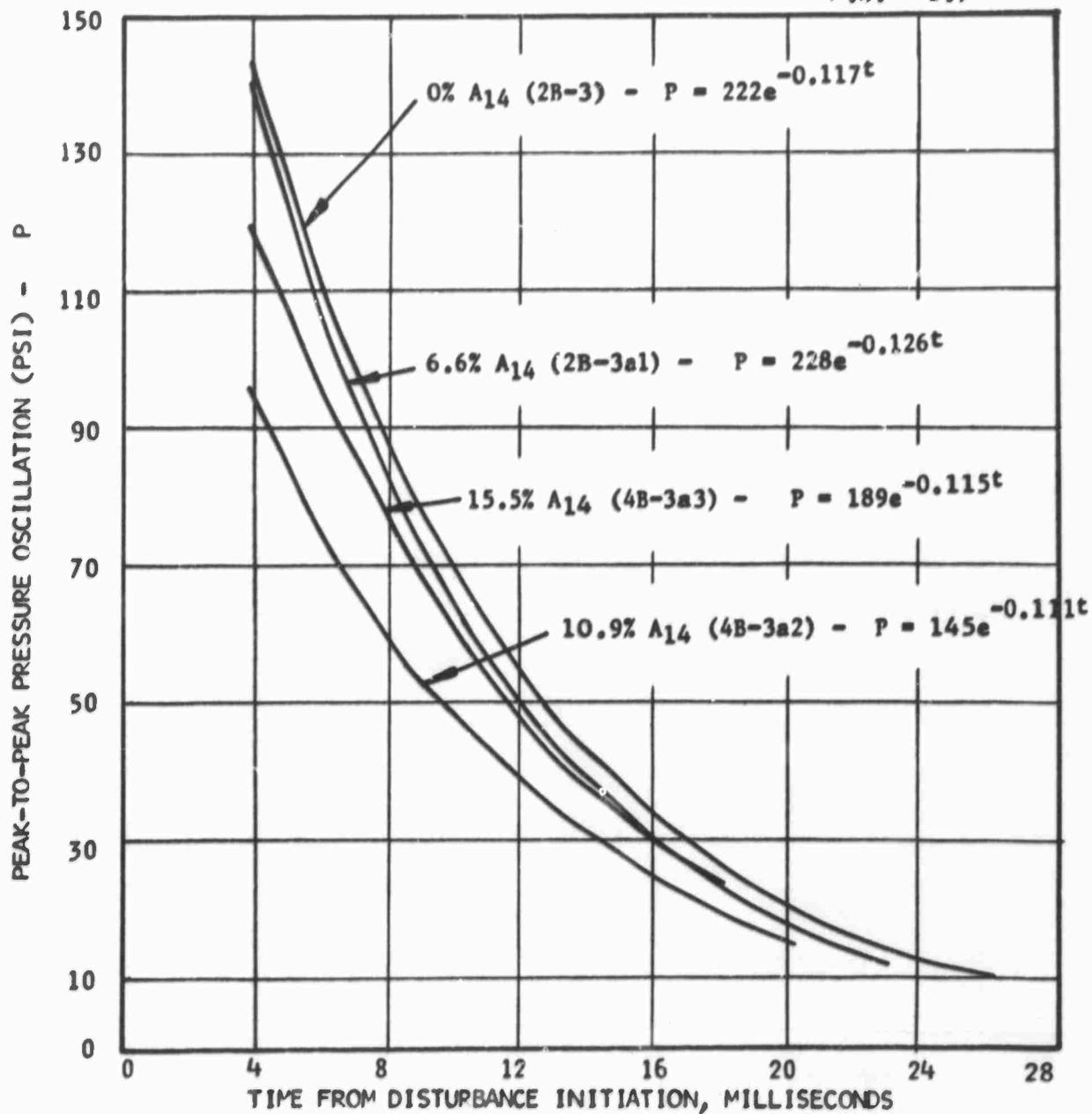
Figure 19. Damping Rate Comparison for Various Concentrations of A<sub>14</sub> Additive; 15 Grain Pulse Charge - Mixture Ratio = 2.7
