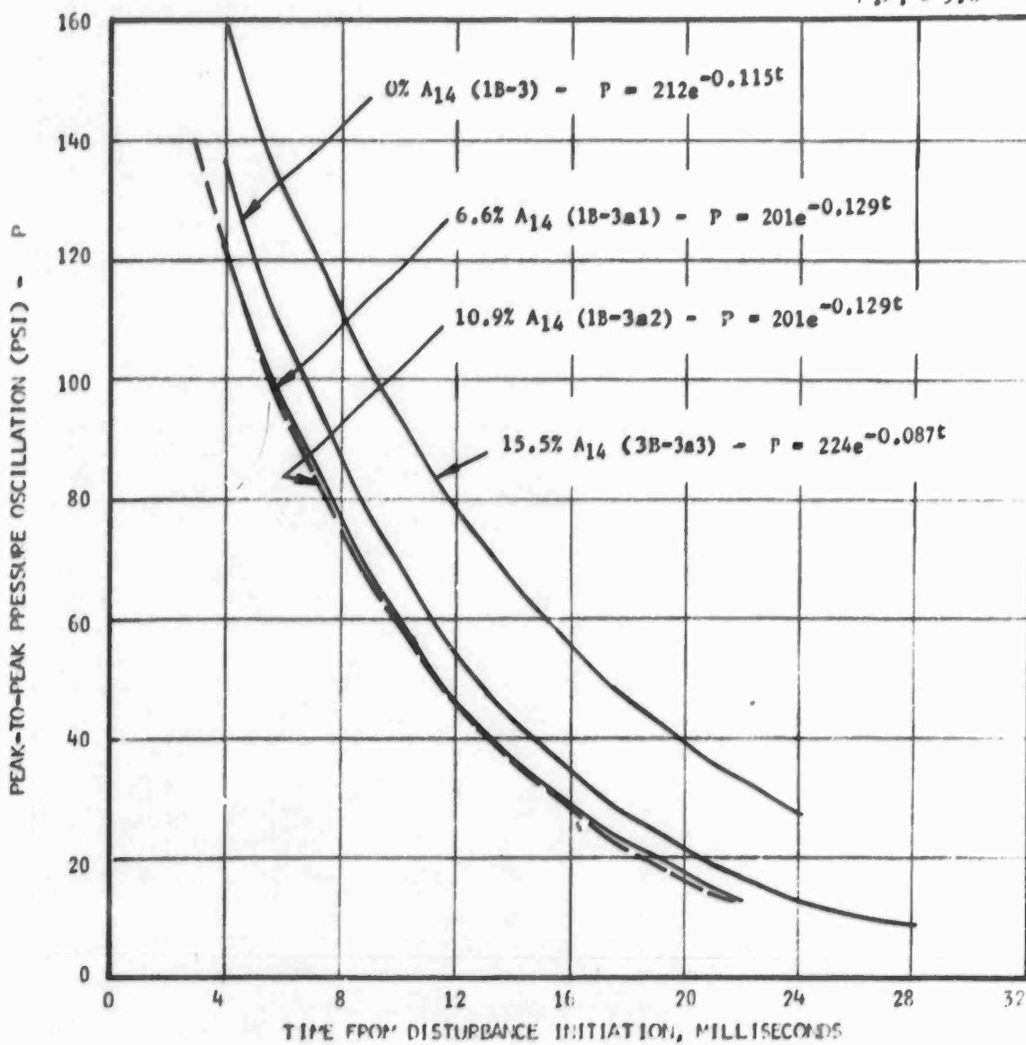
Figure 20. Damping Rate Comparison for Various Concentrations of A<sub>14</sub> Additive; 15 Grain Pulse Charge - Mixture Ratio = 3.0
