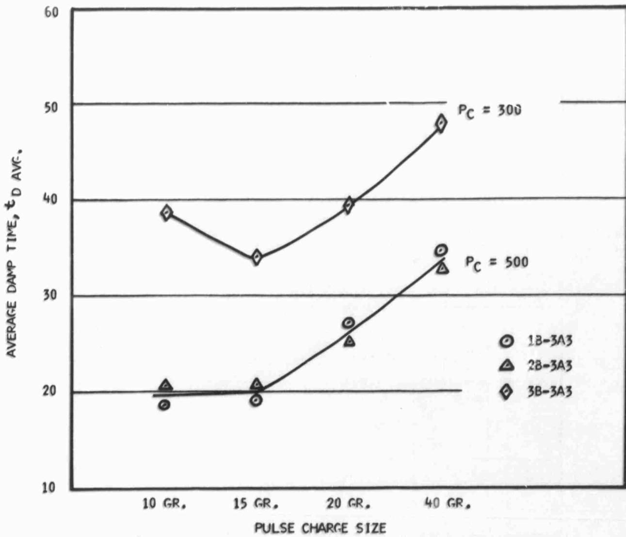
Figure 23. Influence of Chamber Pressure on Instability Damping Characteristics with 15.5%  $A_{14}$  Concentration
