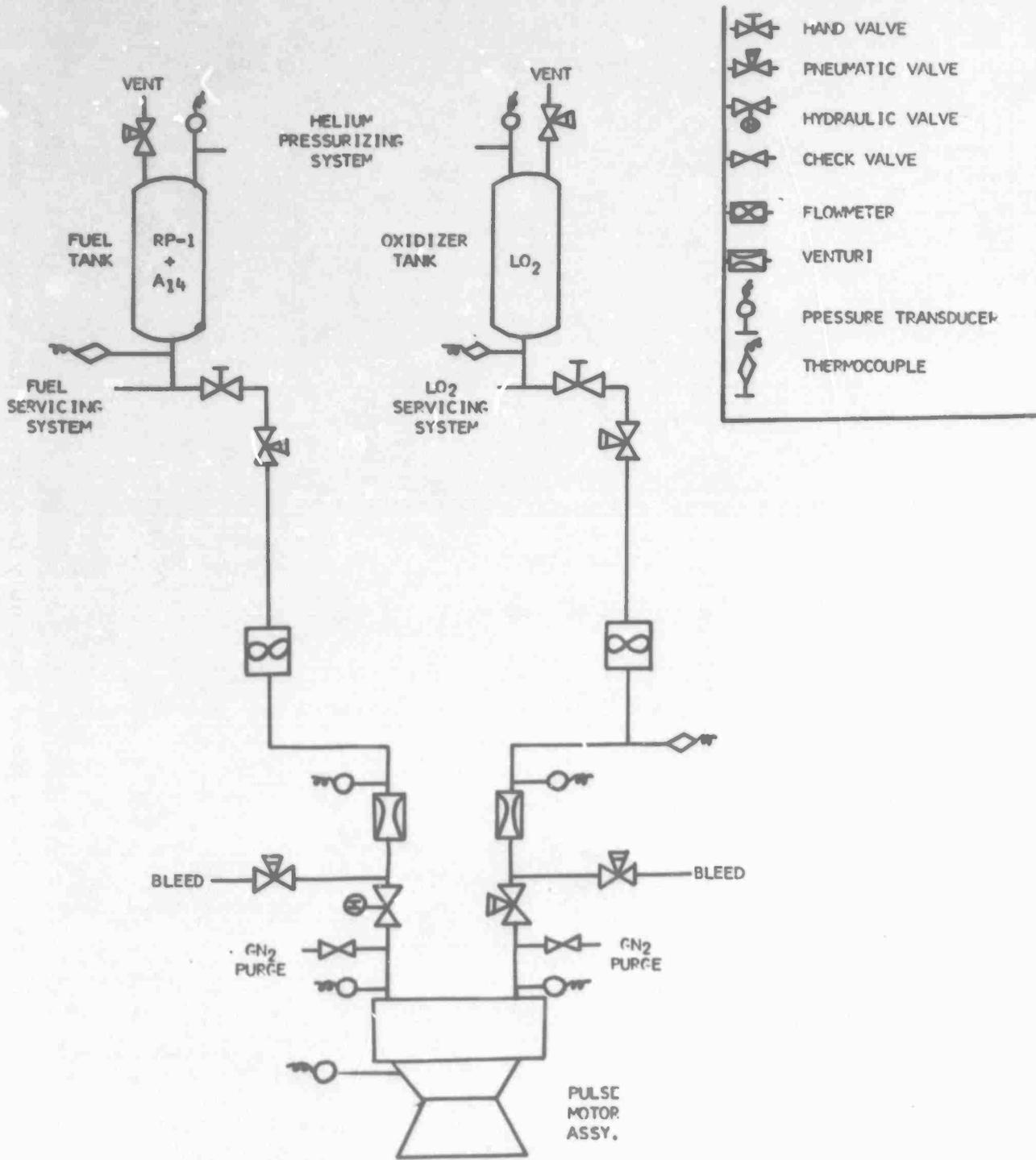
Figure 8. Test System Schematic
