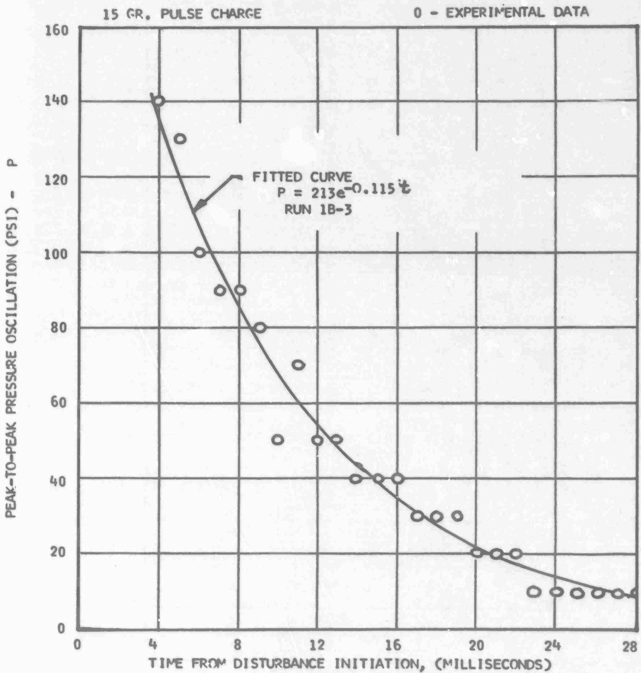
Figure 11. Typical Curve Fitted to Pressure Decay Data
