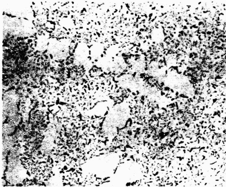
Figure 75. Ir-Os-Pt-C (65/23/5/7): Arc-Melted Alloy X500
