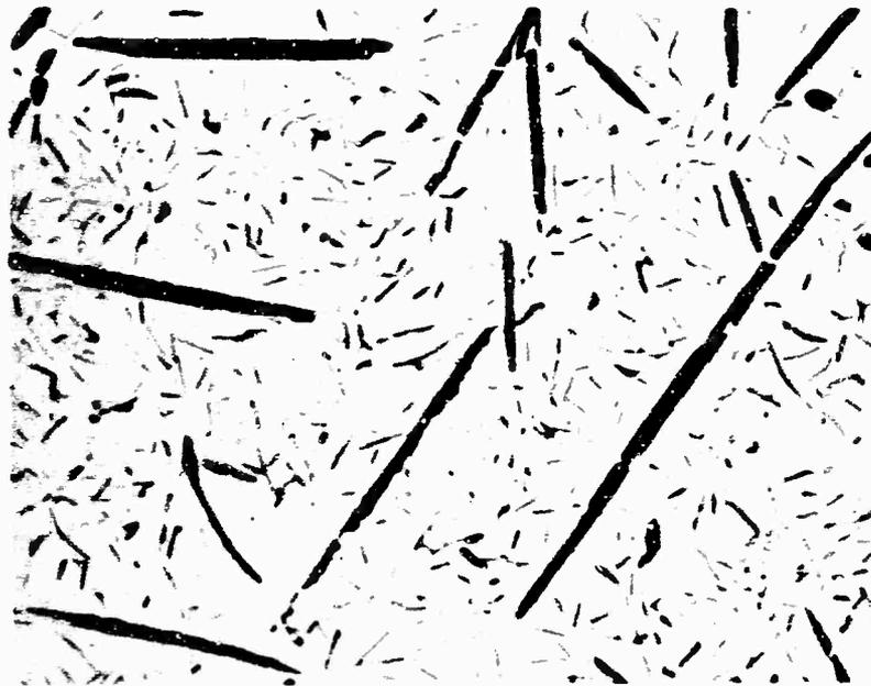
Figure 77. Ir-Os-Pt-C (55/25 5/15): Arc-Melted Alloy Showing X400 Primary Graphite in a Metal Carbon Eutectic.
