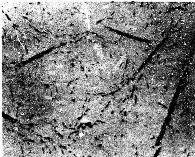
Figure 69. Ir-Pt-C (71/18/11): Alloy Cooled in the DTA
