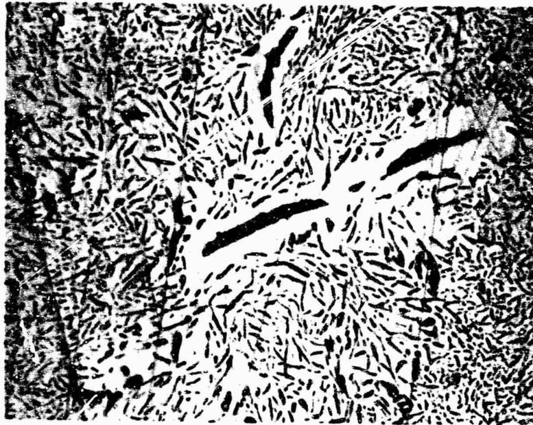
Figure 55. Rh-C (83/17), Arc-Melted Alloy Showing Primary Graphite in a Eutectic Matrix.
