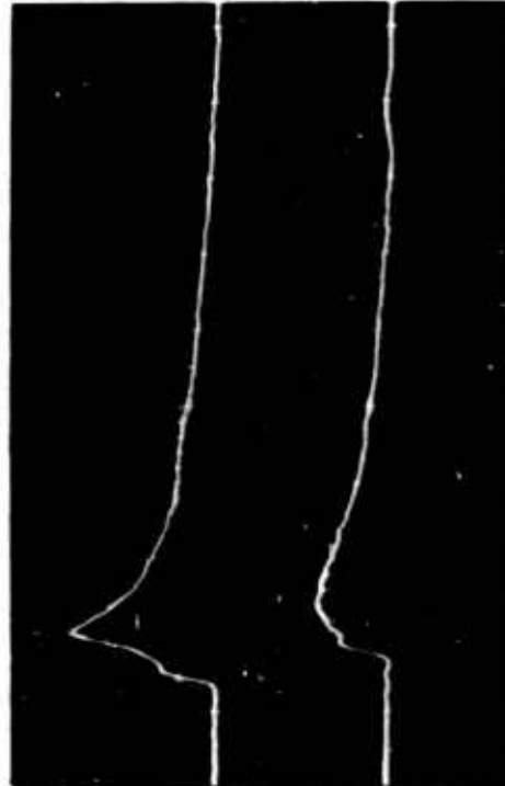
d. An 80 duPM/20K Charge Examples of Pulse Gun Blast Waves From Slower Burning duPont Military 3031 Powder
