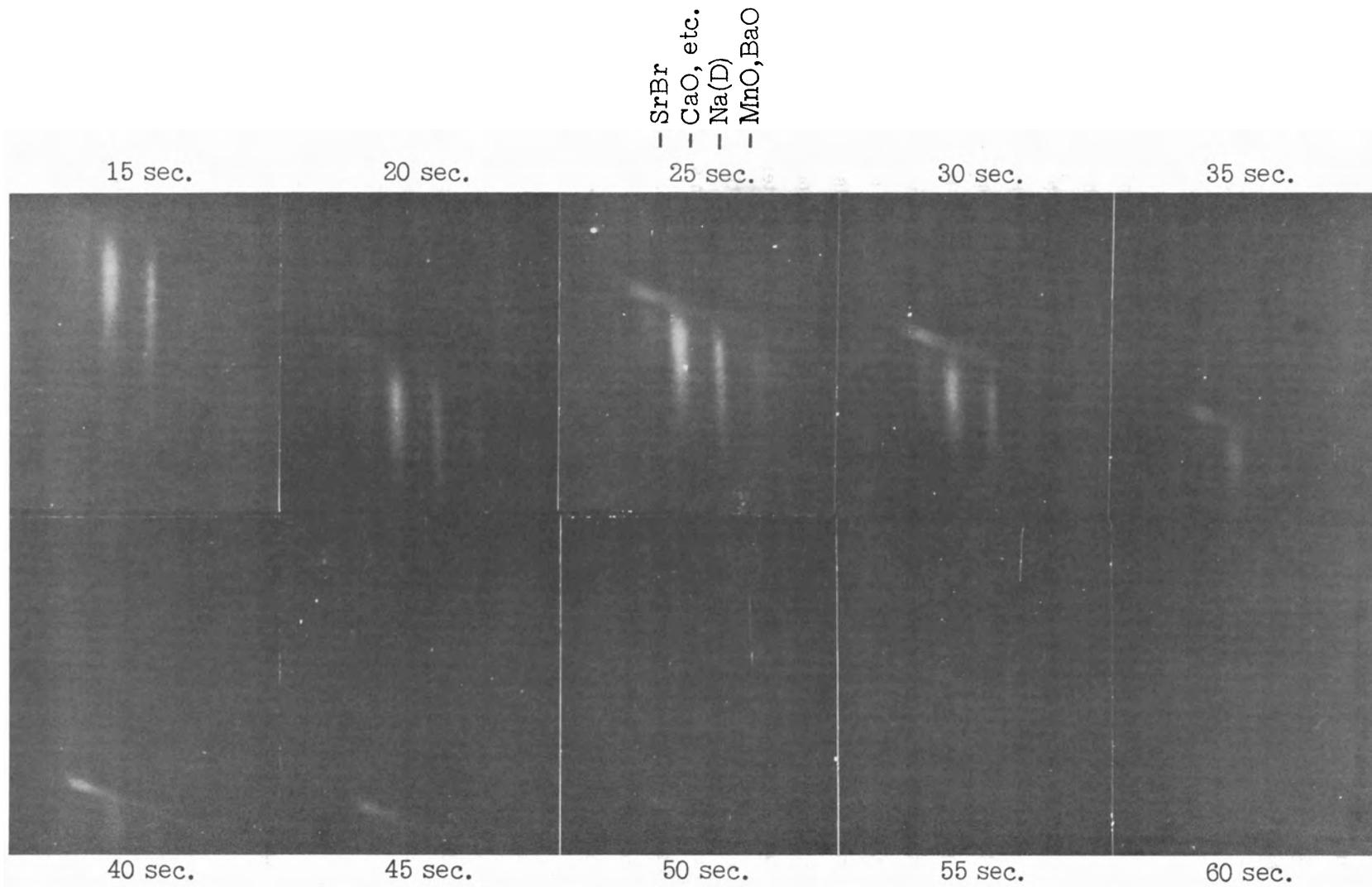
Plate 6. Slitless Spectrograms V2 Jet Without Added Substances
