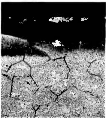
FIGURE 23. \alpha + COMPOUND Ti_2Cu . CONDITION PRIOR TO EUTECTOID DECOMPOSITION WAS EQUIAXED \alpha + \beta . (Ti-6Al-3Cu; 1560 F - 4 HOURS - AC, 1020 F - 24 HOURS - AC.)*
