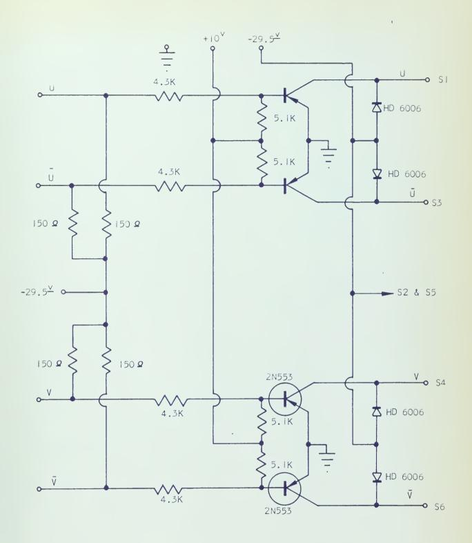
Figure 3 Power Gate Isolation for Logic Circuit
