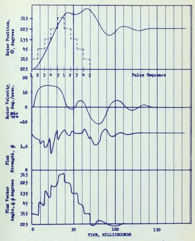
Figure 13 Size 11 Notor response to 5 fwd.-5 rev. pulse train showing failure profile.
