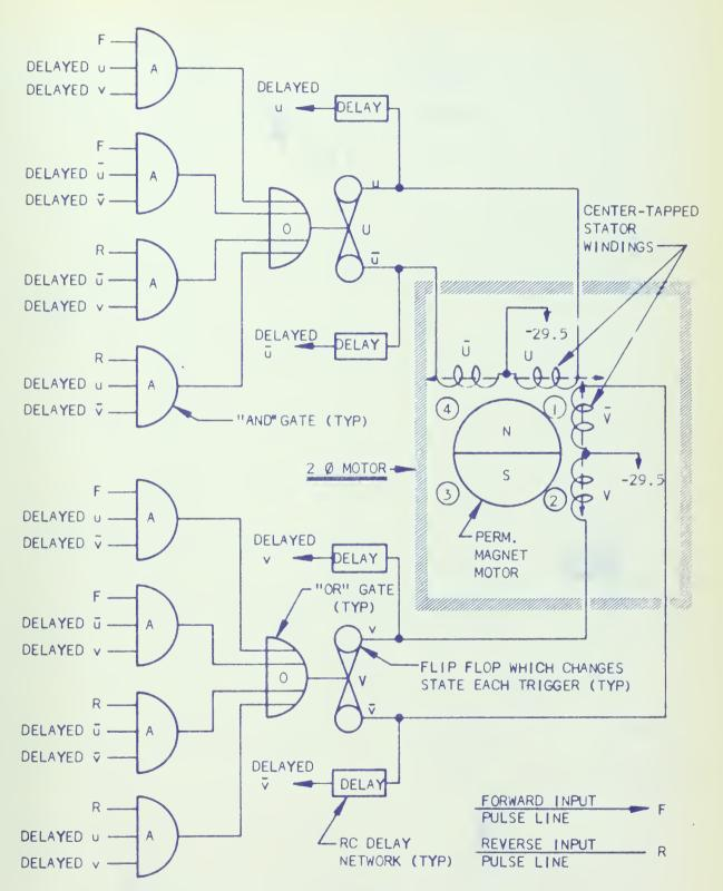
Figure 2 Stepper Motor Drive Logic Diagram
