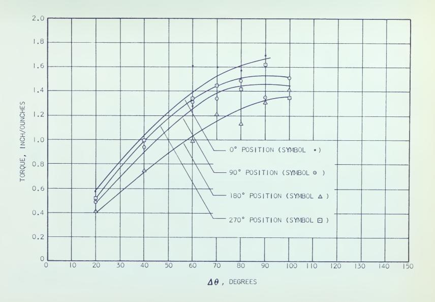
Figure 6 Static Torque Tests of Size 11 Stepper Motor with -29.5 volts on Stator
