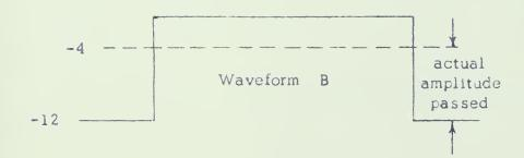
This is directly coupled to the "or" gate. The "or" gate operates such that the cathode nodes of the "or" gate diodes assume the most positive potential of the four available. Since the cathodes of the "or" gate diodes are all held at -12 volts, as soon as the plate of any "or" gate diode begins to rise above -12 volts that diode will conduct. Hence, in the case of the FUV "and" gate passing the B waveform, the topmost diode of the Q3 "or" gate in Fig. 1 will conduct and faithfully pass the
