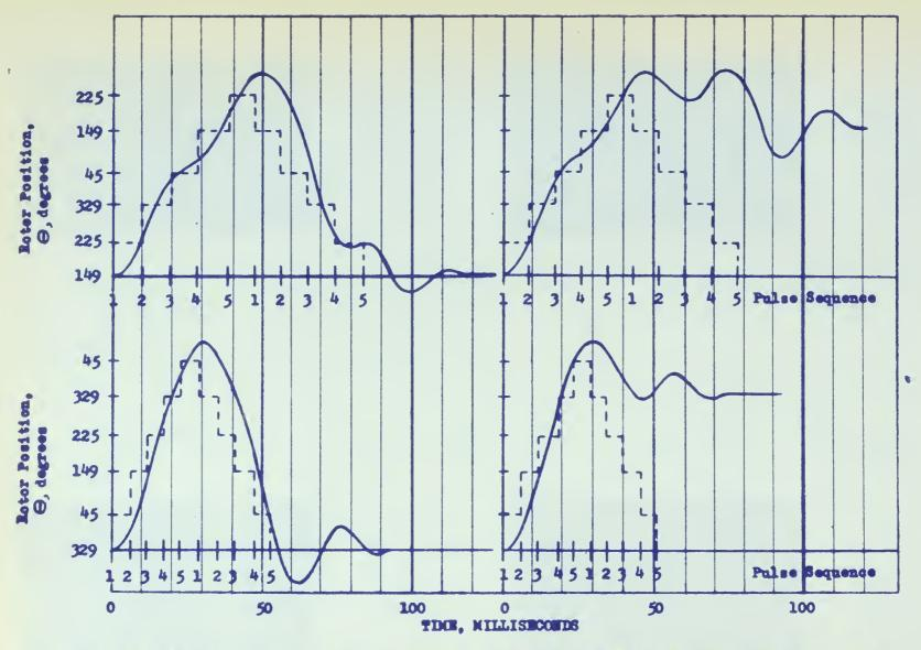
Figure 17 Size 8 Notor responses to 5 fwd.-5 rev. program showing Rotor Position: Top Left: just before anomalous failure; Top Right: at anomalous failure; Bottom Left: just before "normal" failure; Bottom Right: at "normal" failure.
