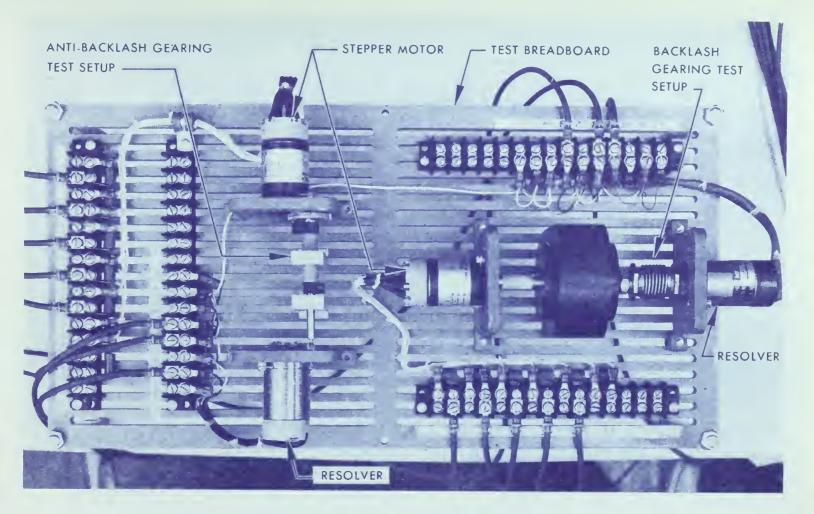
Illus. 3 Test Breadboard No. 1 Showing Gear Trains with and without Anti-Backlash Gearing
