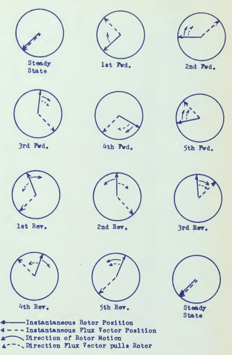
Figure 15 Size 11 Motor Rotor and Resolved Flux Vector Positions for 5 fwd.5 rev. program failure.
