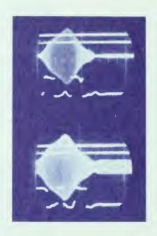
Photo. 11 Response to 5-Forward-Pulse, 5-Reverse-Pulse Train Showing Large Back EMF Hump in  $\overline{U}$  State (top) and Change in  $\overline{U}$  Logic State as a Result of Back EMF (bottom). At 76 p.p.s., 00~ms/cm.
