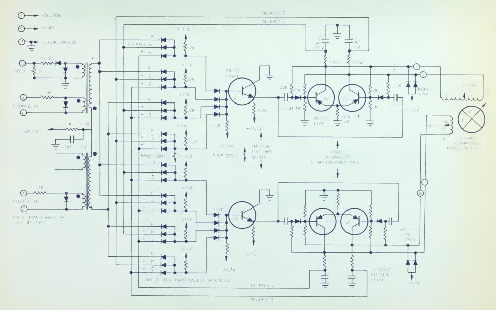
Figure 1 stepper Motor Drice Logic Circuit schematic
