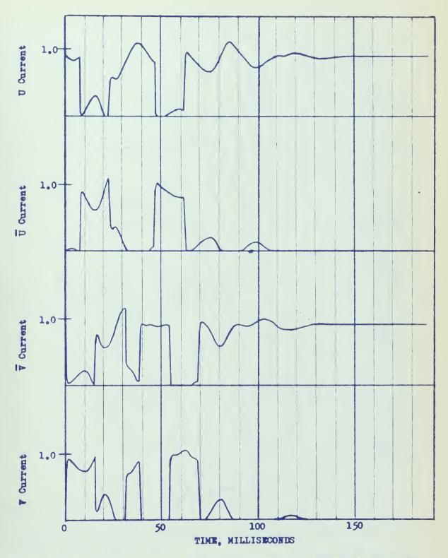
Figure 14 Size 11 Motor response to 5 fwd.-5 rev. pulse train showing all currents at failure.
