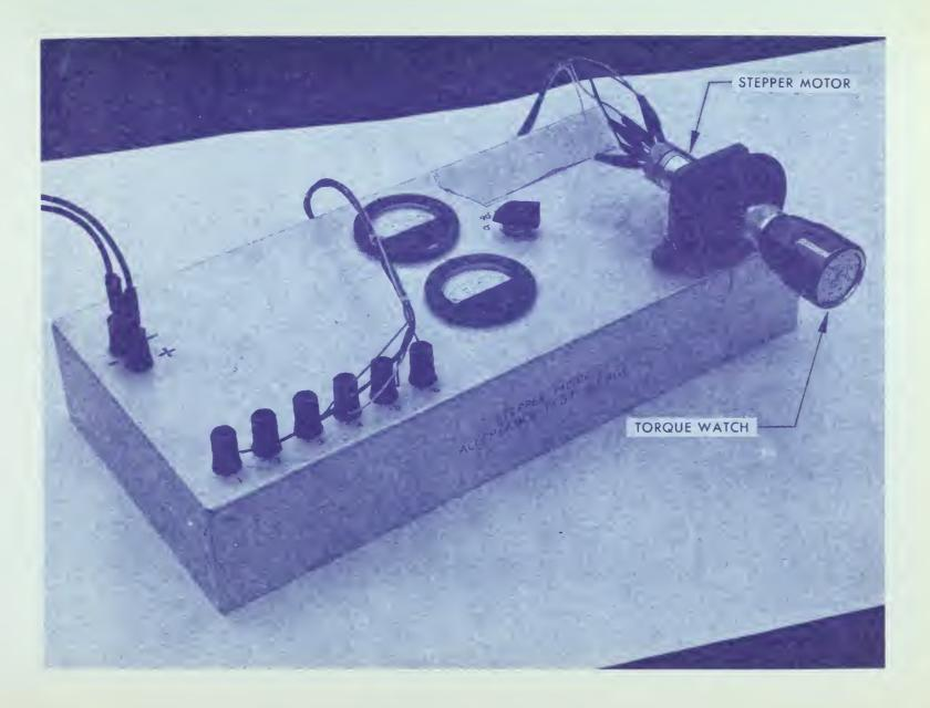
Illus. 7 Stepper Motor Acceptance Test Kluge for Static Torque Testing
