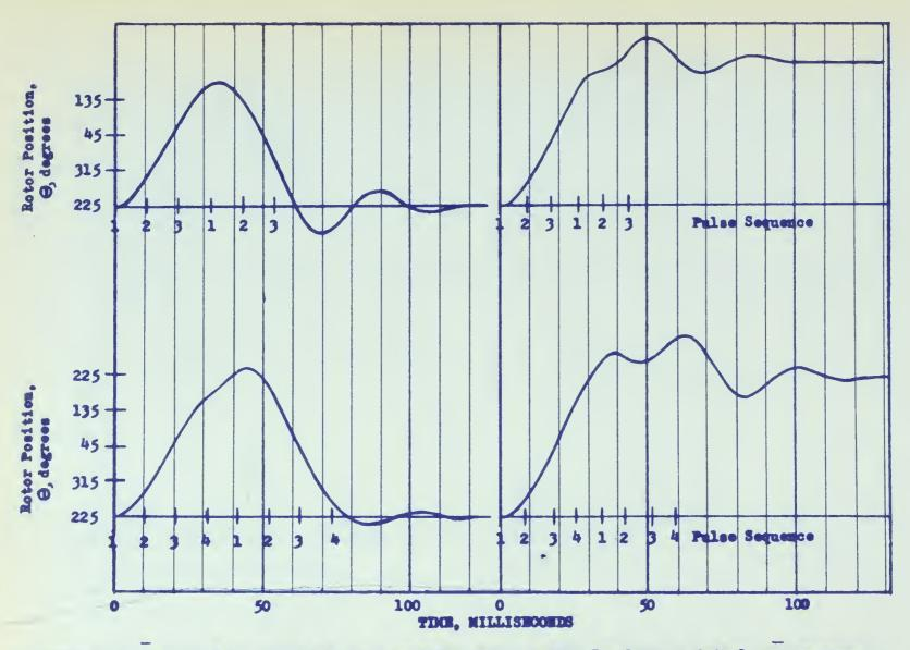
Figure 16 Size 11 Notor responses showing Rotor Position for: Top Left: 3 fvd.-3 rev. program just before failure; Top Right: 3 fvd.-3 rev. program at failure; Bottom Left: 4 fvd.-4 rev. program just before failure; Bottom Right: 4 fvd.-4 rev. program at failure.
