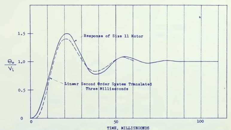
Figure 7 Comparison of Transient Response to a Step Input of the Size Il Motor and a Theoretical Linear Second Order System ( J= 0.27,  $\omega_{m}=188.1$  radians/sec.)
