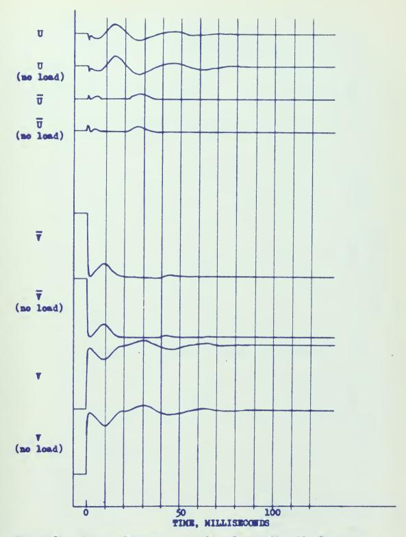
Figure 8A Ourrent Responses to a Step Input, Sixe 11, Showing Comparison of No Load Currents and Currents with Load of Resolver and Anti-Backlash Gear Train (70.6:1)
