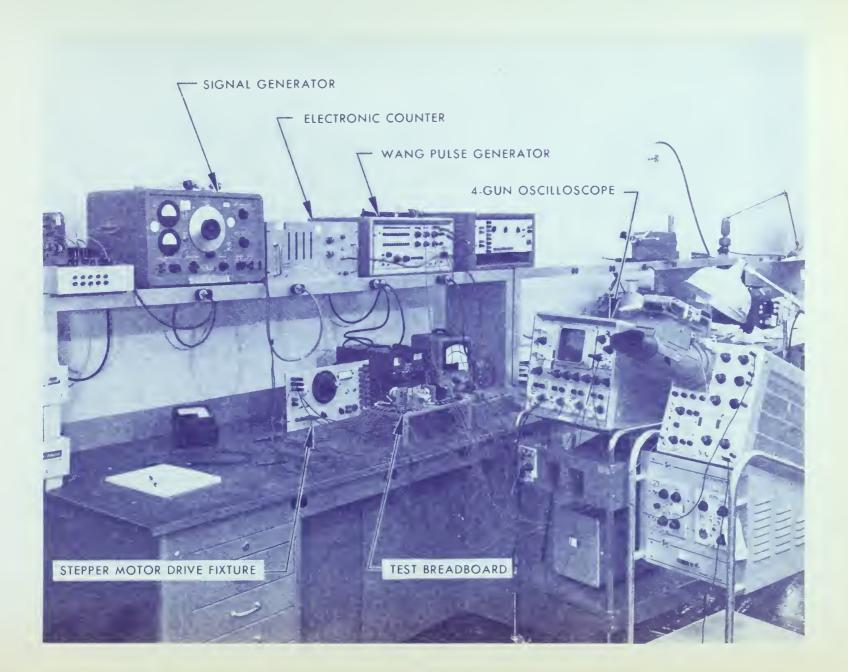
Illus. 2 General Arrangement of Stepper Motor Test Equipment and Testing Area
