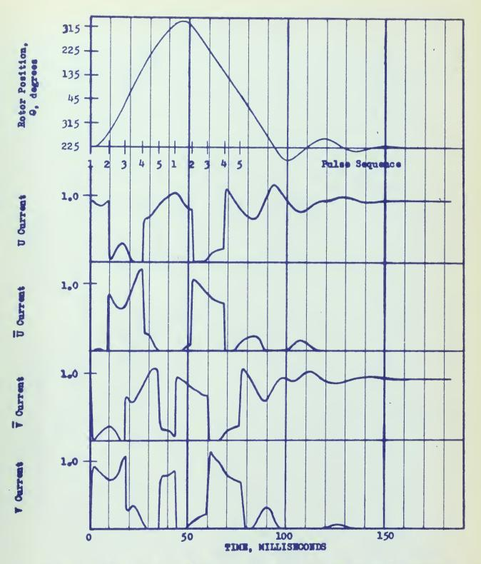
Figure 12 Size 11 Notor Response to 5 fwd.-5 rev. pulse train, showing (top to bottom ) Rotor Position and each current just prior to motor failure.
