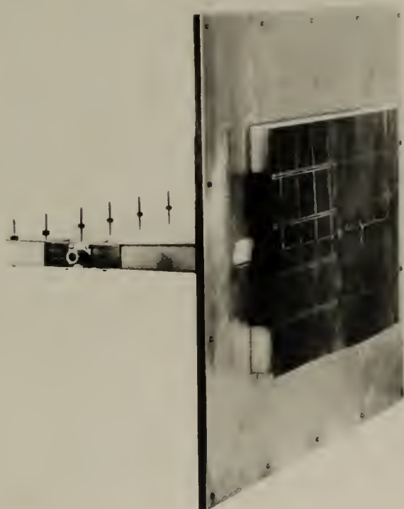
Figure 64. Forty Element Coplanar Array
