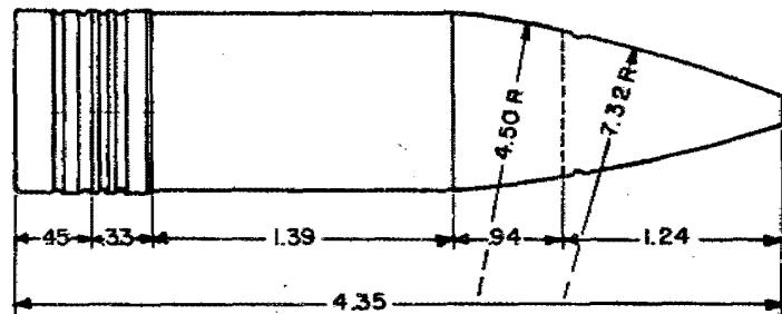
PROJECTILE, ILLUMINATING, 3-INCH, MARK 25; DUMMY NOSE PLUG
