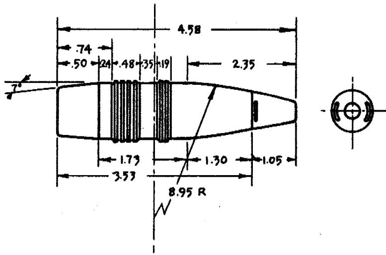
SHELL, H.E., 90MM, T15; FUZE, DUMMY, M44A2
