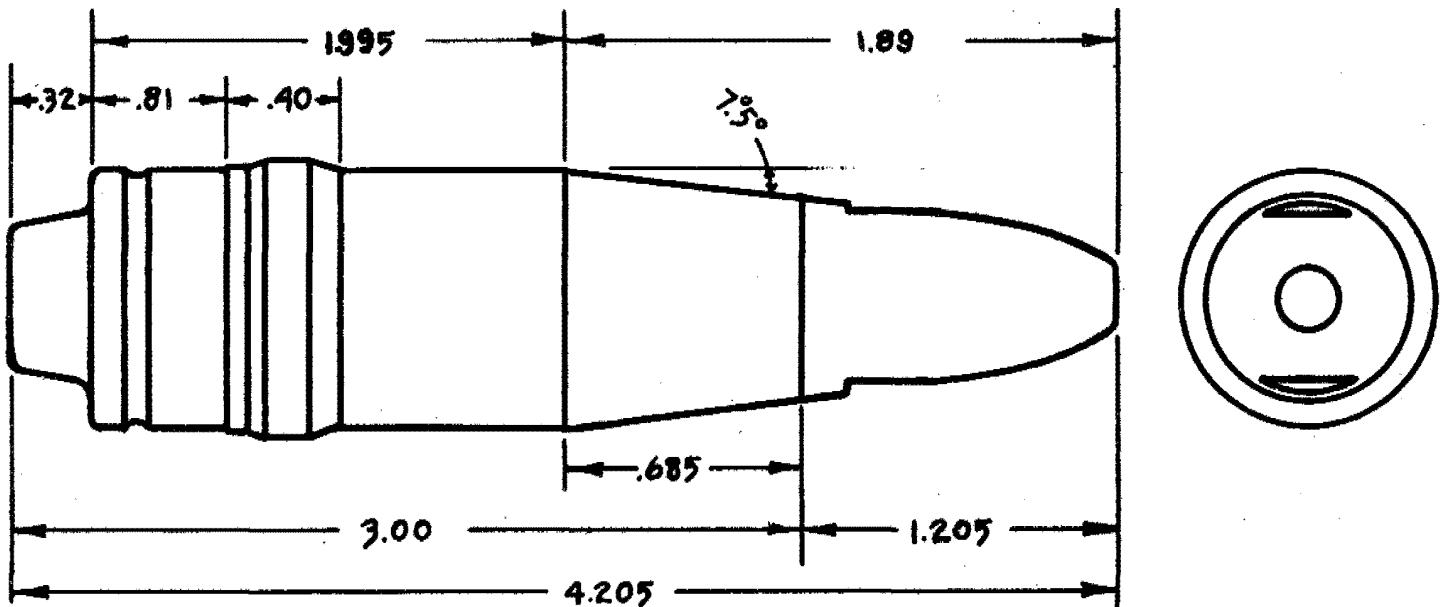
SHELL, H.E., 40MM, T7; FUZE, DETONATING, MARK 27
