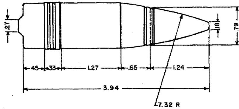
PROJECTILE, 3-INCH, MARK 27; DUMMY NOSE PLUG
