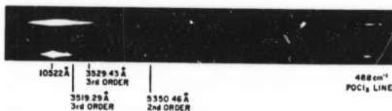
Fig. 12. Spectra of mode-locked Nd:POCl 3 liquid laser. Two shots show \approx 100 \text{ cm}^{-1} central band and Raman shifted light.
