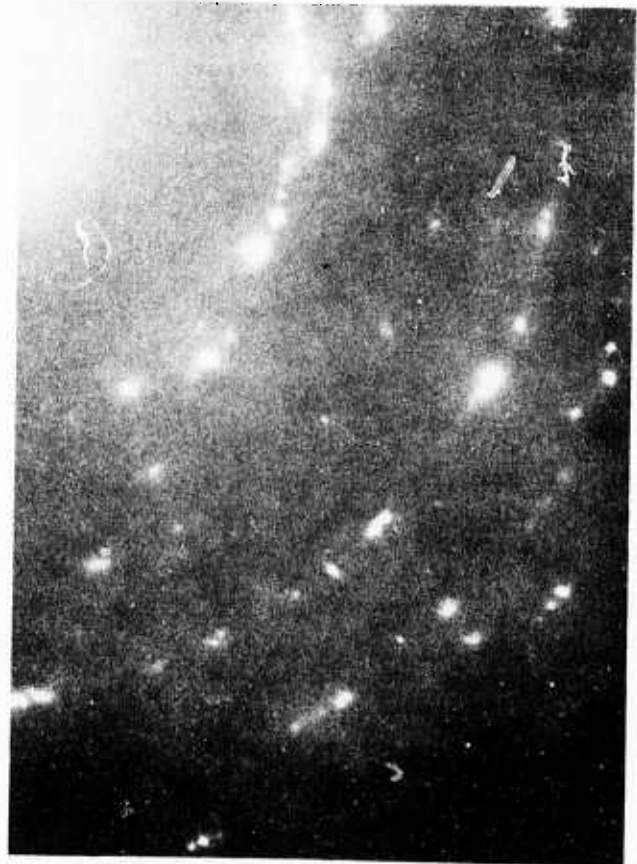
c) Electron Diffraction Pattern. Both Cu and Mo Rings are Visible.
