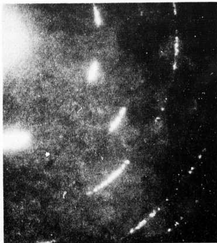
a) Note that the Layered Structure is no Longer Present. Mo Spheres are Approximately 860 Å in Diameter. 51,000X
