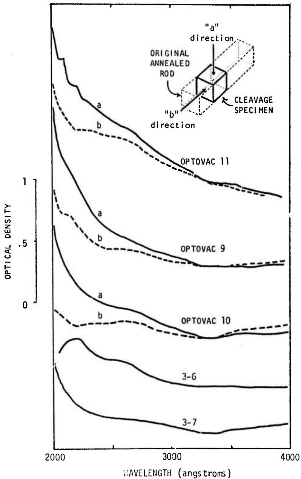
FIGURE a.2.1 Ultraviolet Absorption of KBr Specimens
