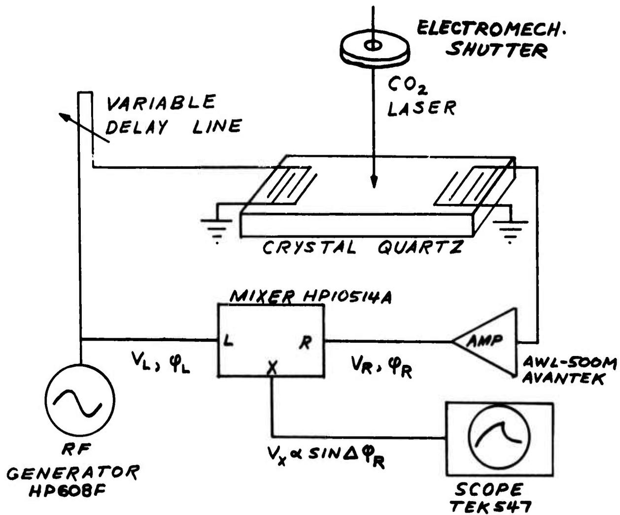
Figure 1 Experimental apparatus used to measure induced phase shifts.
