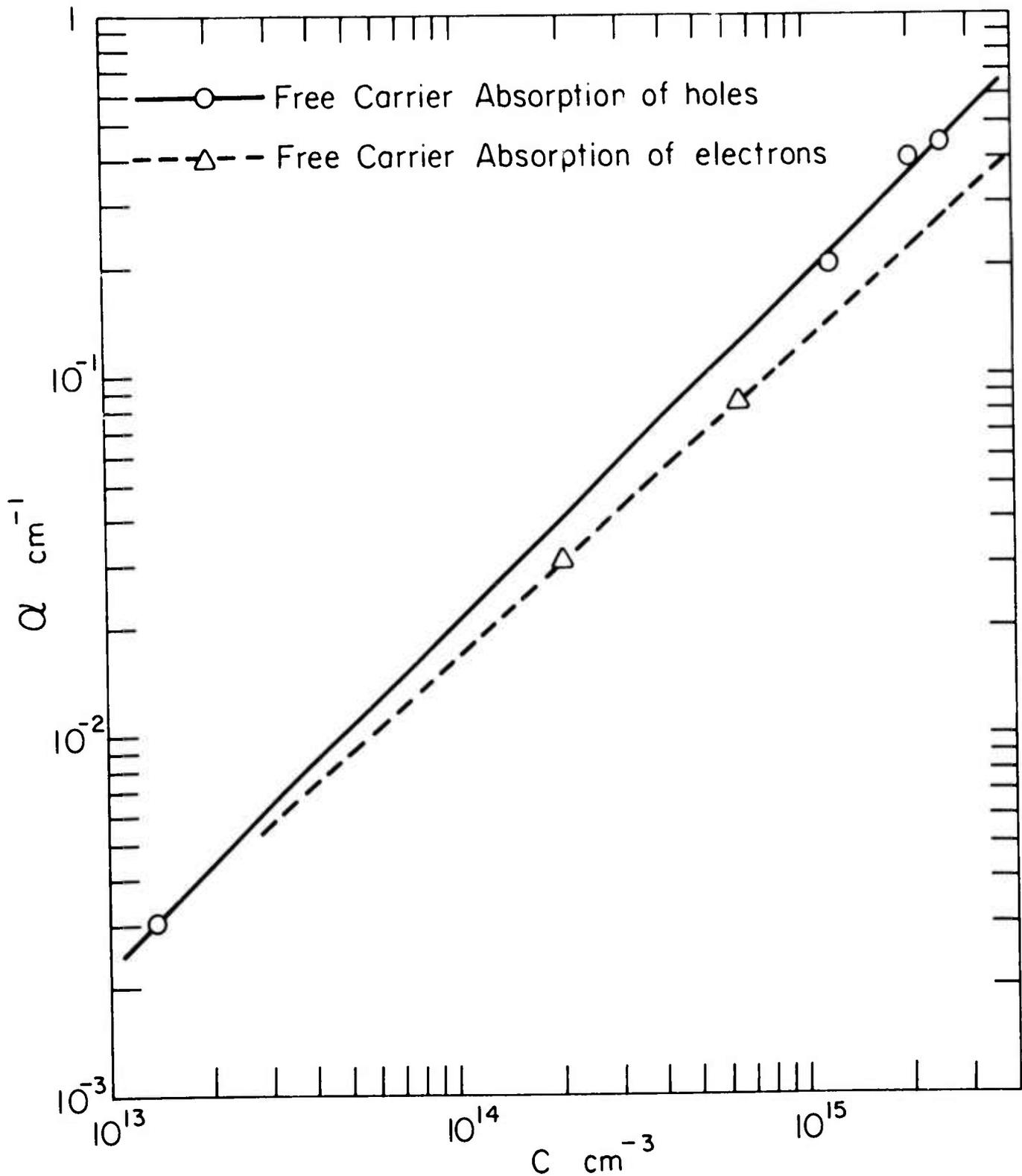
Figure 3: Absorption coefficient of CdTe +  $5 \times 10^{16} \text{Cl cm}^{-3}$  at  $10.6 \mu\text{m}$  determined by calorimetry as function of carrier concentration (electrons or holes) determined from Hall measurements at room temperature for crystals cooled from  $700^\circ\text{C}$ .
