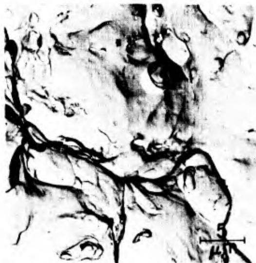
(b) Replica electron fractograph of crack extension at the plate midthickness after heat-tinting
