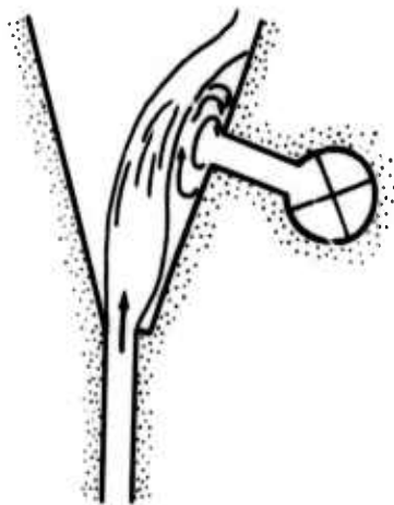
Control Port Initially Closed
