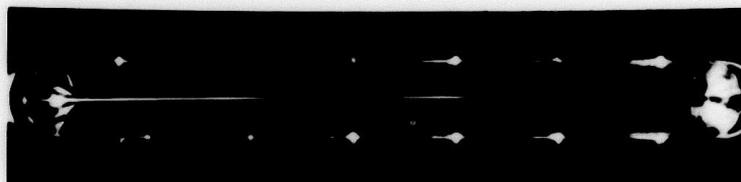
b. DIFFUSE DISCHARGE,  $p = 5.0$  atm,  $X_{N_2} = 0.07$ ,  $X_{He} = 0.93$ ,  $I_o = 6.0 \times 10^8$  W/cm<sup>2</sup>
