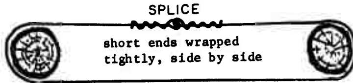
Sketch A-3.1. Assembly of Wire Loops.
