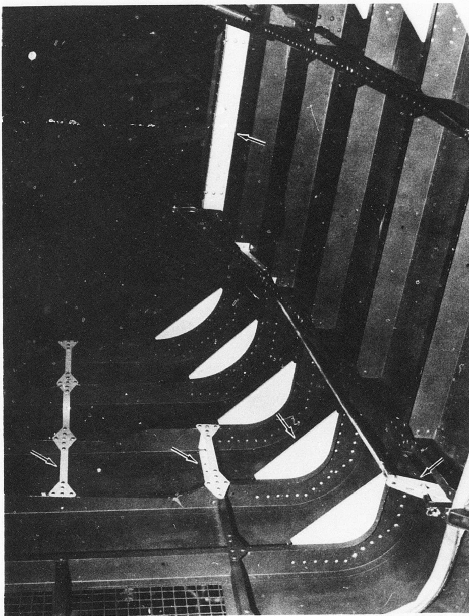
Figure 22. Main Rotor Pylon, Redesign.
