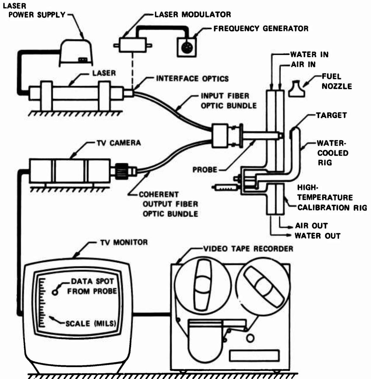
Figure 31. High-Temperature Demonstration Tests.
