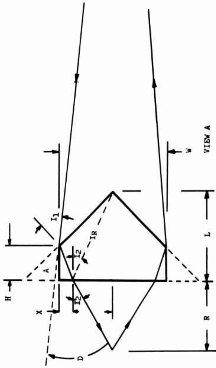
Figure D-1. Ray Trace Diagram For Three-Lens Probe.
