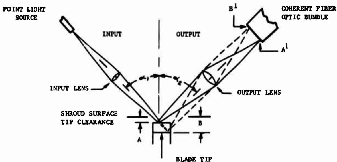
INPUT LIGHT IS FOCUSED THROUGH INPUT LENS ONTO THE BLADE TIP. LIGHT REFLECTED FROM THE BLADE TIP IS FOCUSED THROUGH THE OUTPUT LENS AND IS INCIDENT ON THE COHERENT FIBER OPTIC BUNDLE. AS THE BLADE TIP MOVES FROM POSITION A TO POSITION B (REPRESENTING AN INCREASE IN TIP CLEARANCE), THE FOCUSED OUTPUT BEAM MOVES FROM POSITION A<sup>1</sup> TO POSITION B<sup>1</sup>. THIS CHANGE IS THEN RECORDED AS REPRESENTING THE CHANGE IN TIP CLEARANCE.
