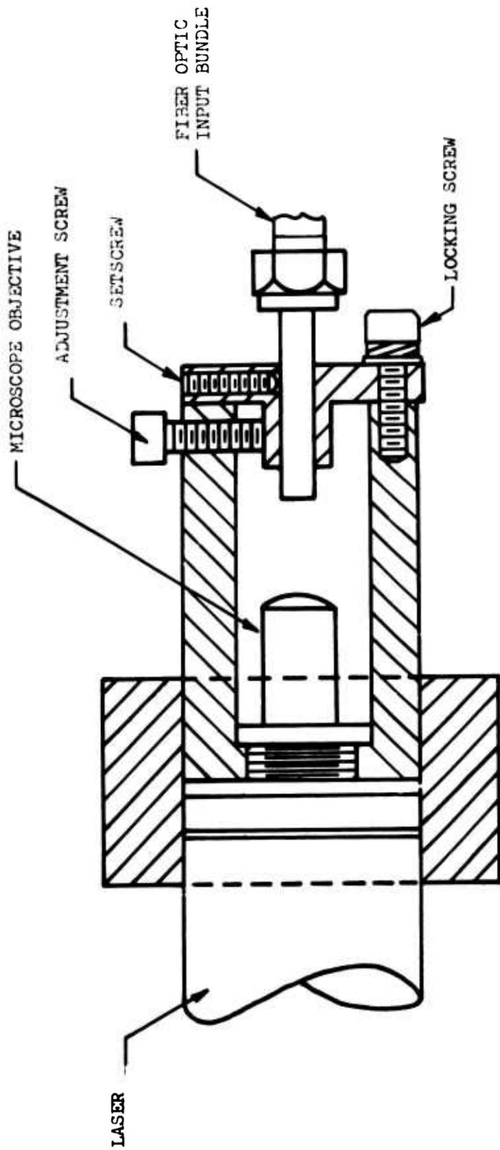
Figure 10. MTCMD Input Light System.
