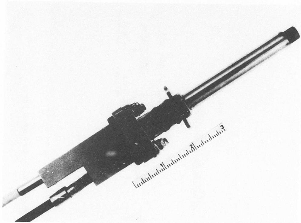
Figure 21. Three-Lens Probe.
