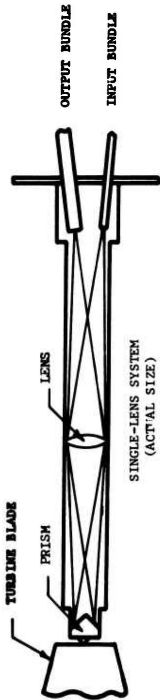
THE PRISM "FOLDS" THE BASIC TRIANGULATION SYSTEM. THE SINGLE LENS PERFORMS THE FUNCTIONS OF THE SEPARATE LENSES OF THE BASIC TRIANGULATION SYSTEM.
