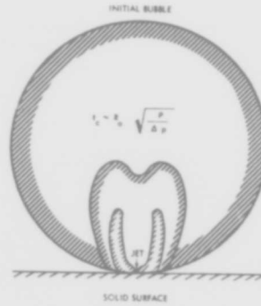
FIGURE 4-7 - COLLAPSE OF BUBBLE IN THE NEIGHBORHOOD OF A SOLID BOUNDARY (PLESSET AND CHAPMAN (56))
