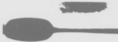
FIGURE 4-8a - "STEADY" CAVITY BEHIND A DISK. EXPOSURE TIME 2 SECONDS (EISENBERG AND POND (58))
