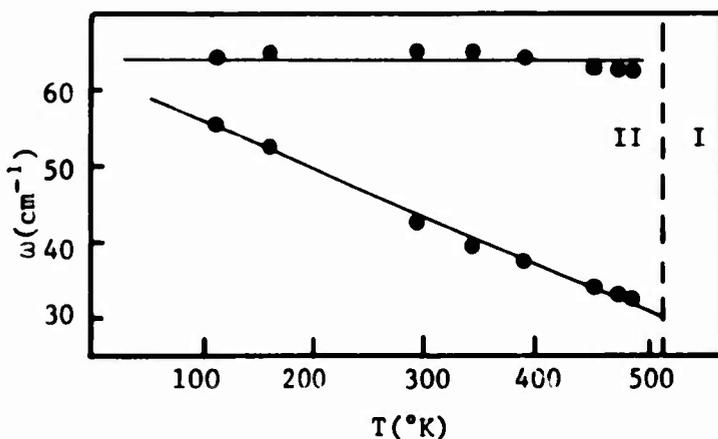
FIGURE 4: Temperature dependence of the Ag symmetry-species  $\text{ClO}_4^-$  vibrational modes. The orthorhombic to cubic phase transition is at  $513^\circ\text{K}$ .  $\omega$ , here, represents the peak position.
