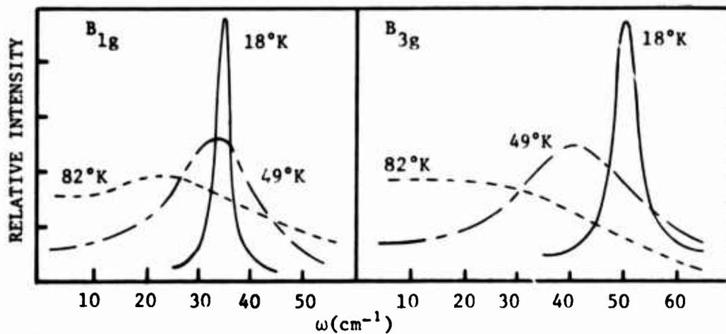
FIGURE 3: Raman spectra of the  $\text{NH}_4^+$  soft modes observed in ammonium perchlorate.
