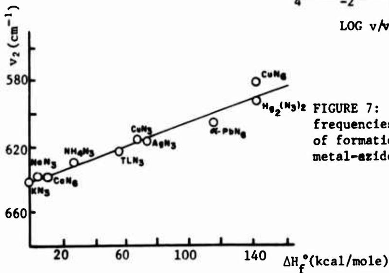
FIGURE 7: Bending mode ( $\nu_2$ ) frequencies versus the heat of formation for a number of metal-azide salts.
