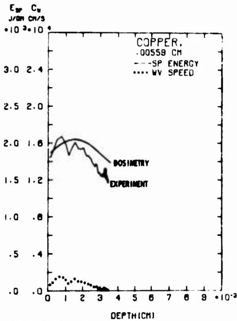
FIGURE 9. Specific Energy ( $E_{sp}$ ) and Wave Speed ( $C_w$ ) versus Depth in Copper at 48 cal/cm<sup>2</sup> Absorbed.
