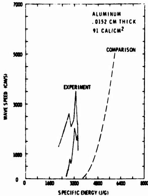
FIGURE 14. Measured Wave Speeds versus Specific Energy Compared with Exploding Wire Data Fit.
