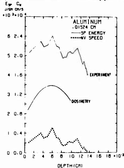
FIGURE 11. Specific Energy ( $E_{sp}$ ) and Wave Speed ( $C_w$ ) versus Depth in Aluminum at 91 cal/cm<sup>2</sup> Absorbed.
