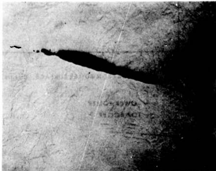
Figure 62. Cracks Extending From Electron Beam Weld Voids.
