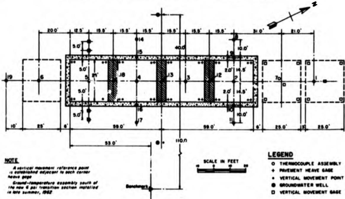
Figure 7. Instrumentation location.
