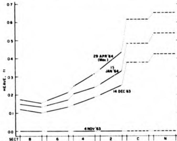
Figure 22. Longitudinal heave profiles, 1963-64.
