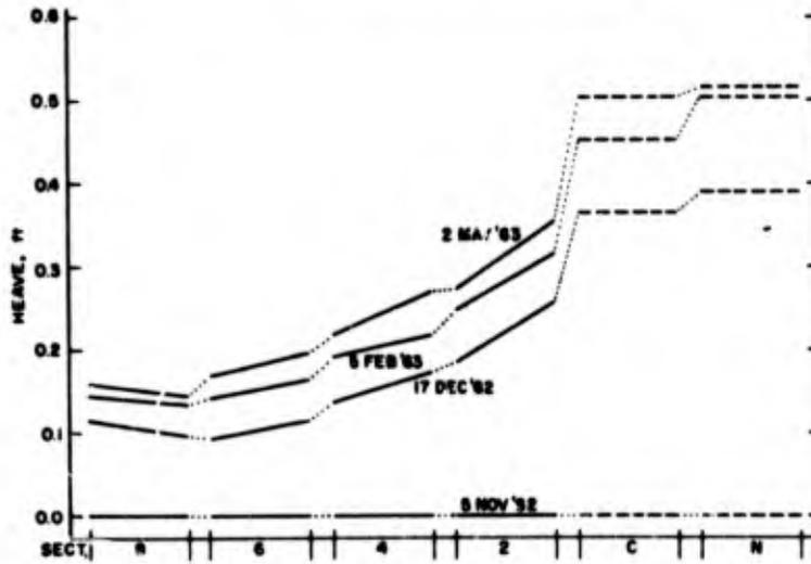
Figure 19. Longitudinal heave profiles, 1962-63.
