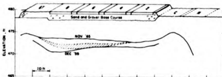
Figure 6. Depth to permafrost along centerline of test area.
