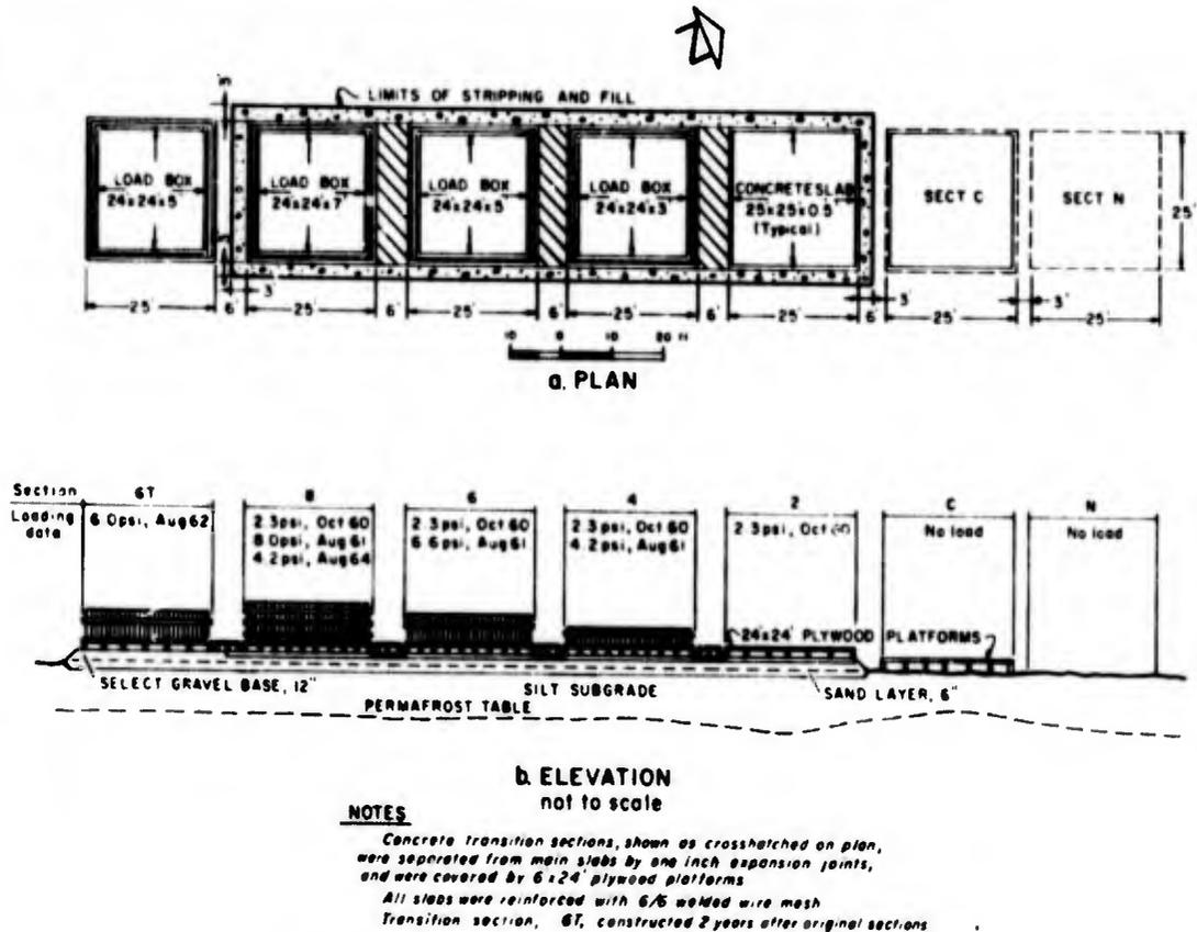
Figure 3. Plan and elevation of test installation.
