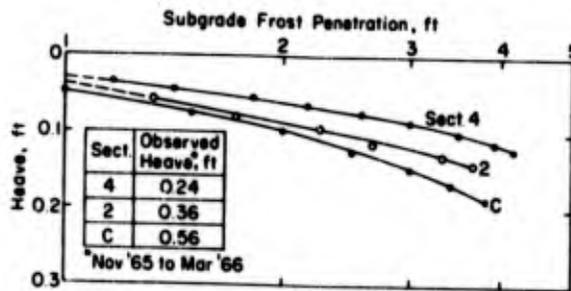
Figure 25. Heaves calculated from November 1965 soil data.
