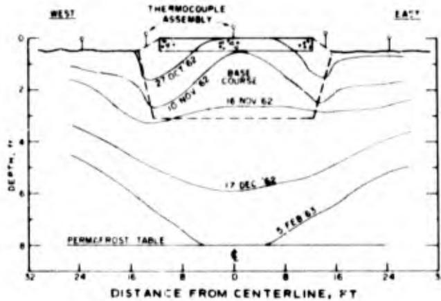
Figure 10. Transverse frost penetration, section 6.
