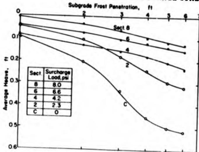
Figure 24. Subgrade frost penetration versus heave and surcharge load.
