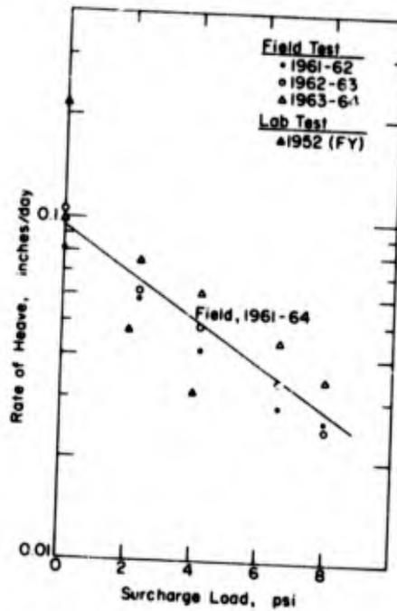
Figure 29. Rate of heave-versus-surcharge load.
