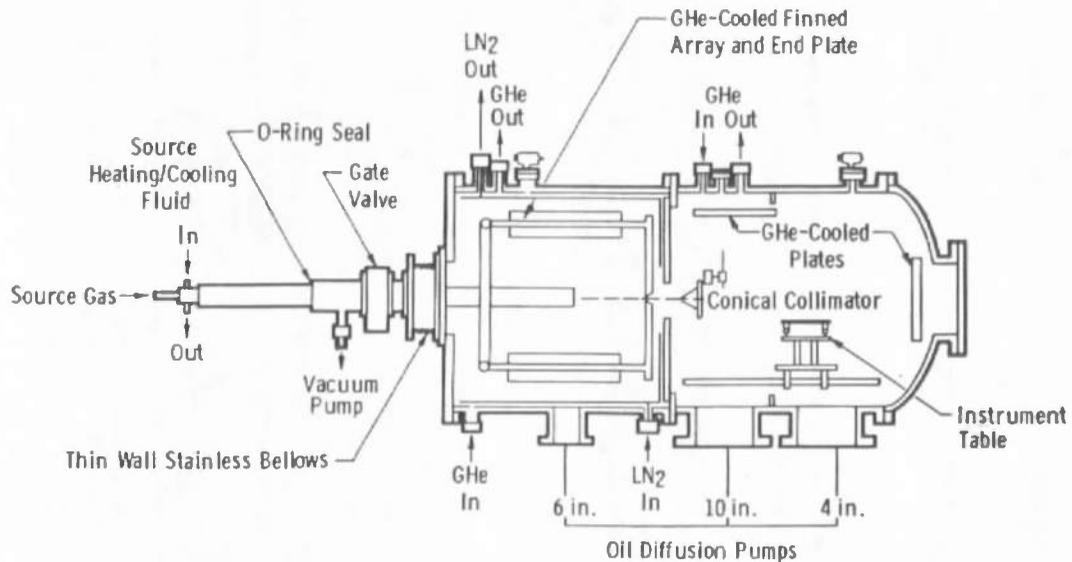
Figure 1. Schematic of AEDC-VKF molecular beam chamber.
