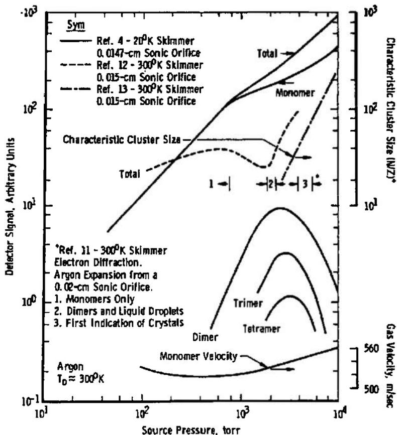
Figure 3. Indicators of condensation in free-jet expansions.
