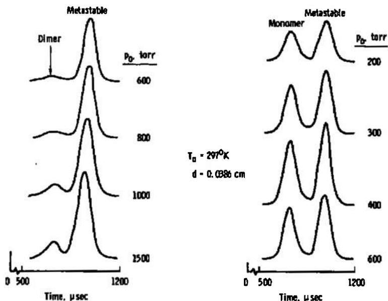
Figure 4. Velocity distribution for an argon beam.
