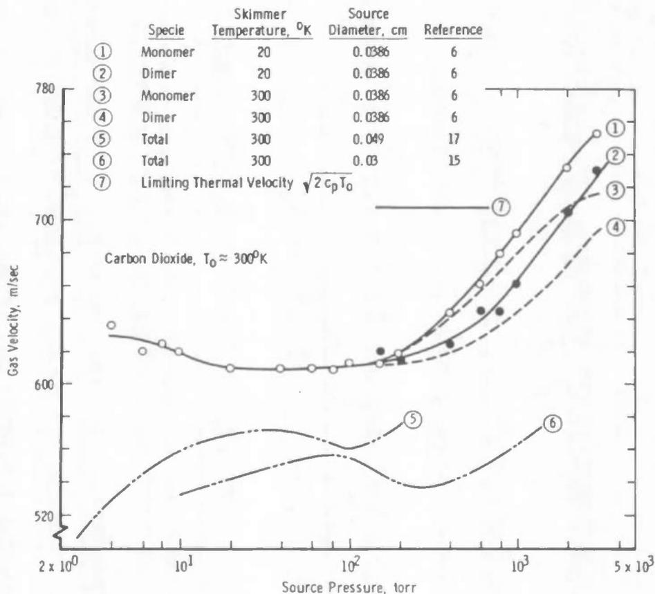
Figure 9. Comparison of carbon dioxide velocity measurements.
