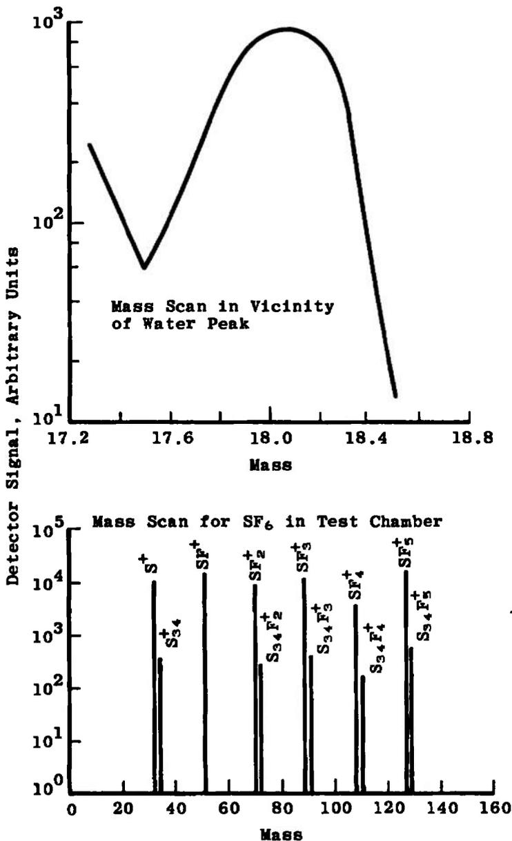
Figure 4. Resolution characteristics of the mass spectrometer.
