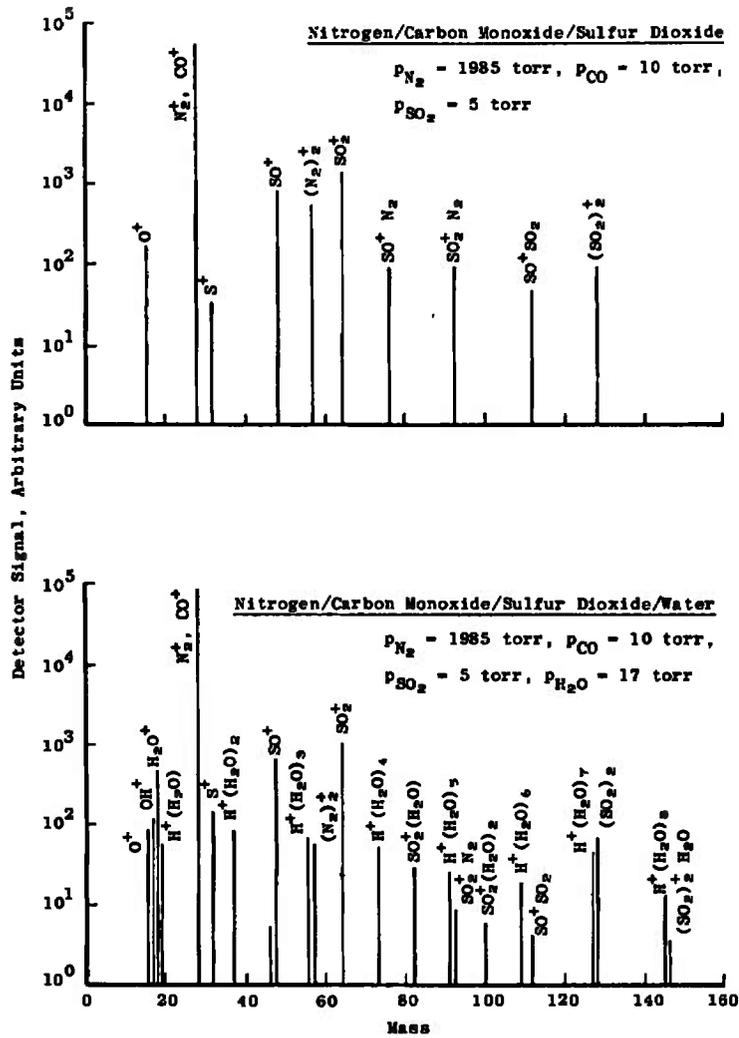
h. Nitrogen/carbon monoxide/sulfur dioxide and nitrogen/carbon monoxide/sulfur dioxide/water
