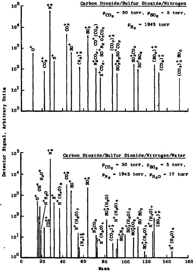
i. Carbon dioxide/sulfur dioxide/nitrogen and carbon dioxide/sulfur dioxide/nitrogen/water
