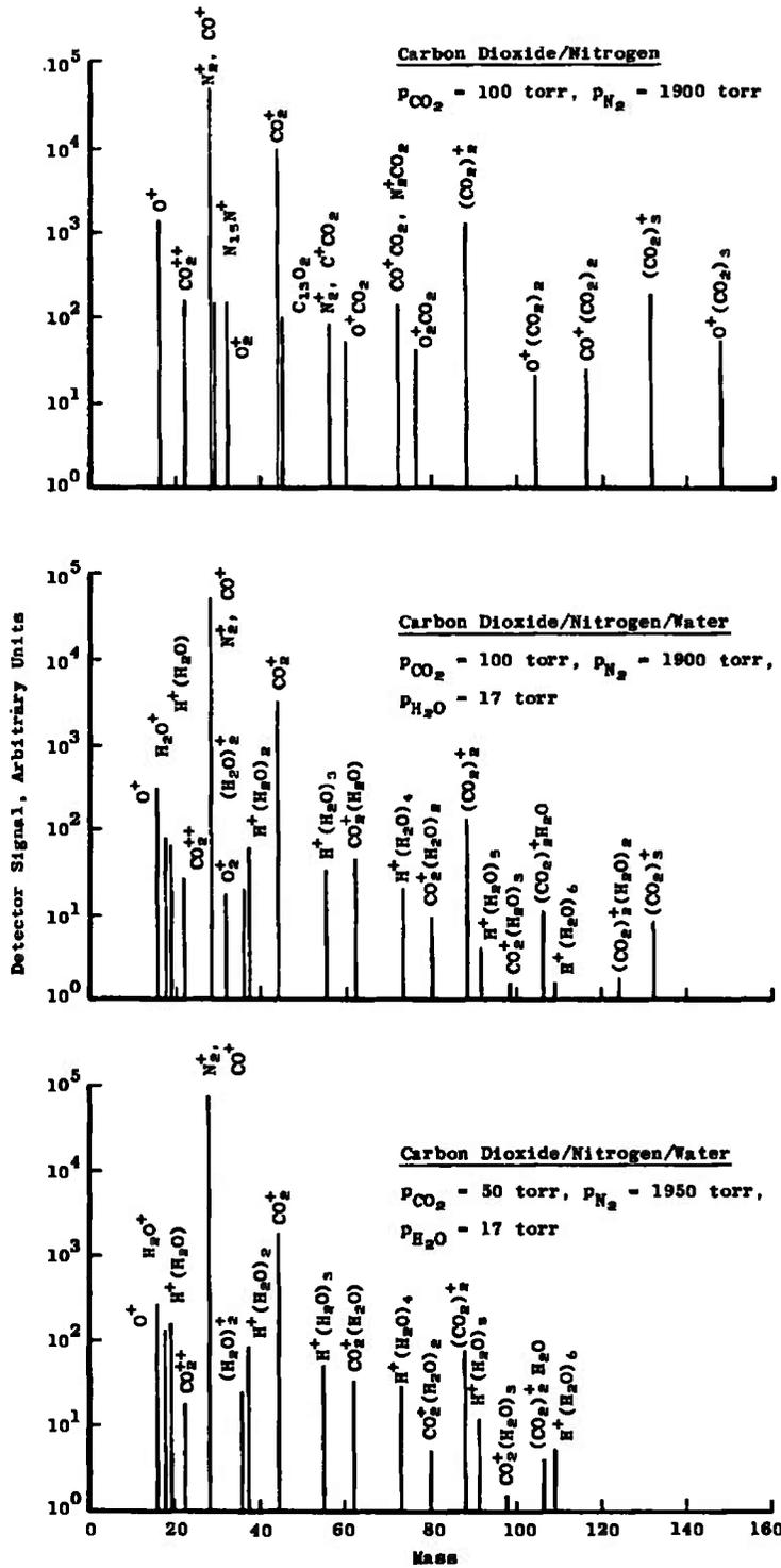
e. Carbon dioxide/nitrogen and carbon dioxide/nitrogen/water
