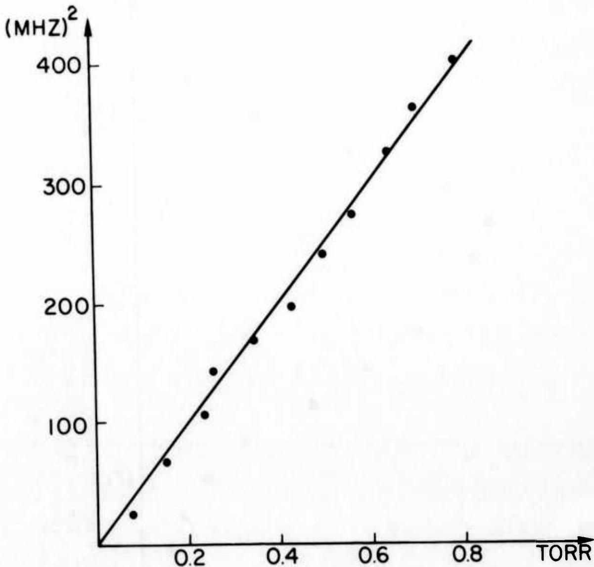
FIG. A-4 - CALIBRATION CURVE ON THE P(7) LINE IN THE (2,1) BAND. THE MEASURED  $\Delta\nu^2 - \Delta\nu'^2$  IS PLOTTED AGAINST THE CO PRESSURE IN THE REACTOR. THE FRACTION OF CO IN (V=1, J=7) IS  $2.7 \times 10^{-6}$ .
