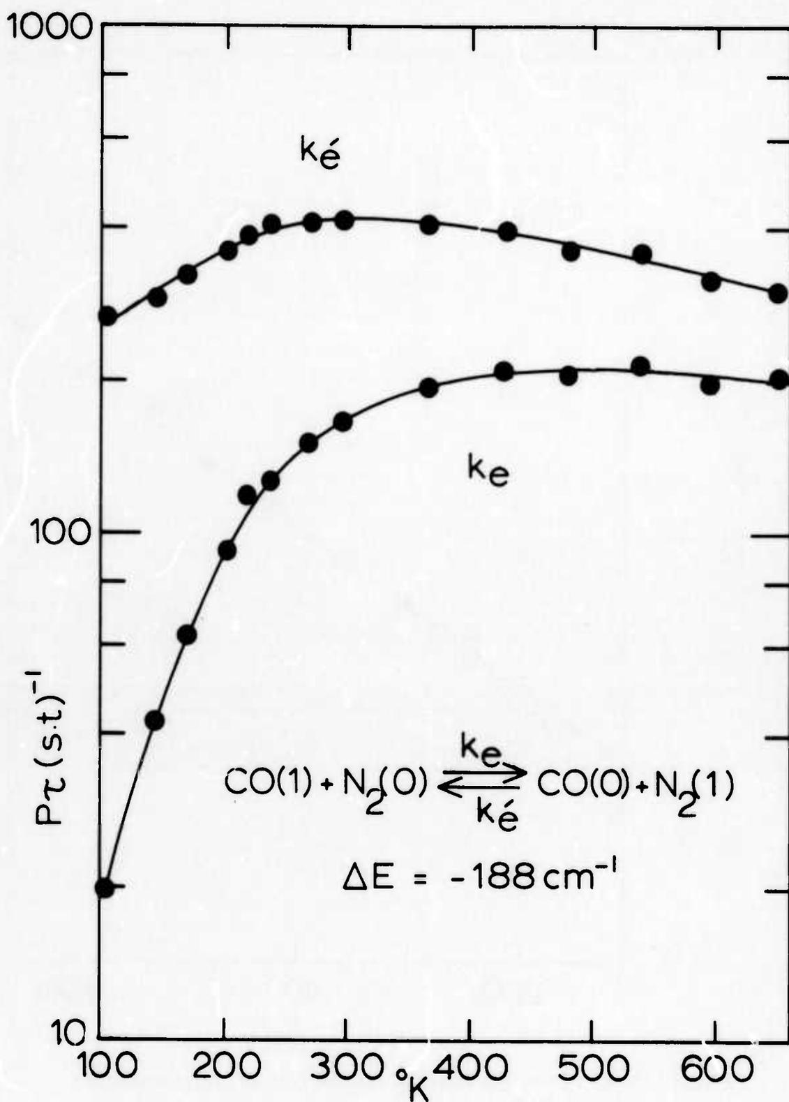
Fig. 4 - Temperature dependence of the relaxation times for V-V energy transfer from CO(v=1) to N<sub>2</sub>.
