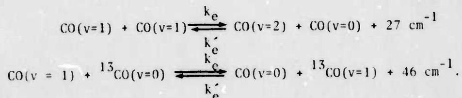
These and future temperature studies are intended to provide rate data of import to electrical and chemical CO lasers, and to test the validity of high temperature V → V data tediously extracted from shock tube measurements.
