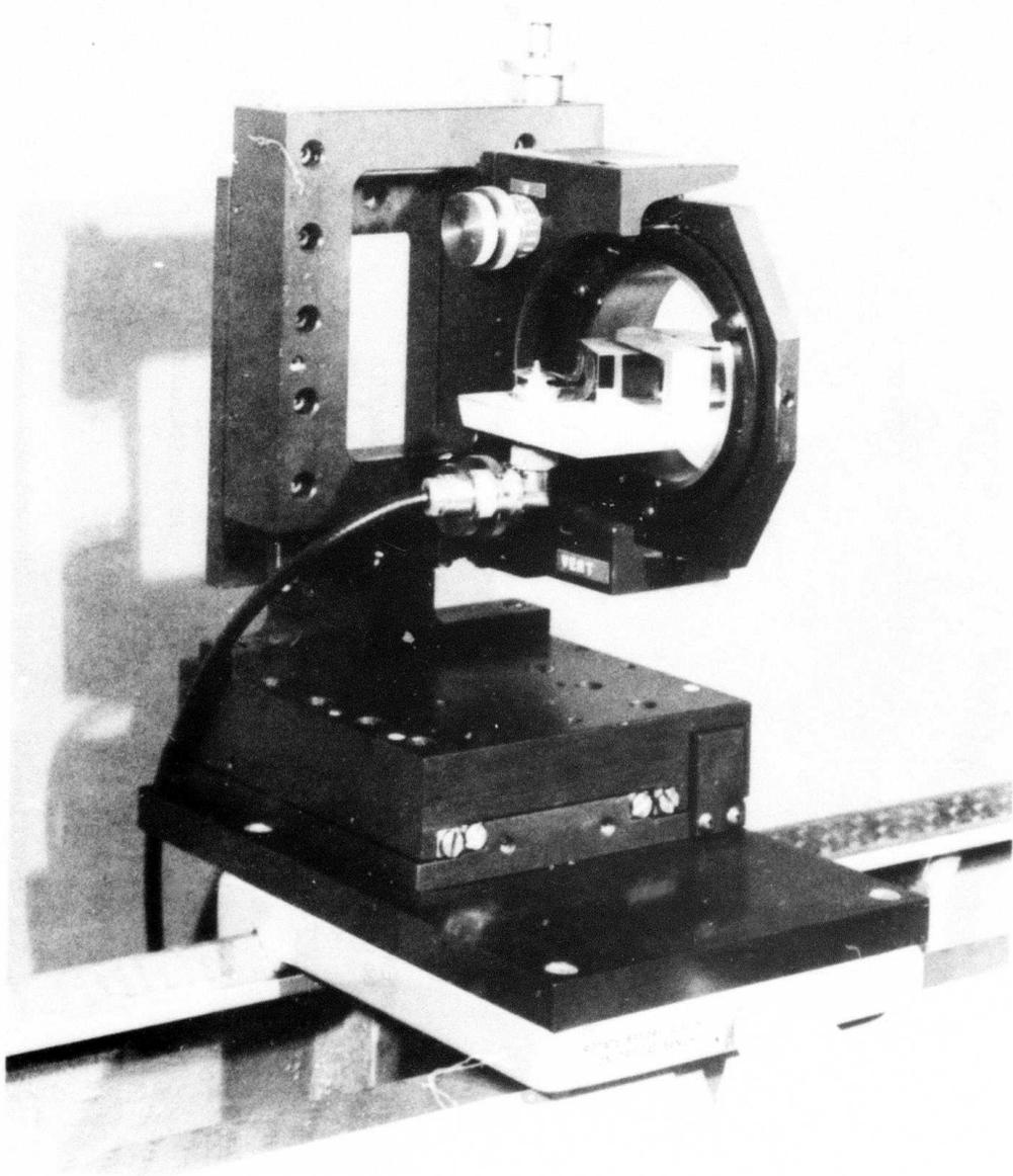
Fig. 8 - Photograph of acousto-optic mode locker.
