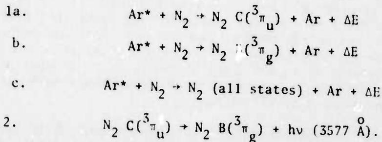
The parameters of interest are the ratio of the rate constant for reaction 1a to that for reaction 1c and the ratio for populating the upper and lower laser levels  $k_{1a}/k_{1b}$ .
