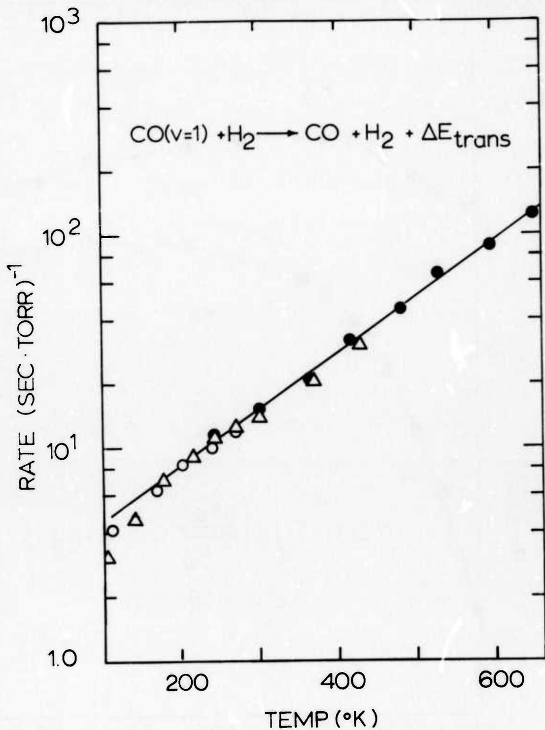
Fig. 3 - Temperature dependence of the rate of relaxation of CO(v=1) by H<sub>2</sub>.
