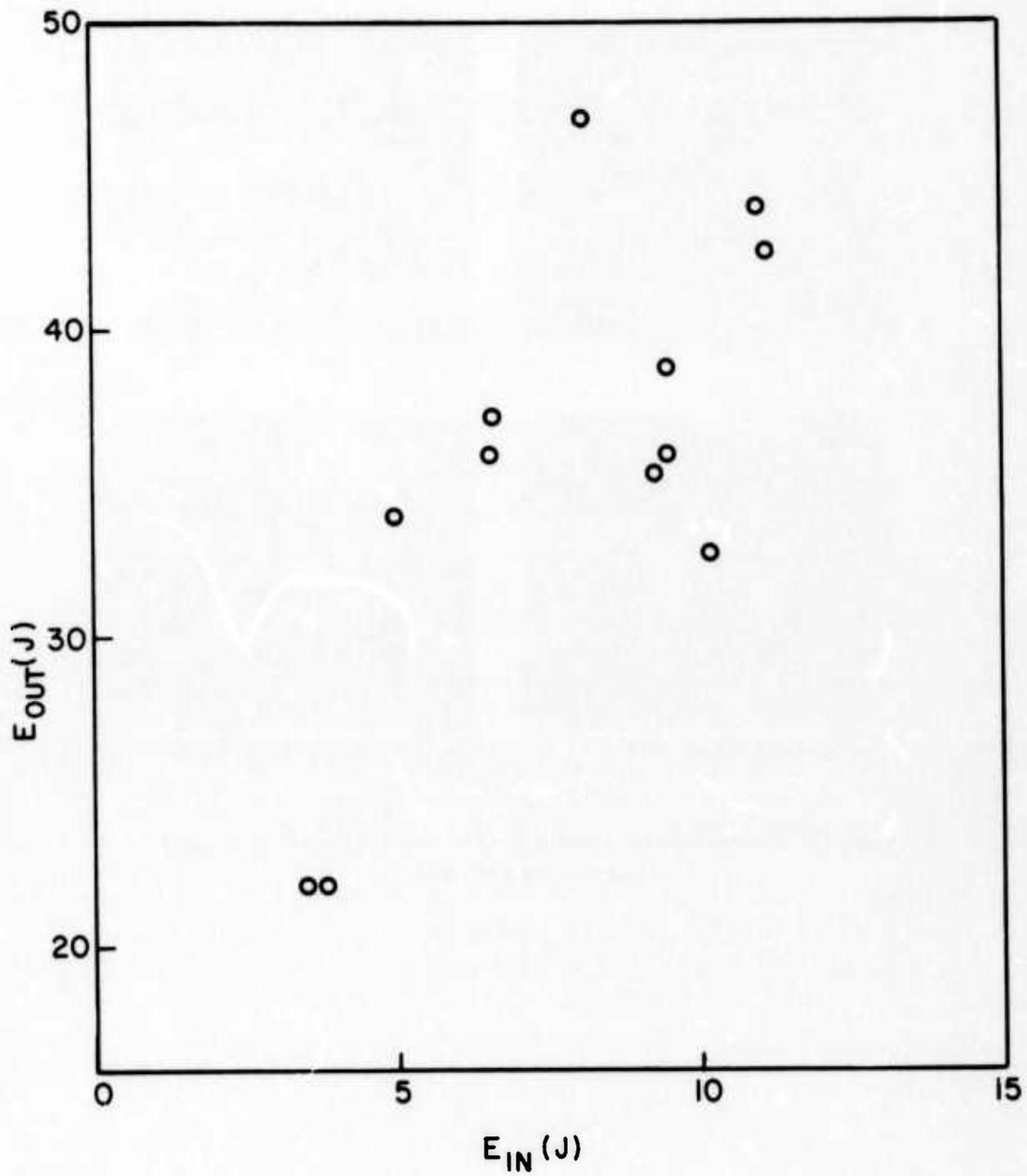
Fig. 16 - Results of pulse amplification with e-beam amplifier .
