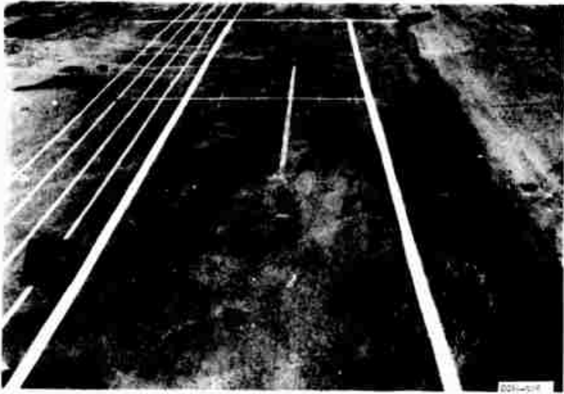
Figure B28. Item 1, lane 2, flexible pavement test section prior to traffic
