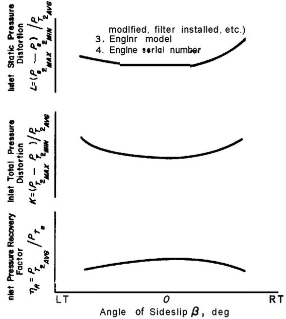
Figure 13-4. Inlet Performance Variation With Angle of Sideslip
