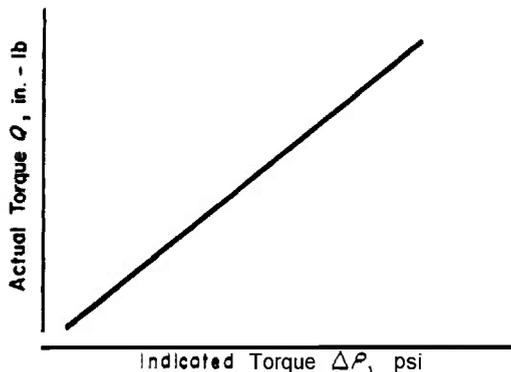
Figure 14-4. Torquemeter Calibration
