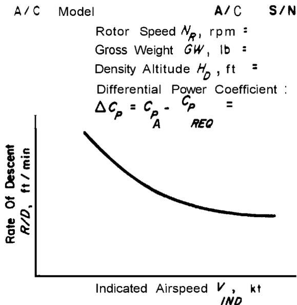
Figure 11-5. Variation in Powered Descent Performance With Differential Power Coefficient
