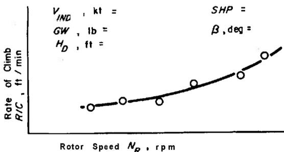
Figure 8-6. Climb Performance Variation With Rotor Speed
