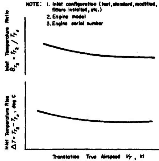
Figure 13-14. Inlet Temperature Rim During Translation
