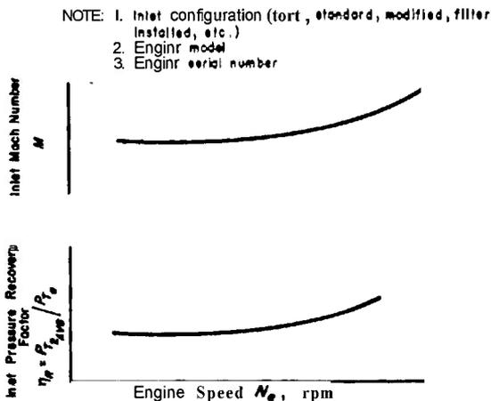
Figure 13-7. Inlet Performance Variation With Engine Speed
