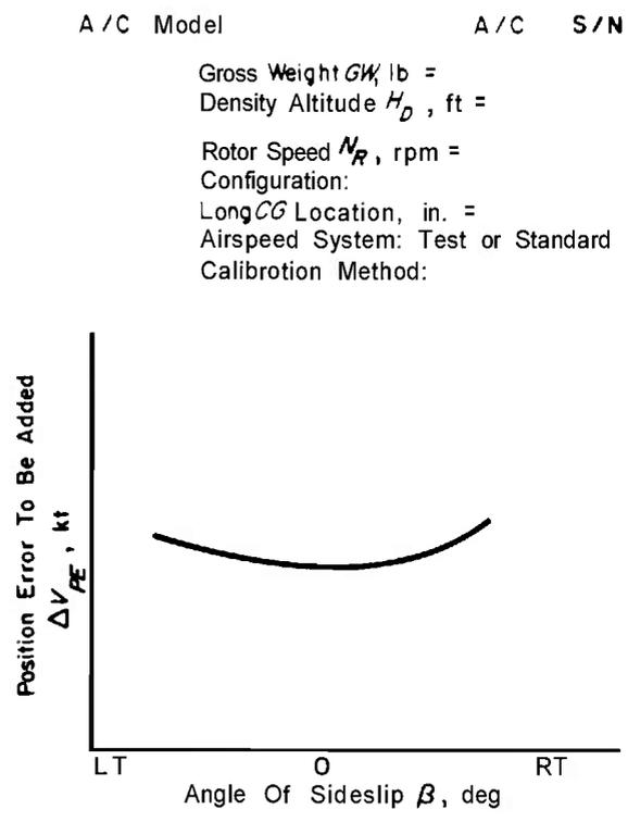
Figure 12-6. Position Error Correction for Angle of Sideslip
