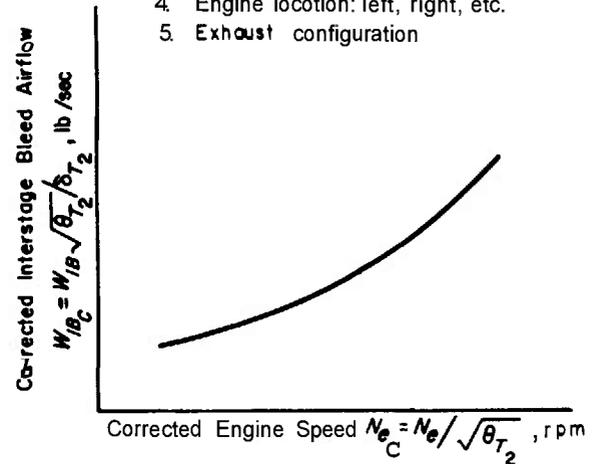
Figure 14-10. Interstage Bleed Airflow and Engine Speed
