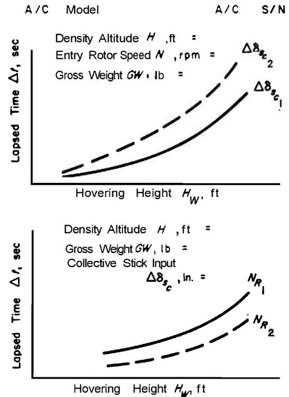
**Figure 10-28. Lapsed Time During Hover Landing**
