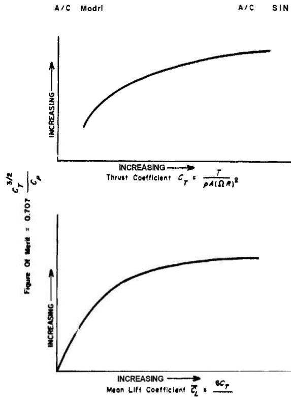
**Figure 5-9. Figure of Merit and Mean Lift Coefficient**
