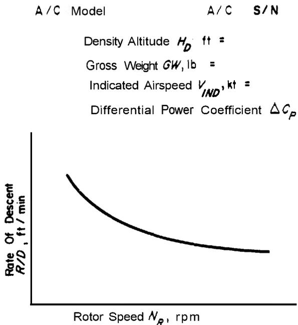
Figure 11-6. Powered Descent Performance Change With Rotor Speed
