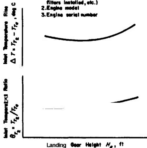
Figure 13-12. Inlet Temperature Variation With Hover Height
