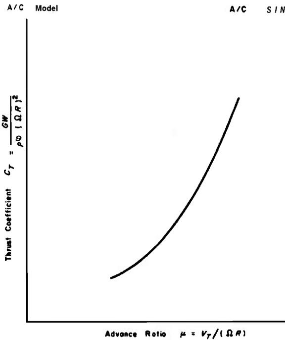
Figure 9-10. Advance Ratio for Minimum Power Required
