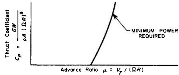
Figure 9-5. Nondimensional Airspeed for Minimum Power Required
