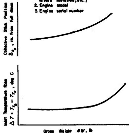
Figure 13-13. Inlet Temperature Variation With Hover Thrust
