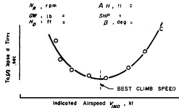
Figure 8-1. Rate of Climb Variation With Airspeed
