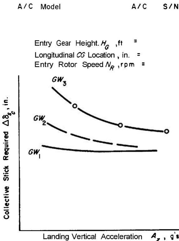
**Figure 70-26. Collective Stick Required During Hover Landing at Various Gross Weights**
