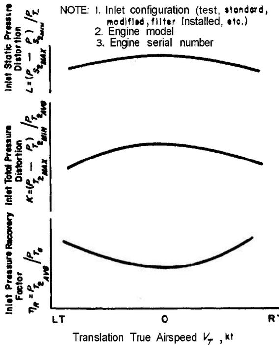
Figure 13-6. Inlet Pressure Characteristics During Translation
