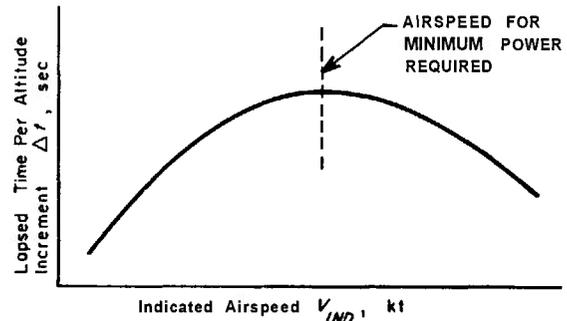
Figure 11-1. Rate of Descent Variation With Airspeed
