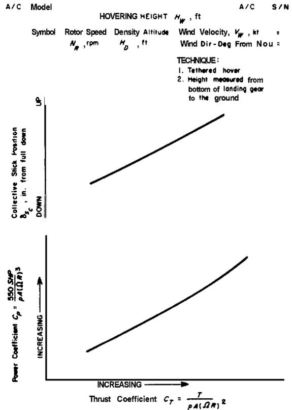
**Figure 5-1. Nondimensional Hovering Performance and Collective Stick Positions**
