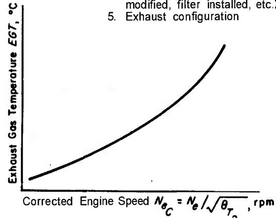
Figure 14-14. Exhaust Gas Temperature and Engine Speed
