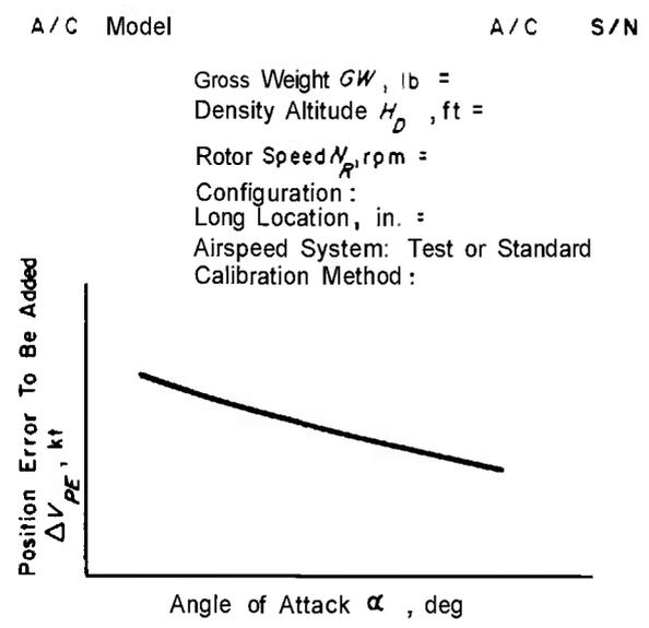
Figure 12-7. Position Error Correction for Angle of Attack
