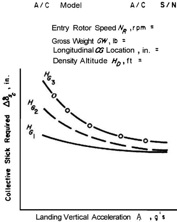
**Figure 10-25. Collective Stick Required During Hover Landing at Various Entry Gear Heights**
