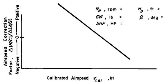
Figure 8-5. Rate of Climb Correction Factor for Airspeed
