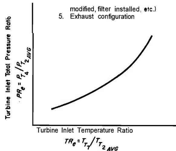
Figure 14-11. Turbine Inlet Pressure and Temperature Characteristics
