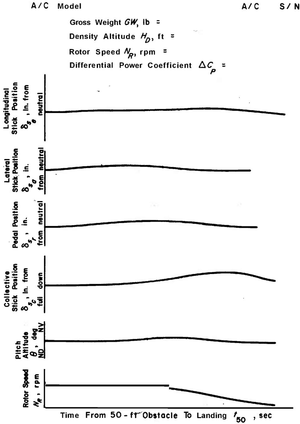
Figure 11- 12. Control Positions During Maximum Performance Landing
