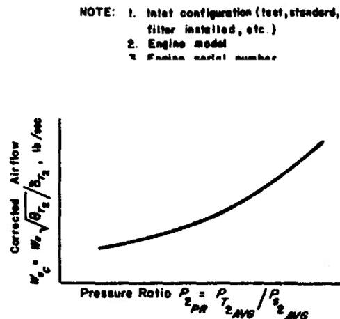
Figure 13-9. Inlet Airflow and Pressure Characteristics
