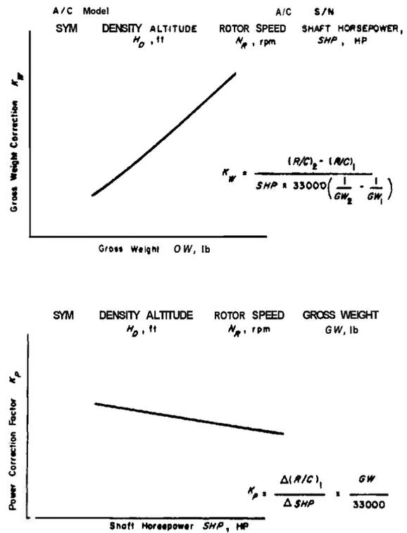
Figure 8-73. Gross Weight and Power Correction Factors
