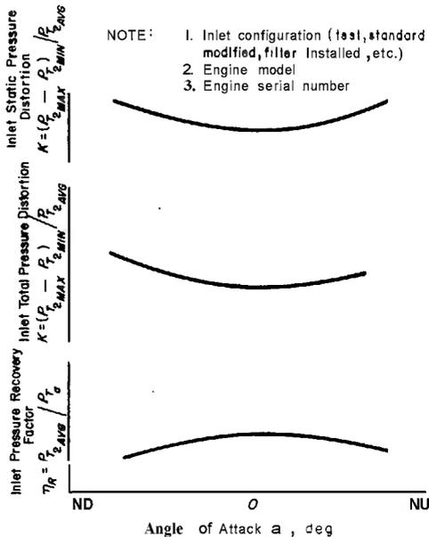
Figure 13-3. Inlet Performance Variation With Angle of Attack
