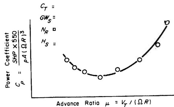
Figure 9-3. Nondimensional Level Flight Performance
