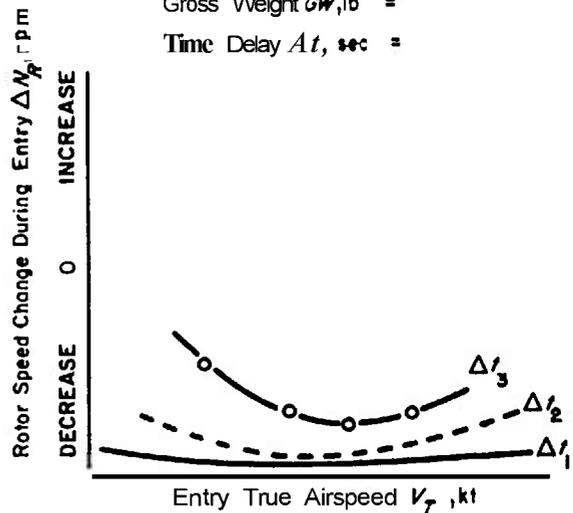
Figure 10-16. Rotor Speed Change During Autorotation Entry
