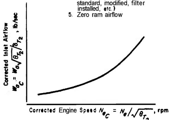
Figure 14-6. Inlet Airflow and Engine Speed
