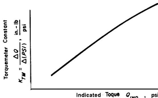
Figure 14-1. Torquemeter Constant as a Function of Power Setting
