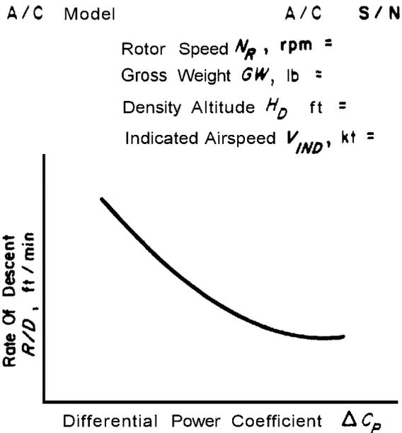
Figure 11-4. Variation in Powered Descent Performance With Airspeed
