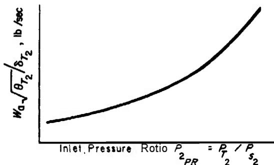
Figure 14-5. Airflow Variation With Inlet Pressure Ratio
