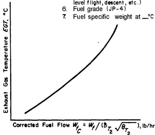
**Figure 14-16. Exhaust Temperature Variation With Fuel Flow**
