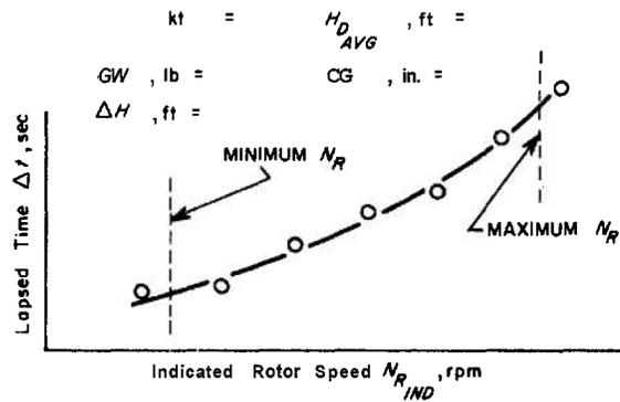
**Figure 10-2. Autorotational Descent Performance Variation With Rotor Speed**
