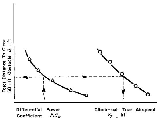
**Figure 7-11. Airspeed and Distance for Maximum Takeoff Performance**
