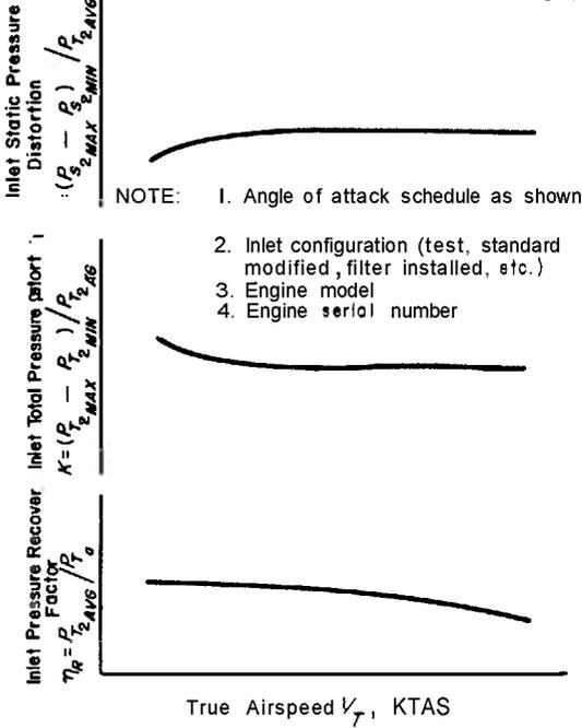
Figure 13-2. Inlet Performance Variation With Airspeed
