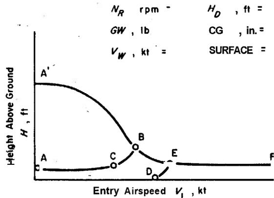
Figure 10-8. Recommended Altitude for Safe Landing Following an Engine Failure
