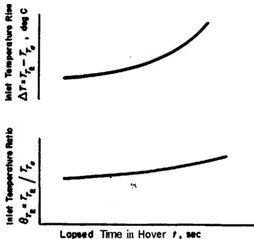
Figure 13-11. Inlet Temperature Variation During Hover
