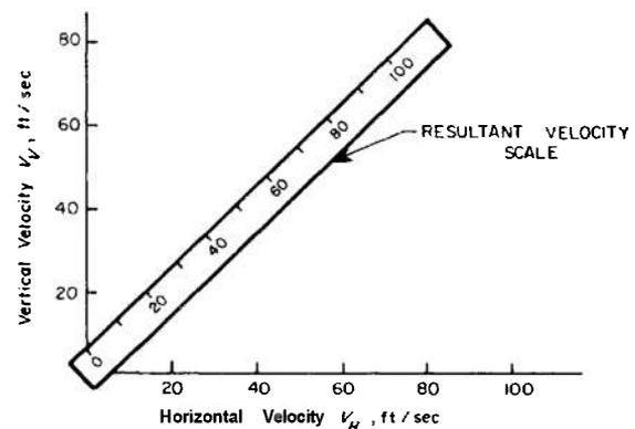
Figure 7-8. Device for Graphical Determination of True Airspeed
