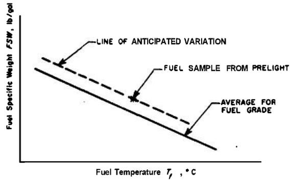
Figure 14-2. Fuel Specific Weight Variation With Temperature
