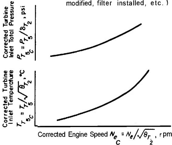
Figure 14-12. Pressure and Temperature Variation With Engine Speed
