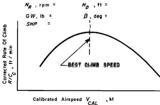
Figure 8-4. Sawtooth Corrected Climb Performance
