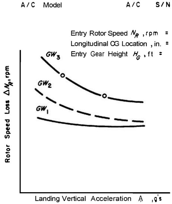
**Figure 10-27. Rotor Speed Required During Hover Landing**
