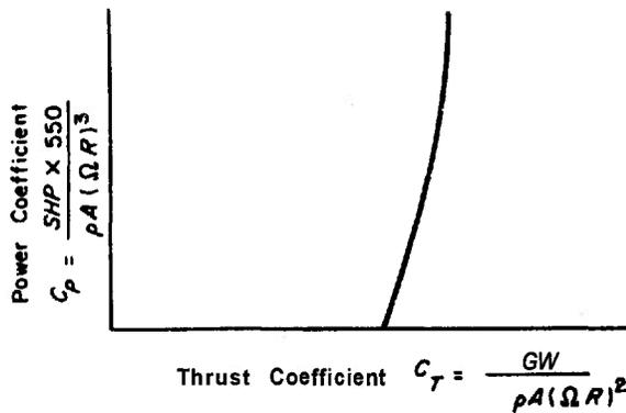
**Figure 9-6. Nondimensional Power Required at Best Endurance Airspeed**
