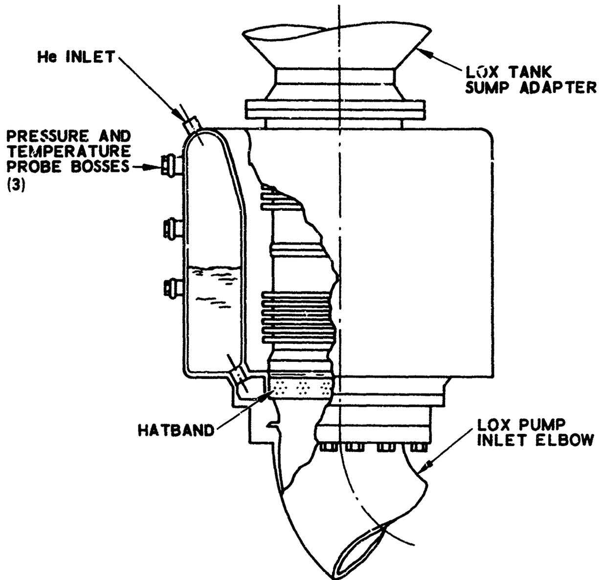
Fig. 17. ITOS-E Lox Accumulator
